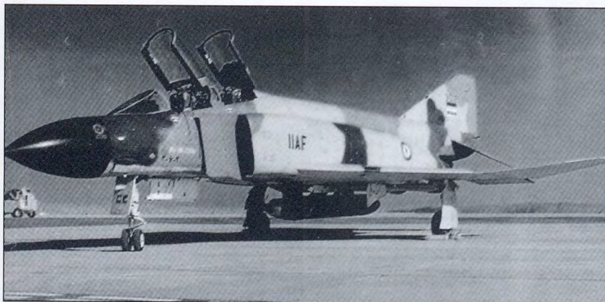
F-4D 67-14870 was the second Phantom II supplied to Iran, and the jet is seen here shortly after its delivery to the IIAF. Note the SUU-23/A gun pod mounted on the aircraft's centreline. This weapon was standard equipment for the F-4D during the Iran-Iraq War (US DoD)
