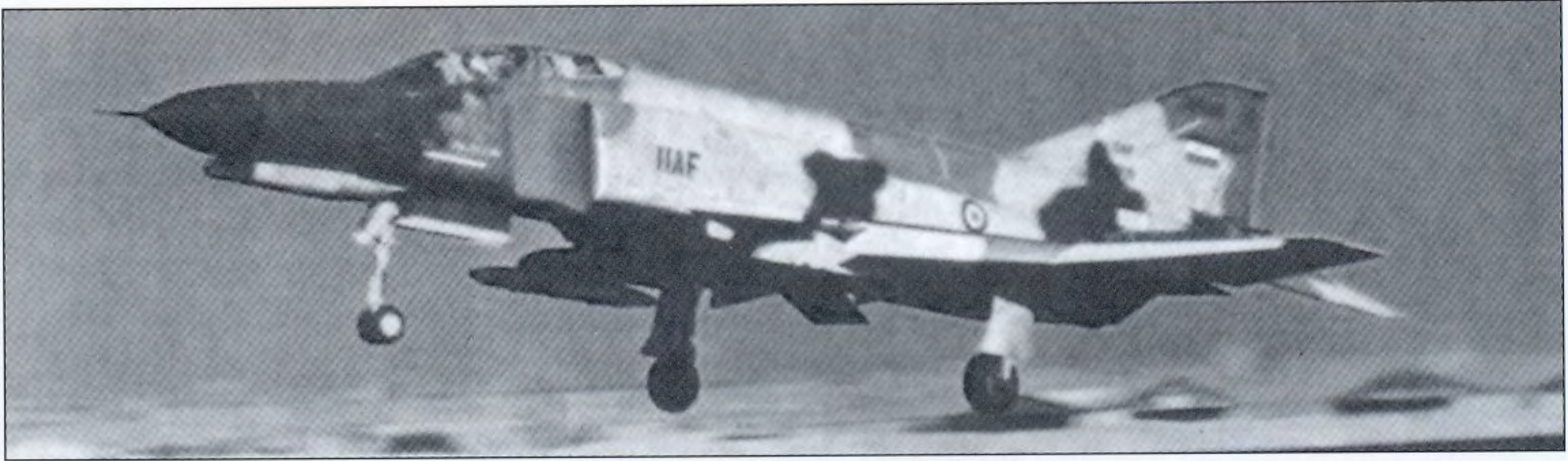
An ALQ-87(V)3 ECM pod-equipped Block 51-56 F-4E takes off from Mehrabad air base in the late 1970s. The aerals on the underside of the pod have been touched out on the photo by the IRIAF's official censor (authors' collection)
