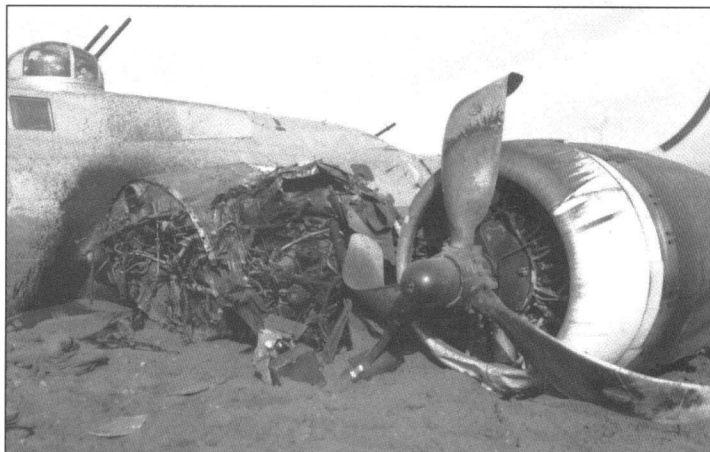
This unidentified B-17G from the 483rd BG had its No 2 engine ripped off its mounts in a crash-landing that almost certainly resulted in the bomber being salvaged. The date and location of this incident also remain unrecorded (USAAF)
