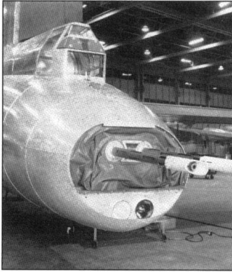
The tail-gun station on a B-17E photographed on the Boeing production line on 1 October 1941. This view shows the early style ring-and-bead sight mounted outside the window, which was replaced on Fortresses two years later by an internal reflector sight. In the Pacific, Japanese fighter pilots who had grown accustomed to attacking early Fortresses from the rear received an unpleasant shock when they came up against the rear gun installation fitted to B-17Es for the first time. Prior to the arrival of tail guns, Fortress pilots had learned to compensate for this weakness by jinking their aircraft back and forth when being attacked from the rear, alternatively giving the left and right waist gunners a shot at the approaching fighters ( Boeing )
