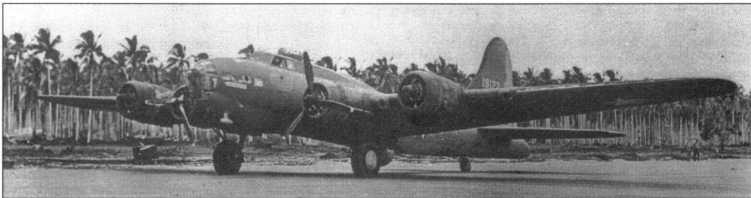
B-17E 41-9122 Eager Beavers of the 72nd BS/11th BG taxis in on two outboard engines at Henderson Field in an effort to save precious fuel, which was always in short supply in the Solomons. This Fortress later transferred to the Thirteenth Air Force (USAF)
