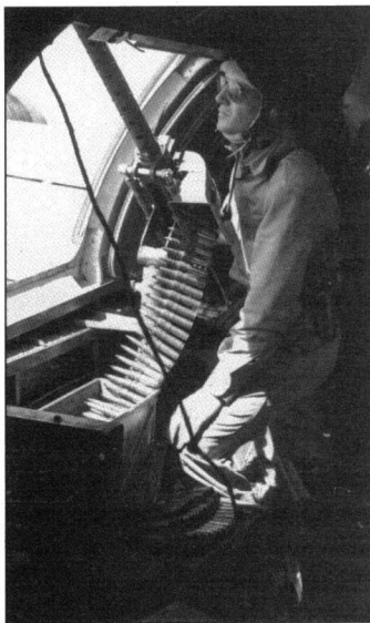
A B-17E waist gunner maintains a watchful eye during a photo-reconnaissance mission over New Guinea. The gun mount allowed him to swivel his 0.50-cal machine gun both inside and outside the window opening (USAF)
