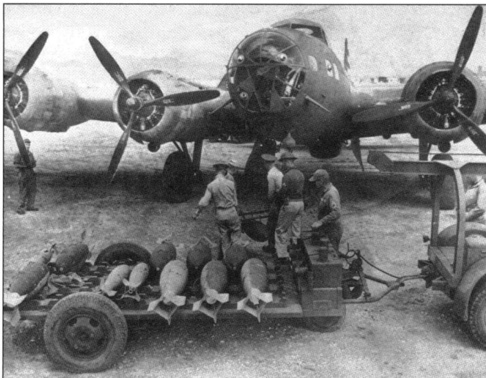
Armourers hastily load 100- and 500-lb bombs into the bomb-bay of a B-17D either in the Philippines or the Dutch East Indies during the first weeks of the war in the Pacific (USAF)
