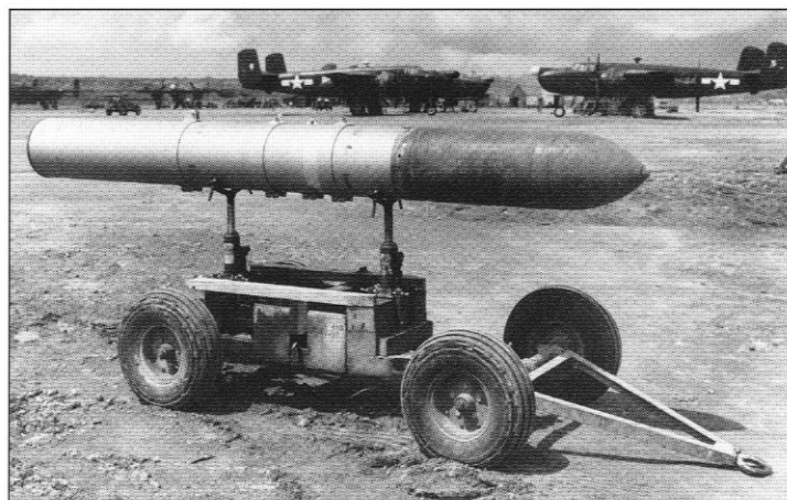
A modified truck hoist is used to swing the rocket onto its special wheeled trailer (National Archives)
