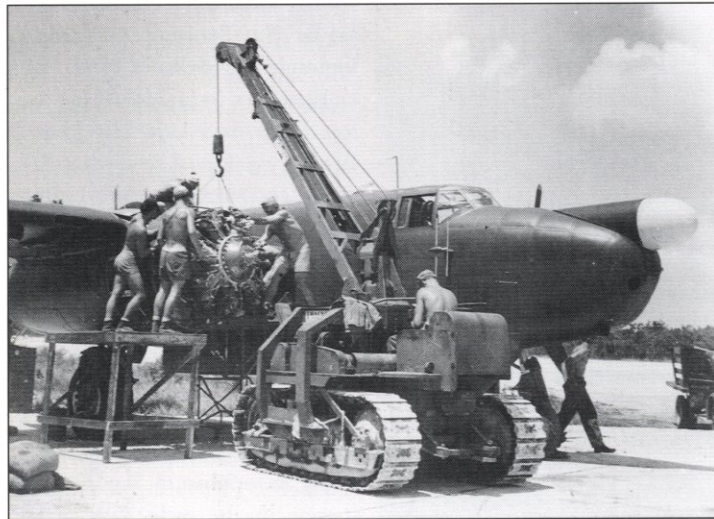
For the final period of the war VMB-612's PBJs wore the overall sea blue colour scheme introduced for patrol bombers in 1944. In this view, a crane assists the groundcrew as they change an engine at Boca Chica prior to the unit heading overseas ( via Thomas Honeycutt )
