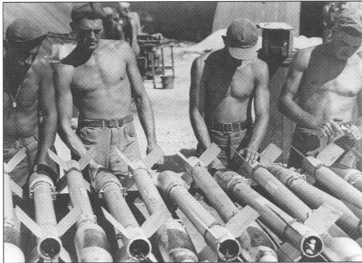
When VMB-612's PBJs dropped most of their machine guns to save weight on long over-water flights, the squadron's favoured armament became the high velocity aircraft rocket (HVAR). Each PBJ carried eight, and armorers are seen here checking rockets with shaped-charge heads (via Thomas Honeycutt)
