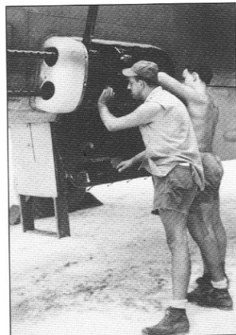
VMB-433 armourers inspect the breeches of the port twin 0.50-cal package guns fitted to a squadron PBJ-1D. Operated by the pilot, the four 'cheek' guns gave a useful spread of fire during strafing runs. Good maintenance access was provided via a single downward-hinged panel (Henry Sory via Alan Carey)
