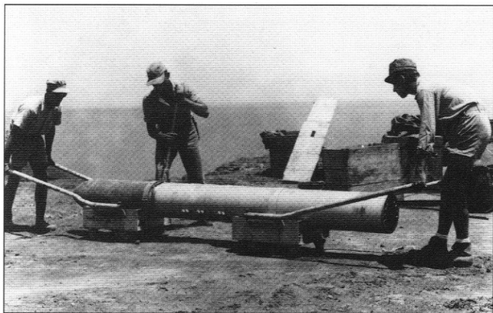
After uncrating, the rocket's motor section (light colour) was attached to the warhead (darker colour) using a spanner wrench (National Archives)
