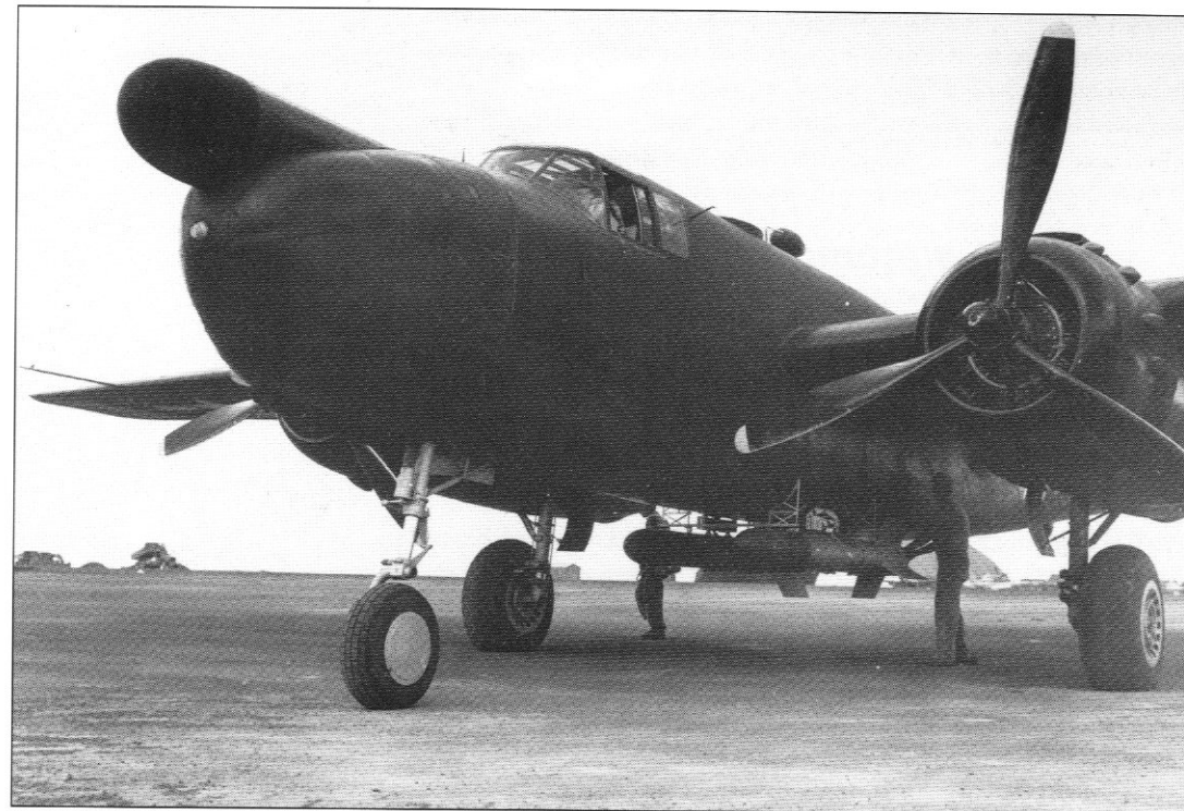
Another VMB-612 PBJ-1J with 'Tiny Tim' rockets in place. Like most Mitchells assigned to the unit, this aircraft has had its dorsal turret and all other guns, except one in the tail, removed ( National Archives )
