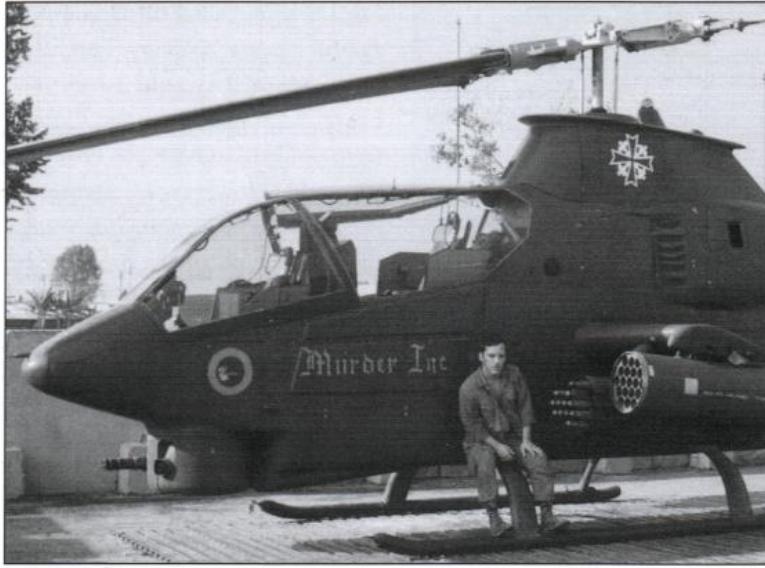
Like AH-1G 67-15649, featured in the previous chapter, 'Blue Max' Cobra 67-15674 Murder Inc had the wiring panels for 20 mm cannon, but is shown here configured as a 'Heavy Hog', with two XM-159 19-shot rocket pods per stub wing. Photographed in early 1971, this veteran Cobra soldiered on with the 2/20th ARA until it was destroyed on 11 May 1972 defending An Loc (Jim Moran)
