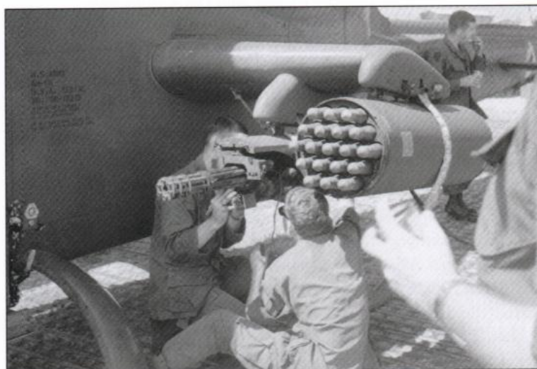
AH-1G 66-15275 is seen undergoing routine maintenance on its left 7.62 mm Minigun. Again, the fairing that covered the weapon when in flight has been removed. Note the fully loaded XM-200 pod on the outer stub pylon (Jessie Robertson)
