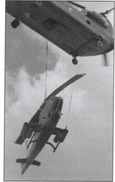
AH-1G 66-15272 of the 'Playboy' platoon was sling-loaded under a CH-47 after being downed by NVA 0.30-cal machine gun fire on 16 November 1967. The helicopter, flown by Capt Rubin, was escorting 118th AHC 'slicks' when it was hit five times, one bullet piercing a wiring bundle which then illuminated a fire warning light on the pilot's control panel. Unsure of whether or not the engine was on fire, Rubin set the aircraft down as soon as possible. The sling-loading of battle-damaged AH-1Gs beneath Chinooks became routine in Vietnam as more Cobras went into combat (Jessie Robertson)
