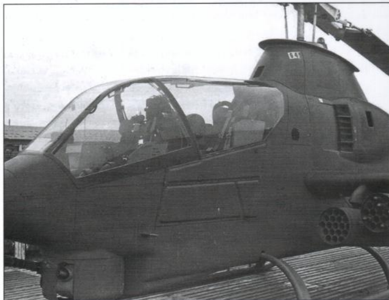
This 'Dragons' AH-1G (67-15649) received the 20 mm gun upgrade, but it is seen here without the fuselage ammunition containers or the cannon. Instead, it is carrying two XM-159 19-shot rocket pods. The helicopter was also retro-fitted with an Environmental Control Unit (air conditioning) in the field (Barry Martens)
