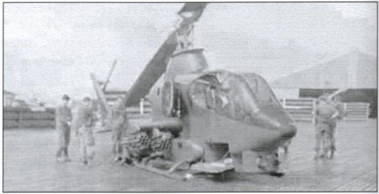
This D/101st Aviation Battalion AH-1, armed with a 20 mm cannon, three seven-shot rocket pods and the nose turret, attempted to take off from Khe Sanh overloaded with ammunition and fuel. Due to the density altitude and the aircraft's gross weight, the helicopter's engine did not have enough power to lift the AH-1 and it settled hard, with the main rotor striking the runway (Barry Martens)
