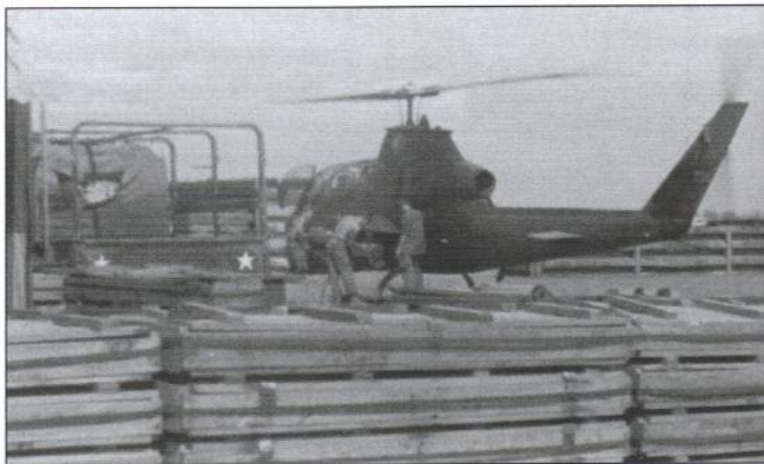
Rotors still turning, a 'Dragons' AH-1 is 'hot' rearmed at Khe Sanh with 10-lb FFAR rockets, offloaded from the back of a 3/4-ton truck, in February 1971 (Barry Martens)
