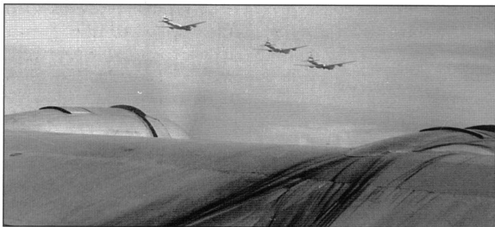
As this B-29 formation heads for North Korea, an oil leak from the number two engine splatters black liquid on the left wing surface. The aircraft, from the 19th BS/93rd BG, is 44-61751, a B-29-45-BN Superfortress (c/n 11218) built at Boeing's Renton factory. The crew called the ill-fated Superfortress Lubricating Lady (Frank Farrell)
