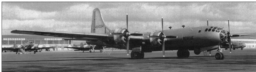
SB-29 Superfortress 44-84084 sits on the ramp between missions. This search and rescue version of the bomber is seen without the lifeboat it was capable of carrying beneath the fuselage. The SB-29 flew vital rescue missions throughout the fighting from 1950 to 1953. (US Air Force)
