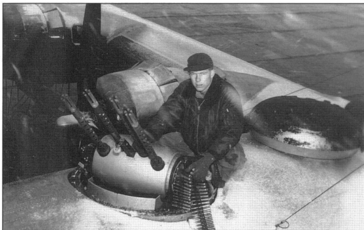
An unidentified B-29 gunner loads a belt of 0.50-cal ammunition into the magazine of his top turret. Note the mount's cover resting on the fuselage behind him (Roland T Speckman)
