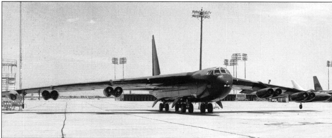
B-52D-75-BO 56-0603 was another early Big Belly aircraft. The way in which the wingtip outriggers remained clear of the ground when the aircraft was lightly loaded is clearly evident in this view. This aircraft was one of those sent to MASDC in the first big batch of D-model retirements between August and December 1978 (Author's collection)
