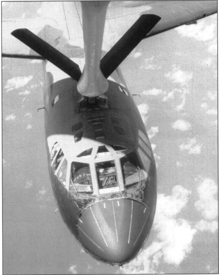
The 'boomer's eye view' of a B-52D, seen during a refuelling contact with a KC-135 tanker. Compared with the previous views of B-52Fs refuelling, this aircraft has new strips running fore and aft on the upper radome (Robert F Dorr)
