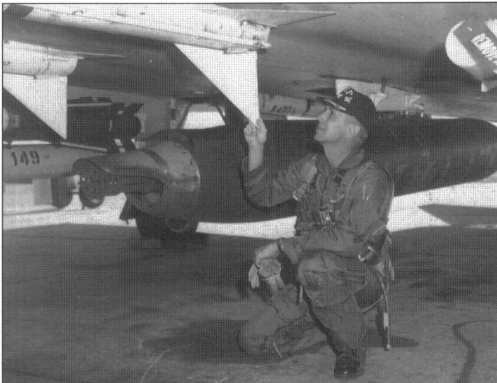
Col D O Williams conducts a pre-flight check of his F-4D at Ubon RTAB in November 1967. The fighter has been load with four AIM-7s, four AIM-4Ds, an SUU-23/A gun and two AN/ALQ-87 ECM jamming pods (via Brig Gen D O Williams)
