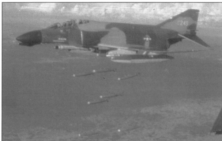
'Raz' Raspberry's F-4D MiG killer 66-0249 remained in South-East Asia until the very end of the Vietnam War, the jet flying its last mission from Ubon on 4 August 1974. Photographed here on a bombing mission over Cambodia in the summer of 1973, the Phantom II carries an AN/ALQ-101 noise/deception jammer. Assigned to the 13th TFS/432nd TRW, its unit markings are confined to a blue fin cap (Col Ron Thurlow)
