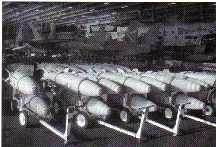
Assembled and ready for loading, 1000-lb GBU-35(V)1/B JDAM crowd the hangar bay of CV-64 on the eve of OIF. All of these weapons would be carefully wheeled onto one of the ship's four elevators and then taken up to the flight deck en masse. Once 'up on the roof', the ordnance would be collected by teams of armourers from the various Hornet and Tomcat squadrons, who would take the bombs away for loading onto their jets (US Navy)
