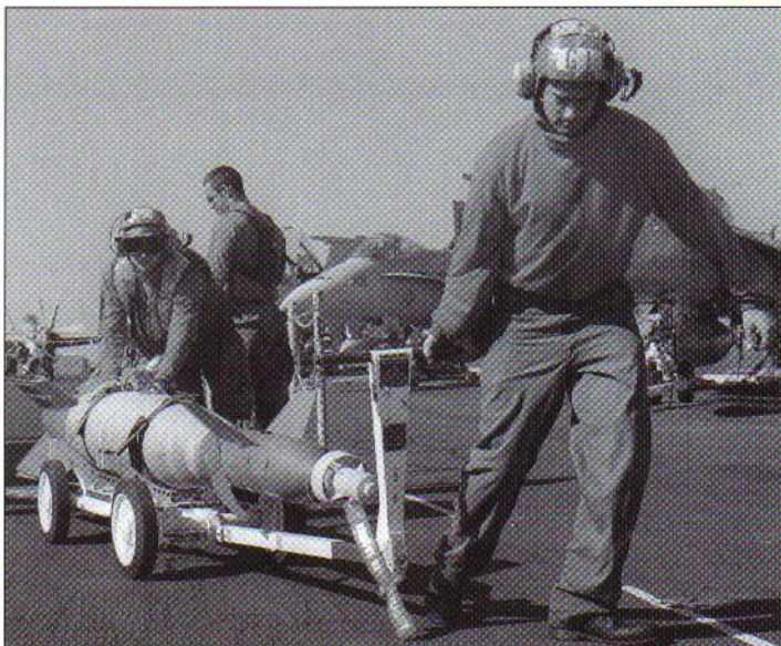
'Ordies' from VFA-94 wheel an Aero-12C weapons skid, laden down with a 2000-lb GBU-10 Paveway II LGB, along the flight deck of CVN-70 in January 1999 (VFA-94)
