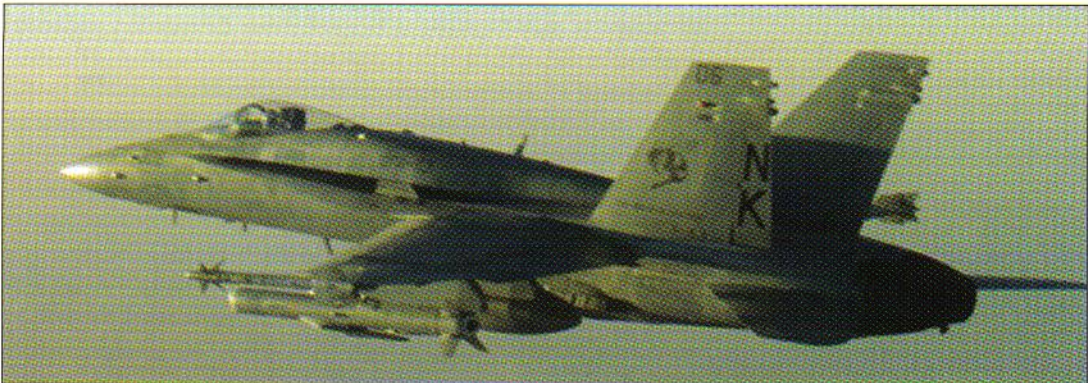
This rare inflight shot of VFA-113’s ‘Sting 306’ (Lot XIV F/A-18C BuNo 164634) was taken on the afternoon of 22 March 2003 as Lt Cdr Paul Olin and his wingman headed for northern Baghdad on CVW-14’s sole AGM-84 SLAM-ER mission of OIF. The weapon, clearly visible on the outer port wing pylon of Olin’s jet, was successfully guided into a large building (Lt Cdr Paul Olin)
