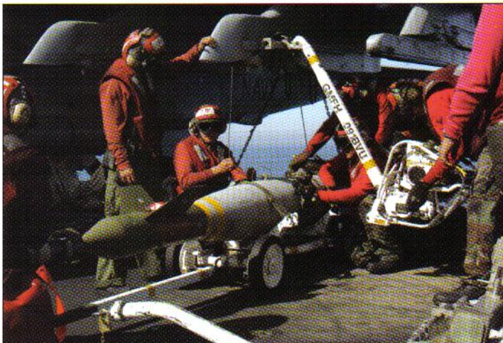
'Talon 202' (BuNo 165783) has a GBU-16 loaded onto station three on 3 April 2003. VFA-115's ordnance team are using a fuel-powered Single Hoist Ordnance Loading System to lift the 2000-lb bomb from its Aero-12C skid up to the SUU-79/A pylon (US Navy)
