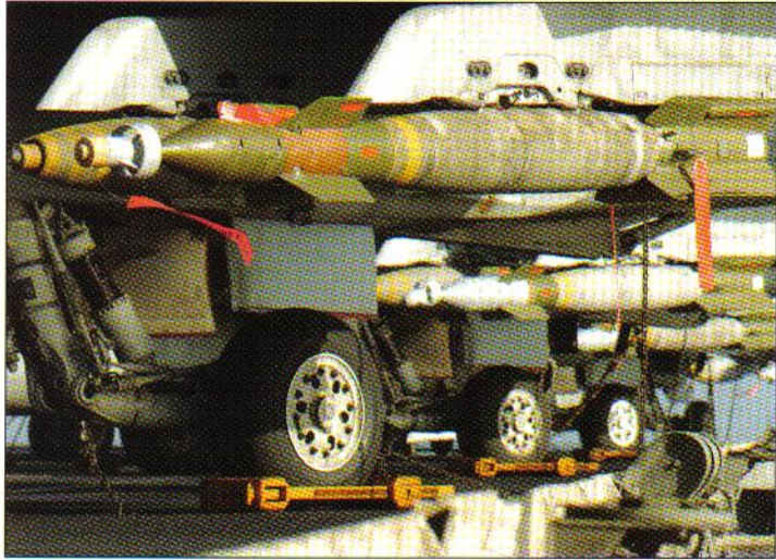
Three F/A-18Cs from VFA-195 and a solitary yellow-legged VFA-192 machine sit over bow cat on one between missions, these aircraft boasting similar war loads. All four have 500-lb GBU-12 LGBs on their outer pylons, with the first three also carrying 500-lb Mk 82 ‘slicks’ (fitted with M904E4 fuses) on the inner pylons. The jet furthest from the camera appears to have a 1000-lb GBU-35(V)2/B JDAM on the inner pylon in place of a dumb bomb (PH3 Todd Frantom)
