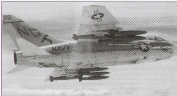
Outbound on a mission in 1970, VA-147 A-7E BuNo 156827 carries a load of Mk 83 bombs (Norm Birzer)
