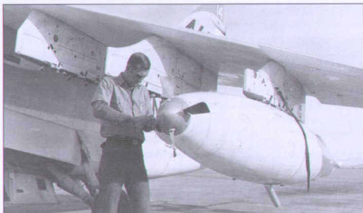
A close-up view of the D-704 in-flight refuelling store – this particular example is carried by a shore-based A-7A of VA-37. The short-bladed propeller on the nose of the tank provided power for extending and retracting the hose
