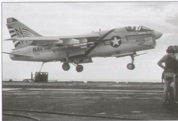
A-7E BuNo 157526 of VA-195 returns to Kitty Hawk after a mission. Note the position of the main wheels (canted outboard) and the raised tow bar on the nosegear. The aircraft carries a full assortment of MERs, indicating that its bombload had been fairly heavy
