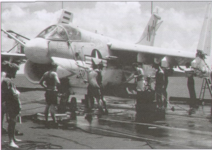
Hard work in a hot, humid environment – washing off corrosive salt is a daily activity for deck crews on deployment. These crewmen are attending to VA-192's A-7E BuNo 157457 aboard Kitty Hawk in 1971. Nicknamed the 'World Famous Golden Dragons', VA-192 had what might be arguably considered the most colourful paint scheme of any A-7 squadron in South-east Asia. This particular Corsair II had the misfortune of landing aboard the wrong carrier in January 1971, much to the collective embarrassment of the pilot and his squadron
