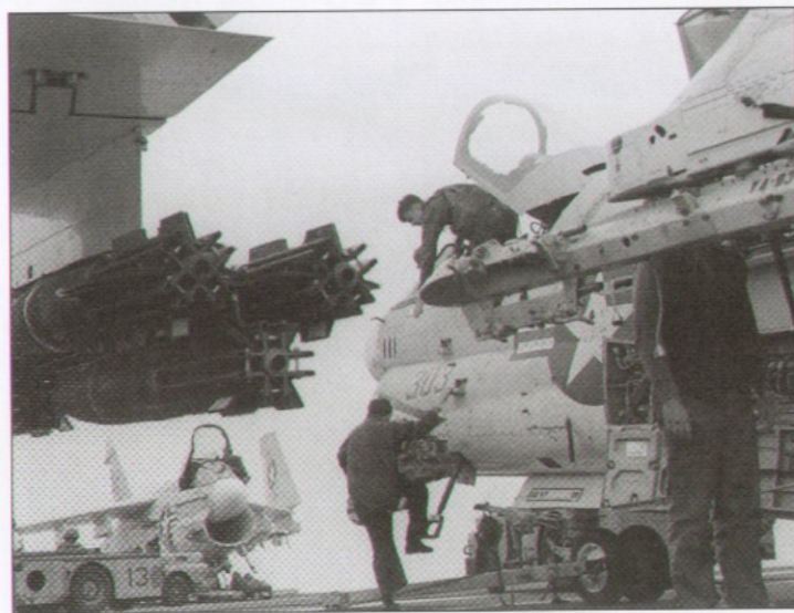
Mk 82 Snakeyes hang from an A-7's MER as deck crews ready their Corsair IIs (from VA-56 and VA-93) for yet another mission during Ranger's 1970 combat cruise (Charles Minke)
