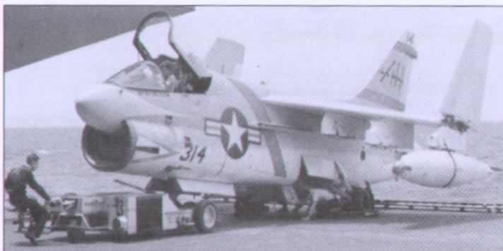
Equipped with a D-704 buddy store on station one, A-7B BuNo 154421 of VA-87 is being prepared for a tanker mission off the Vietnamese coast in the spring of 1969 (Fred Ameel)
