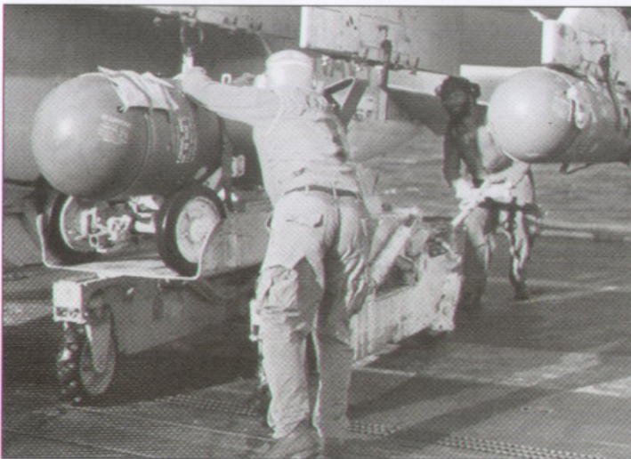
Ordnancemen from VA-94 load maritime mines aboard a squadron A-7 in May 1972
