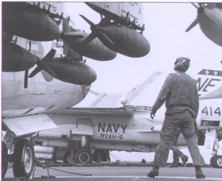
Looking through the maze of bombs carried by a VA-147 A-7 in January 1968. Note the tie-down chains linking the nose landing gear to the pad-eyes on the flight deck (US Navy photo by PH1 Donald F Grantham)
