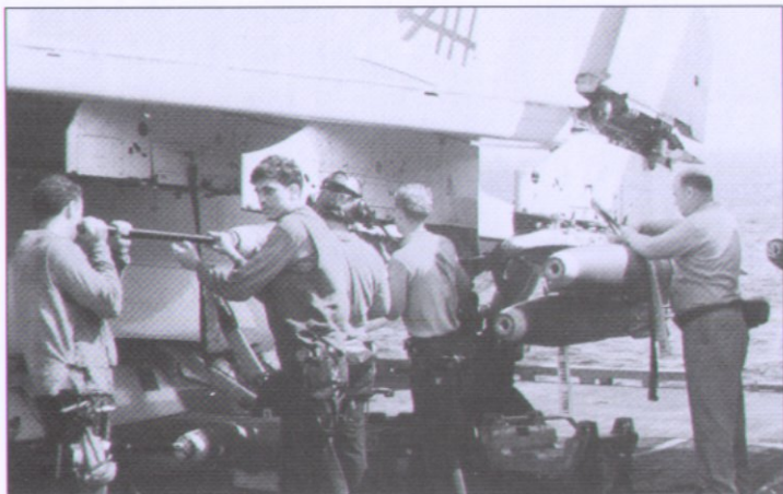
Red-shirted 'Ordies' from VA-87 mount and then fuse low-drag Snakeye bombs beneath the port wing of an A-7B aboard 'Tico' in 1969
