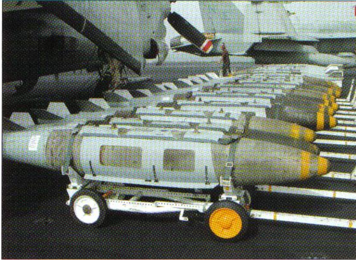
Recently brought up from CV-64's hangar deck, 20 GBU-31(V)2/B JDAM sit on their individual Aero-12C skids awaiting dispersion to the Tomcats and Hornets assigned to the opening strikes of 'Shock and Awe' (PH2 Dan McLain)
