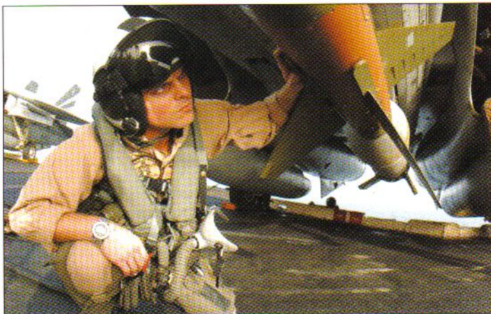
A pilot checks the guidance vanes on a GBU-24 Paveway III LGB. The weapon's larger stabilisation package on the back allows it travel farther in flight (PH3 Todd Frantom)
