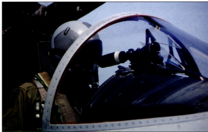
Sniper scopes were fitted to many F-15Cs during Desert Storm to allow early identification of aircraft that were still beyond the visual acuity of the human eyeball. This particular example is seen bolted onto the cockpit coaming of a 1st TFW jet at Dhahran. (Ian Black via Author)
