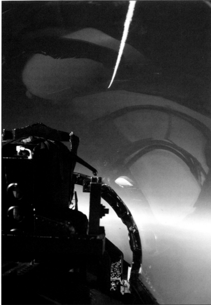
This dramatic photograph shows the launching of an AIM-120 AMRAAM from an F-15D. The weapon has rapidly climbed to altitude after being fired, at which point it starts contrailing. Ultimately, it will impact a Firebee target drone. (Gary Klett via Author)
