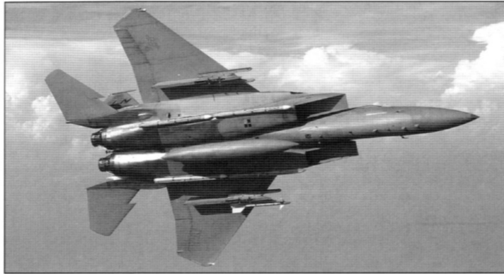
Loaded with four inert AIM-7 Sparrow captive carry missiles on its underfuselage mountings and a single inert AIM-9 training round on the left outboard wing pylon, this F-15C reefs into a sharp turn for the benefit of the camera. With external fuel tanks jettisoned, the Eagle can pull up to 9G without adversely affecting the missiles. (Gary Klett via Author)
