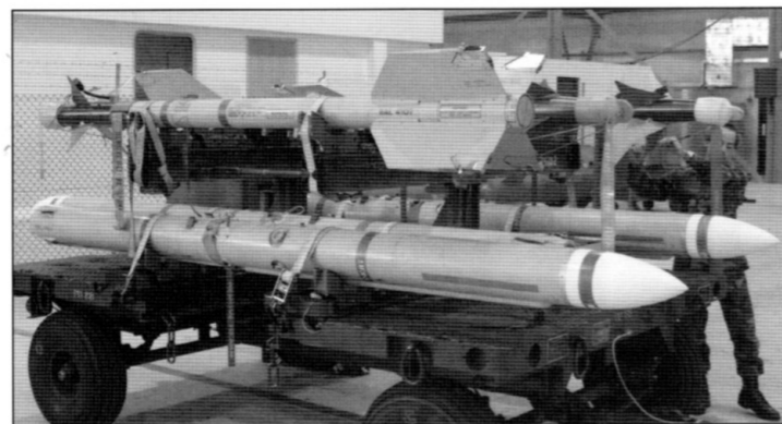
Training versions of the AIM-9 and AIM-7 await loading. The AIM-7 packed a hefty punch that shredded the aircraft against which it exploded – very often there was little left of the target, particularly if the red hot iron rods of the warhead punctured its fuel tanks. (Author/FJPhotography.com)
