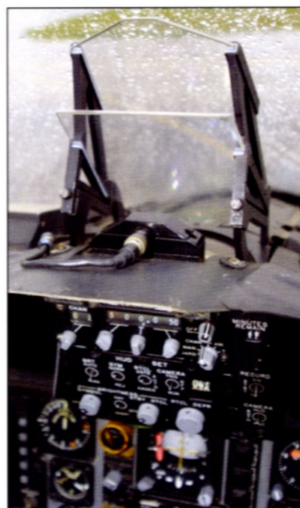
Above and top The F-15's ergonomic cockpit, HOTAS controls, and superb HUD were revolutionary. These images show the Eagle cockpit following the 1983 MSIP II programme, which introduced to the cockpit a new display and enhanced HOTAS controllers. (Author/FJPhotography.com)
