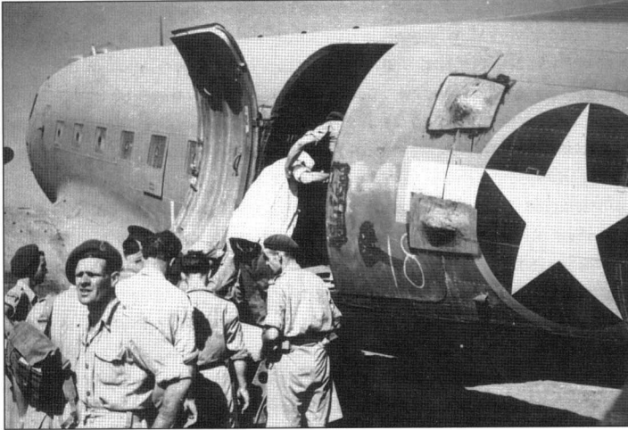
Casualty evacuation C-47s were often the first Allied aircraft into any liberated airfield, bringing in fuel and munitions for forward-deployed fighters. Here, a C-47 on a casualty evacuation mission from Sicily picks up wounded British soldiers. It carries red-bordered insignia and a chalk marking. Note also that the main cargo door hinges have been crudely reinforced 'in the field'. The gunports in the fuselage windows are also clearly visible (National Archives)
