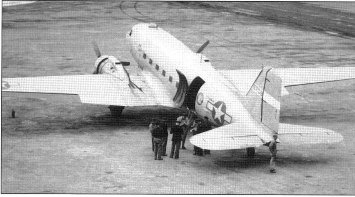
Photographed in Algiers in June 1945, this natural-metal C-47B of MATS/EATS was marked with the 'last four' on a coloured fin band (probably repeated on a nose diamond) and the ATC insignia on the rear cargo door. Even though glider towing was never an ATC mission, note that the streamlined tail cone has been removed ( National Archives )
