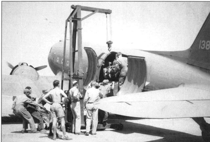
An engine is loaded aboard a C-47 'somewhere in the MTO' in the spring of 1943. One of the most important transport missions flown by the C-47 was the support of Allied air power throughout the MTO, including the airlifting of engines and repair teams to aircraft stuck on forward airfields (National Archives)
