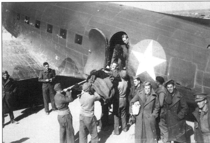
This early-production C-53 transport (basically a DC-3 without airline fittings, and with gunports in the fuselage windows) is seen carrying out a casualty evacuation mission for the British Eighth Army at a forward desert airstrip in the early autumn of 1942. These transports were among the first US-marked aircraft to be committed to the North African campaign, preceding the arrival of the 316th TCG in November 1942. Some were later transferred to the RAF as Dakota Is, while others flew on to the China-Burma-India theatre (National Archives)
