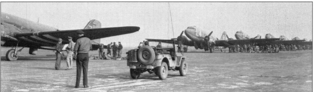
Ready to transport 388 paratroops of the 82nd Airborne Division to Holland, C-47s from the 439th TCG are lined up at Balderton on 17 September 1944. Note the SCR-717 ground-mapping radar radome beneath the fuselage of the C-47 (43-15159) closest to the camera. This aircraft was flown by the group CO, Lt Col Charles H Young (via Roger Freeman)
