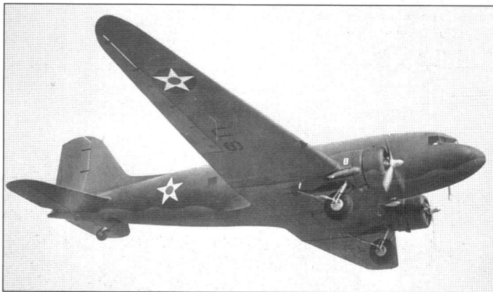
This DC-3 was impressed as a C-49C (one of two ex-Delta Airlines) or C-49D (11 ex-Eastern Airlines) model, powered by Wright Cyclone engines (National Archives)
