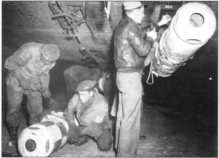
During Operation Manna , external cargo was carried in British-type parapacks with Mk III containers – seen here being loaded under a C-47 by British paratroopers and 51st TCW aircrew at Foggia (National Archives)
