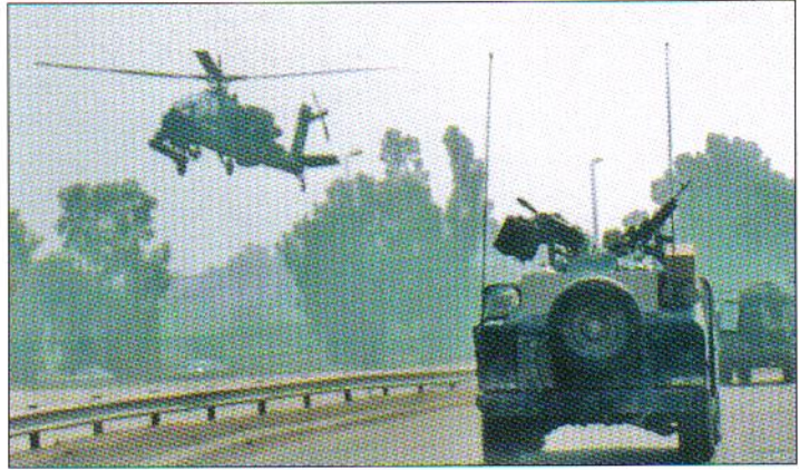
Increasing threats from the Sadr City district of Baghdad warranted increased Apache patrols over the city in support of 1st Cavalry troops sweeping the area in August 2004. Here, a 1-1 AVN AH-64 covers a heavily armed and armoured Humvee fitted with an M240B and a MK19 automatic grenade launcher (US Army)
