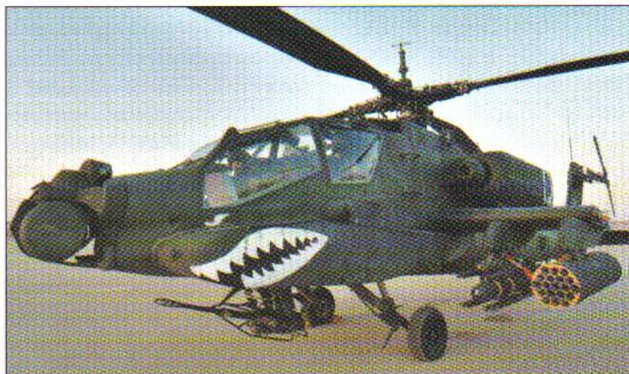
Featuring a newly applied 'sharkmouth', this 4-3 ACR AH-64A carries the now-standard mission load-out of one IR Hellfire and two rocket pods per stub wing (via John Musick)
