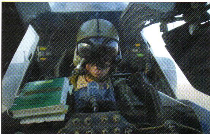
Visor down, IHADSS (Integrated Helmet and Display Sight System) monacle extended and mike boom in front of his face, CW3 Zac Noble looks more like a character from a B-grade horror movie than Pilot in Command of AH-64A 89-0245 DELIVERANCE (CW4 Zac Noble)
