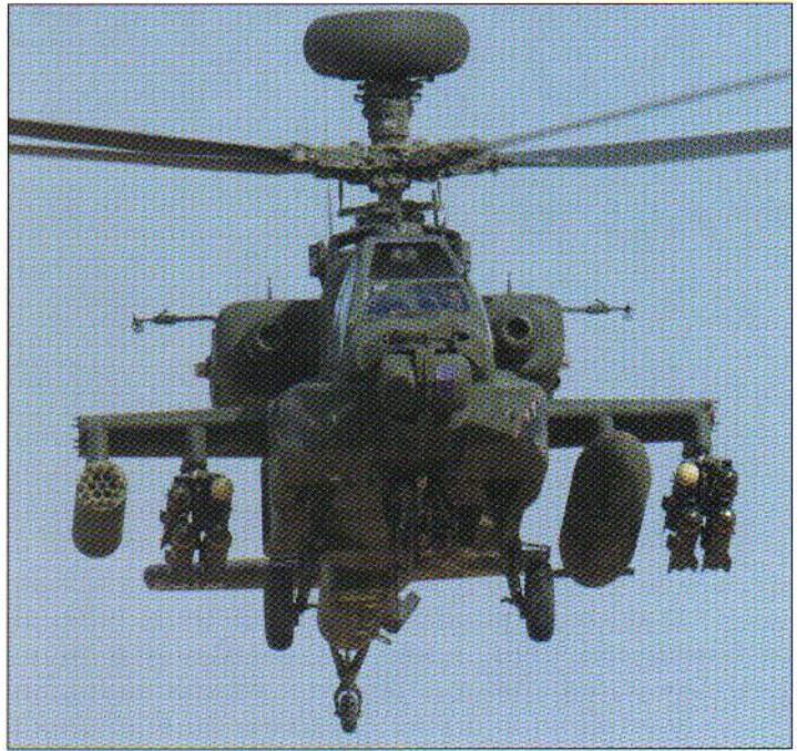
'Viper 04' carries a modified Hellfire load, whereby one of its M261 pods has been replaced by an external fuel tank. This configuration was adopted post-war, when mission duration rather than firepower became more important to 'Vipers' crews (CW3 Michael S Madura)
