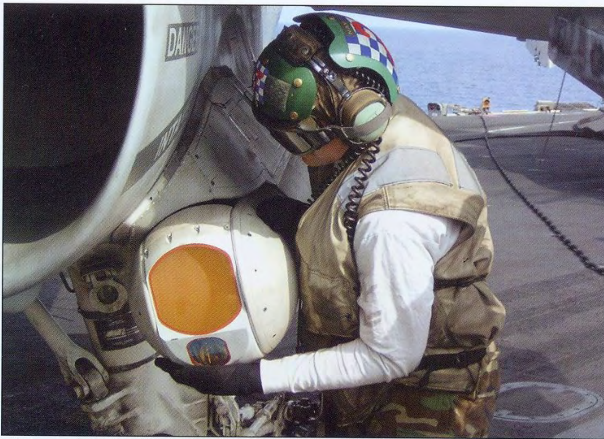
A VFA-105 plane inspector checks the optics of the AN/AAS-38A NITE Hawk target designation pod prior to the jet being unchained and marshalled to a catapult. State-of-the-art 15 years ago, the NITE Hawk struggled in OIF, and the system is now being replaced by the ASQ-228 ATFLIR in fleet service (Cdr Tom Lalor)
