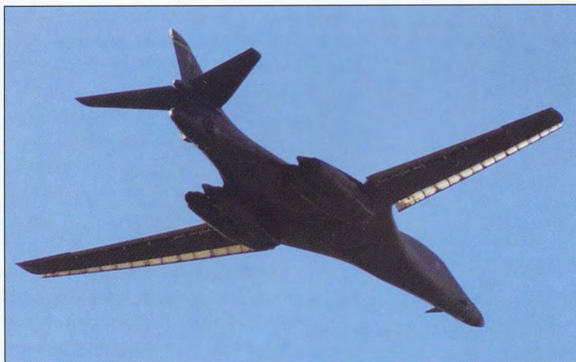
A Bone from the 37th BS/28th BW shows off the dramatic forward sweep of the Lancer's wings, which give the aircraft a reduced take-off run and greater range. The leading-edge slats on the wings are clearly visible, along with sleek shape of the 'Bone', which goes a long way to decreasing the aircraft's radar signature (28th BW)
