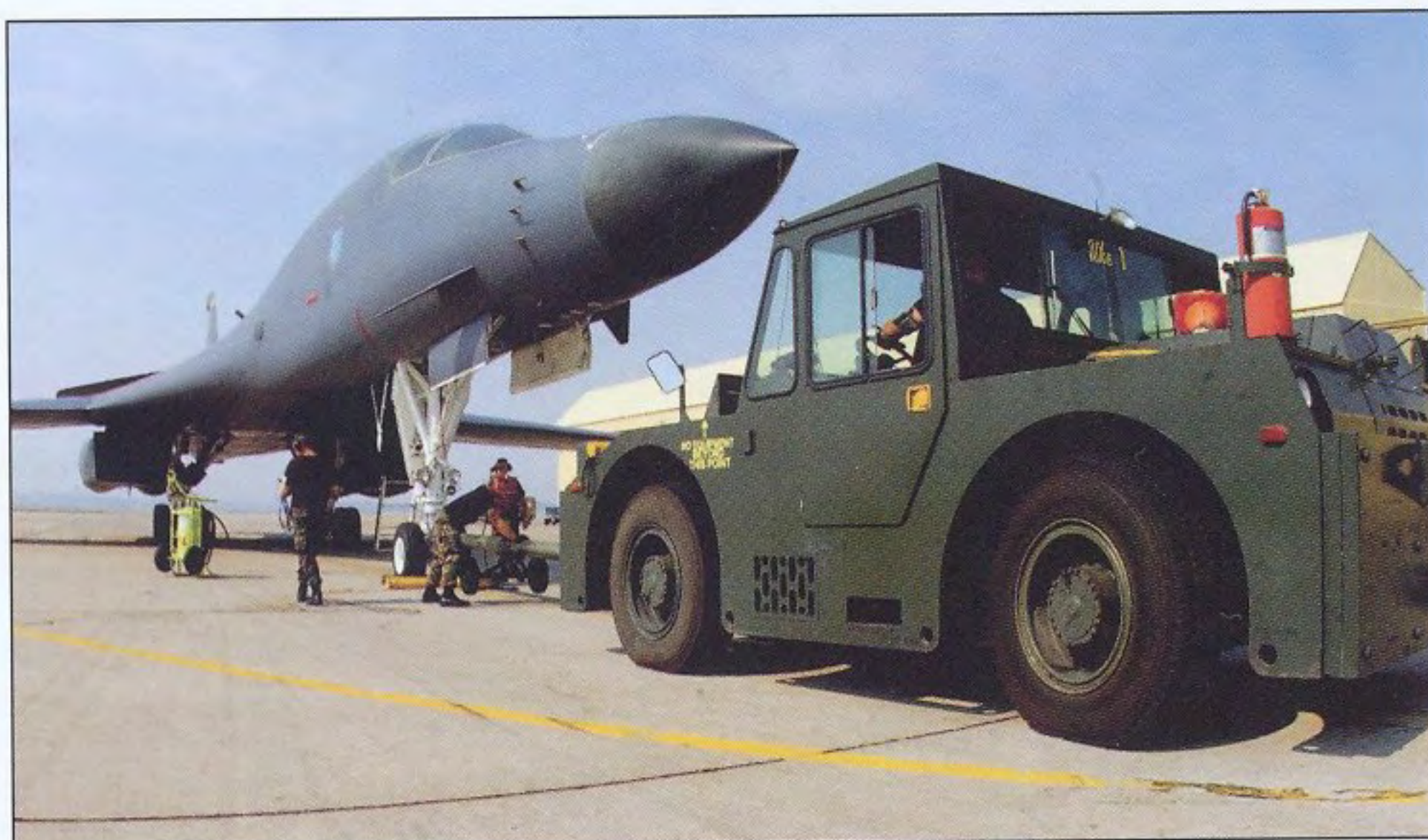
Ready for pushback. A B-1B Lancer of the 37th BS/28th BW is manoeuvred on the ramp at Ellsworth AFB. The outward design of the B-1B differs little from its predecessor, although the cockpit area reveals the main differences between the two aircraft – notably the nose-mounted AN/APQ-164A radar housing, the cockpit windows and the foreplanes (28th BW)
