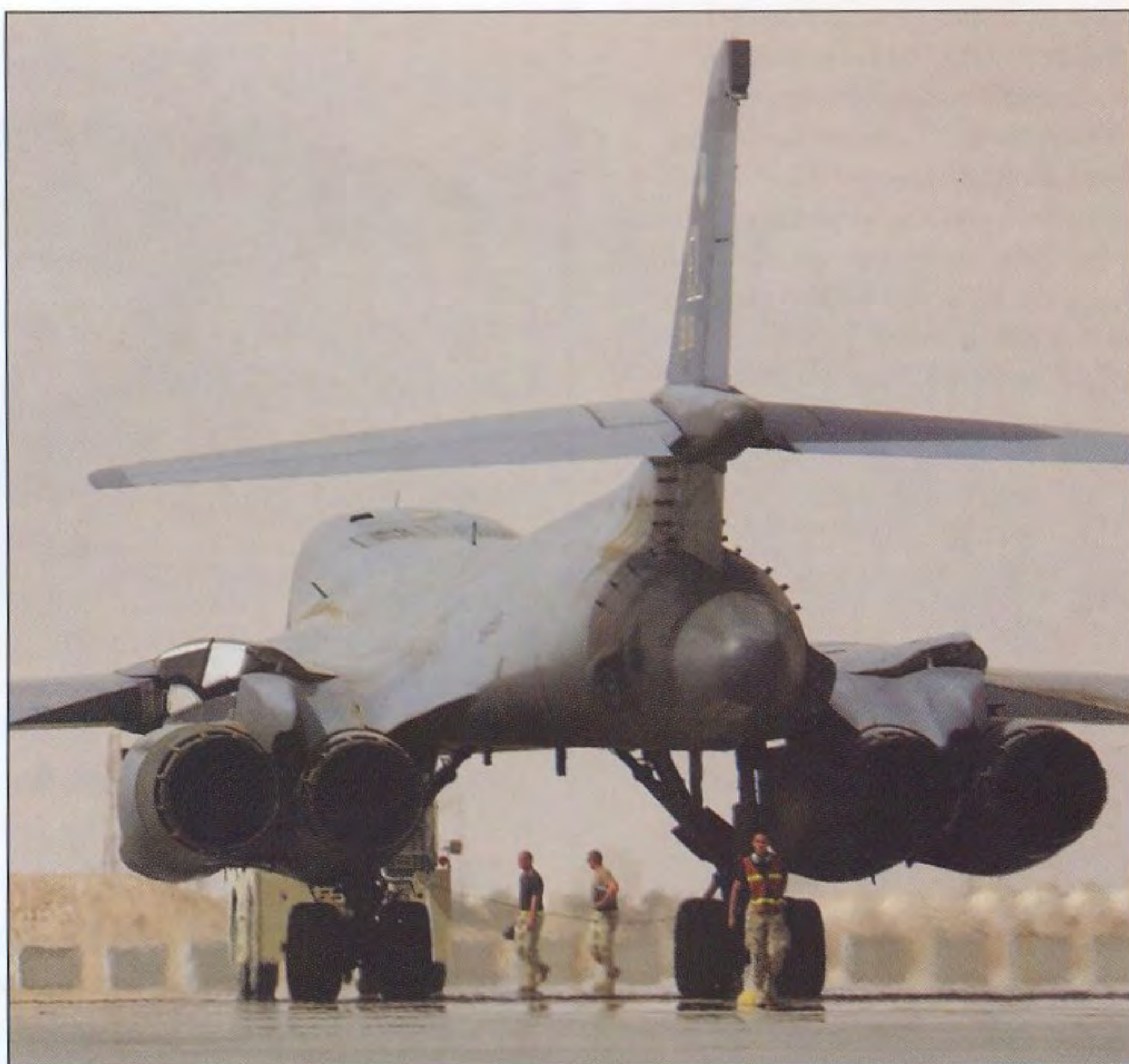
The aft area of the Lancer houses the defensive electronics and countermeasures that enabled the bomber to defeat the robust air SAM and AAA defences which surrounded Baghdad (B-1B Systems Program Office)
