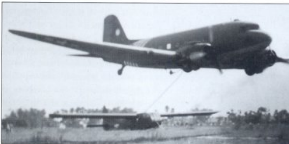
A C-47 of the 1st ACG demonstrates a unit specialty known as the 'glider snatch' at Hailakandy, in India. This tactic was used to extract both casualties and units in the Chindit campaign, along with the few surviving gliders from Broadway , Chowringhee , Clydeside and other forward airstrips (National Archives)
