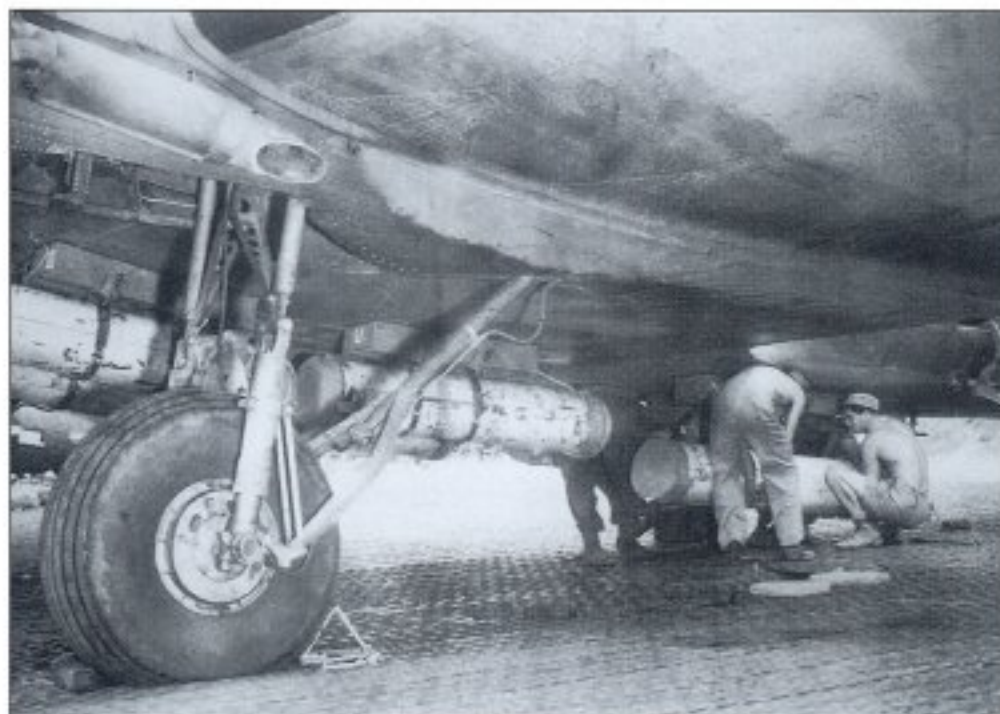
Jettisonable parapacks of British design are fitted to temporary external hardpoints beneath a CCTF C-47 in preparation for Operation Dracula (National Archives)
