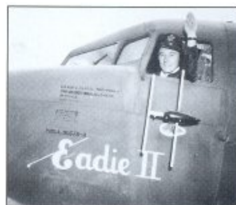
Maj Lewis Burwell, CO of the 27th TCS, waves from the pilot's seat of his C-47, Eadie II . The 27th became the first transport squadron to be permanently based in China after it had supported the Chindits and participated in the airlifts to Imphal and Myitkyina, in Burma. The under-cockpit Rebecca antenna is of the early design, recognisable by light-coloured vertical elements. Burwell was a strong and forceful commanding officer of a unit that, alongside the 315th TCS, joined the Air Commandos and the RAF in supporting the Chindits while the 1st and 2nd TCS worked with Stillwell's forces to the north in 1944. In 1945 the 27th moved to China to make possible the successful Chinese counter-offensive along the Salween River ( National Archives )
