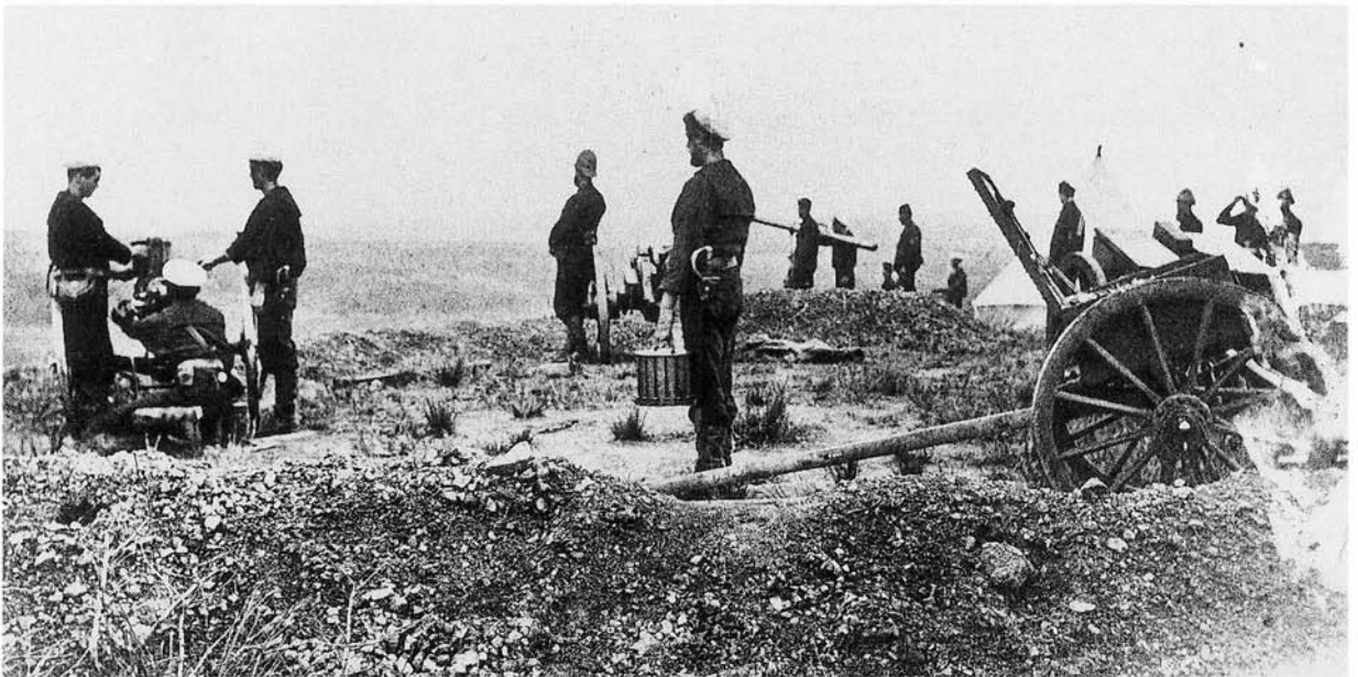
Royal Naval detachment from HMS Tenedos on top of Fort Pearson, overlooking the Lower Drift of the Thukela, with Gatling (left) and limber (right). The Navy Gatling was mounted on a narrower carriage than the RA version, without the axle-tree boxes. The sailor centre is carrying an ammunition hopper. (Local History Museum, Durban)
