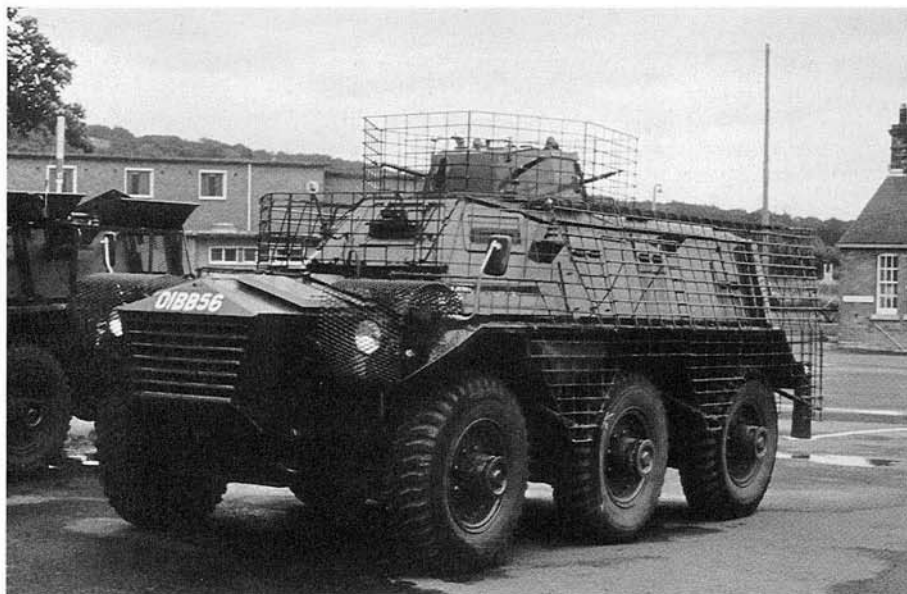
In 1973/74 Saracen APCs in Northern Ireland were fitted with anti-rocket mesh, under a programme called Operation 'Kremlin', to protect them from RPG-7 anti-tank rockets being used by the PIRA. (AIS HQ NI)
