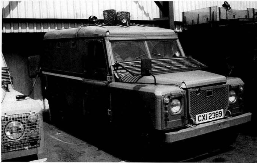
The first armoured Land Rover to enter service with the RUC was known as the Hotspur, is an up-armoured version of the Series III vehicle. (Bob Morrison/Military Scene)
