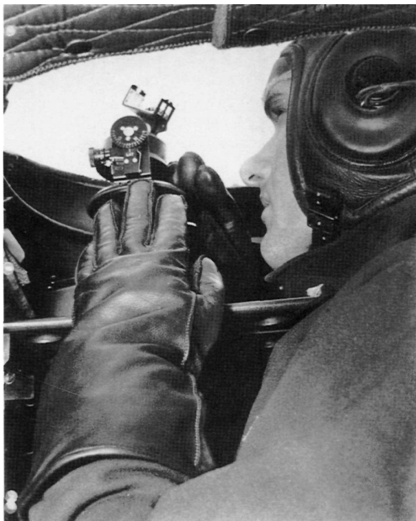
A navigator, operating an AN573N-1 astro compass, wears the F-2 electric heated gloves with an AN-
