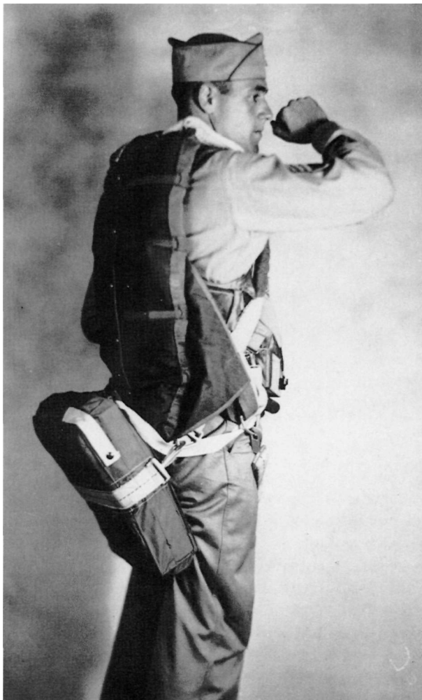
A B-8 back parachute with a C-2 one-man parachute raft case attached in the scat position, probably a test version. This staff sergeant also wears a B-4 life vest and C-1 emergency vest.
