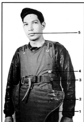
A 36th Troop Carrier Squadron C-47 flight engineer displays the M1 armour vest and M3 apron he wore during Operation 'Market Garden': a single 7.92mm bullet struck at point No. 4, and the other points indicate where bullet fragments struck. This photo is part of the series distributed to airmen in an effort to convince them to wear the heavy flak suits.
