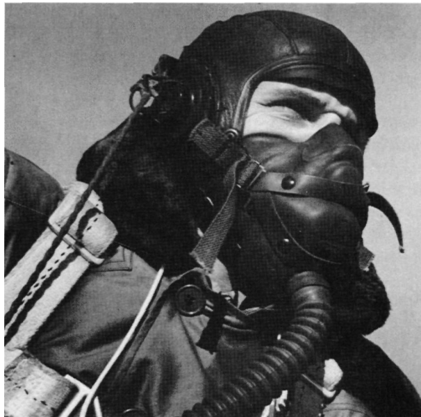
Details of the A-14 oxygen mask retaining strap along with the A-11 intermediate helmet and B-9 winter jacket.
