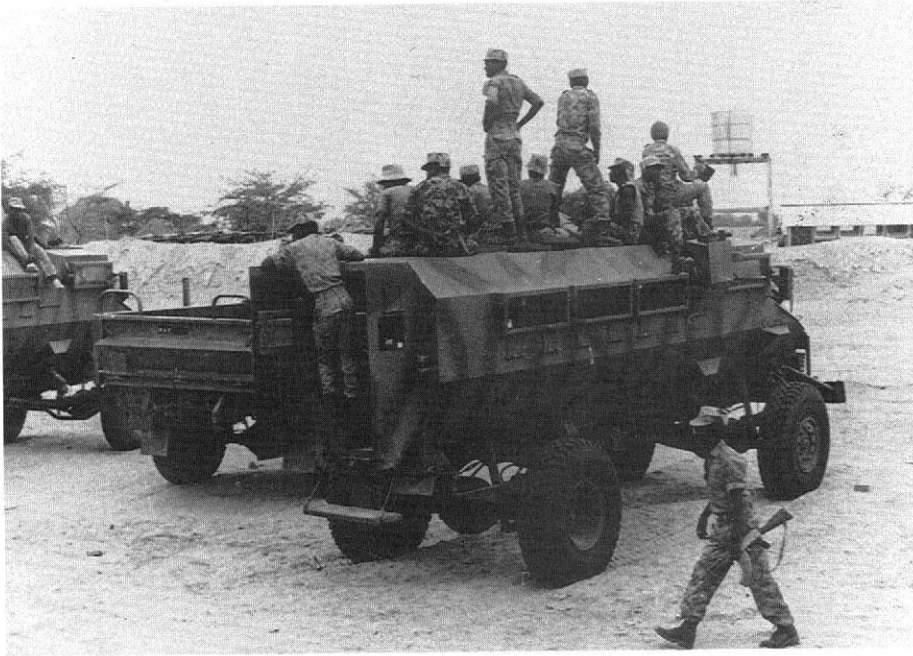
A Koevoet unit prepares to leave Oshakati for an operation in the bush, 1981. The second model Police Casspir is in use, distinguished by the fold-down door immediately in front of the side windows. (South African Police)
