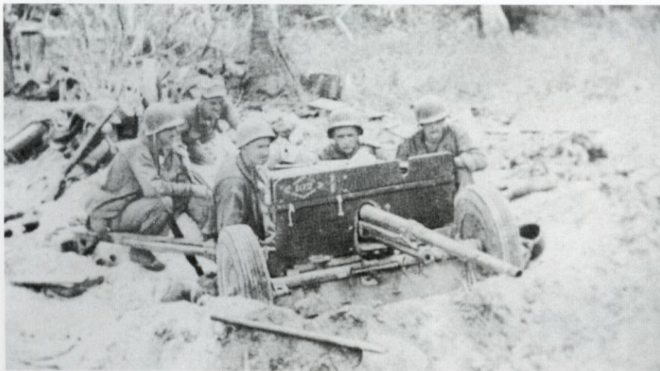
A 37 mm anti-tank gun bears the stencilled yellow 1st MarDiv unit marking on its shield. While intended as an AT weapon firing an armour-piercing projectile, the Marines employed it mainly for infantry support using high explosive and canister rounds.
