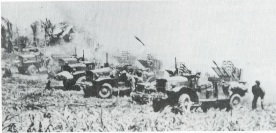
Left: Mounted on 1 ton trucks, the 1st Provisional Rocket Detachment of 4.5 in. T45 launchers fires on Japanese positions on Saipan. The 4.5 in. M8 rockets had a range of 4,600 yards.
