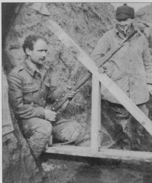
The No.3 or 'J Pattern' Hale rifle grenade being fired from an SMLE rifle in a wooden launching stand; range was up to 150 metres. The No.3 burst well but had over-complex safety mechanisms.
