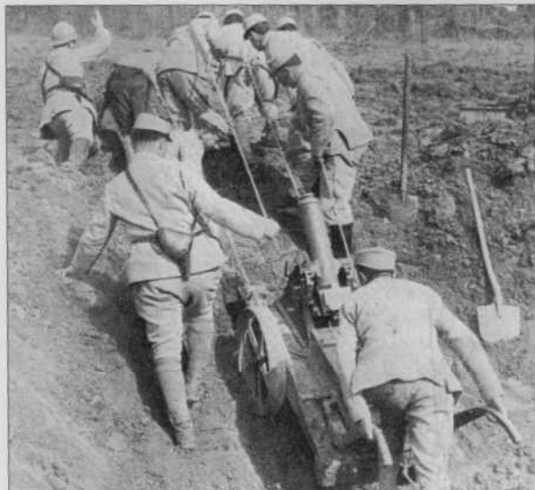
Hauling a French trench mortar into position using the two-wheeled hand barrow. (Section Photographique de l'Armée Française)
