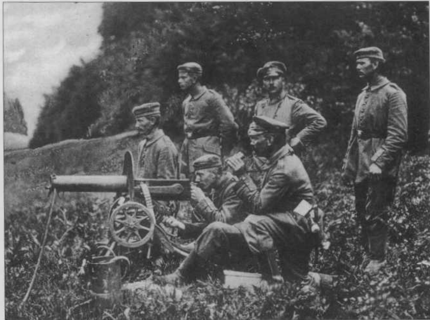
German troops with a captured Russian M1905 Maxim gun. Note the Sokolov wheeled mount, with folding legs which could be swung down to form, with the trail, a tripod - cf Plate H. As with most water-cooled weapons, the hose and can allowed steam generated by water boiling in the barrel jacket to be led off, condensed, and later recycled. Some steam usually escaped, drawing attention to the gun's position.
