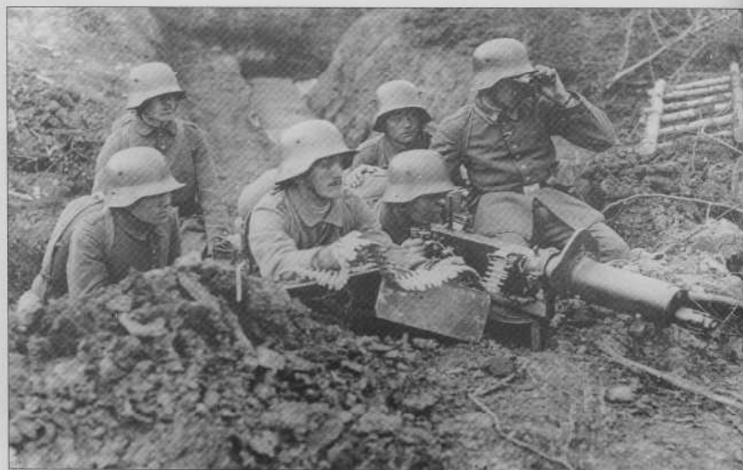
A German MG08 on an improvised 'trench mount'. This arrangement was less stable than the 'sledge' mount but much easier to move.
