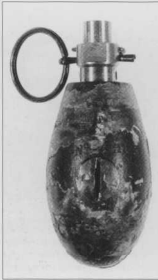
The British No.34 'egg grenade' which was introduced in 1918 to counter the similar German bomb. It was made in four versions; this is a Mk.III of March 1918. After removing the safety pin the user struck the plunger of the Adams striker mechanism against a hard surface, such as his boot, and a .22in cap ignited a five-second time fuze. The No.34 measured 3.9in x 1.9in, and weighed 12oz when filled - usually with Alumatol, indicated by a pink band painted round the casing.
