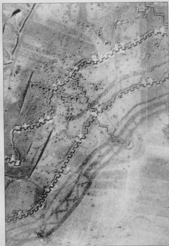
Trenches near Cambrai seen from the air; No Man's Land is at bottom right. This clear aerial photo shows the pocking of shellholes, the stark crenellated lines of two fire trenches, the lazy zig-zag of communication trenches, the shadows cast by belts of wire, and D-shaped advanced posts pushed out beyond them.
