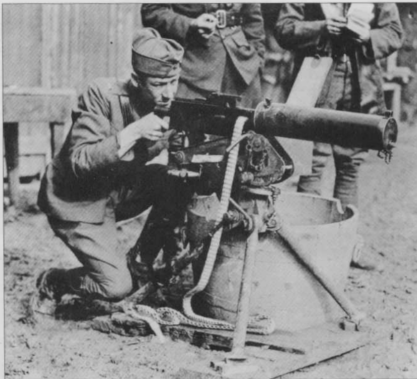
Thillombois, October 1918: American Lt.V.A.Browning firing the .30in M1917 machine gun invented by his father John Moses Browning. A conventional recoil-operated, water-cooled, tripod-mounted weapon in the tradition of the Maxim and Vickers, capable of delivering sustained fire, it was selected as the US Army's principal machine gun in May 1917, and some 27,000 were eventually sent to the AEF. Each three-battalion infantry regiment had a 16-gun MG company; each brigade had a three-company MG battalion, and each division a four-company MG battalion.
