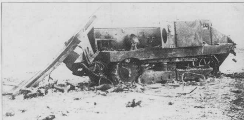
Postcard illustration of a wrecked French Schneider tank, and the remains of some of its crew. Early Schneiders were dogged by a lack of spare parts, an alarming susceptibility to German armour-piercing 'K' bullets, and fuel tanks which were prone to ignite. One wonders at the reaction of Fraulein Sophie Cöster of Warburg on receiving this picture from 'her Rudolf'.
