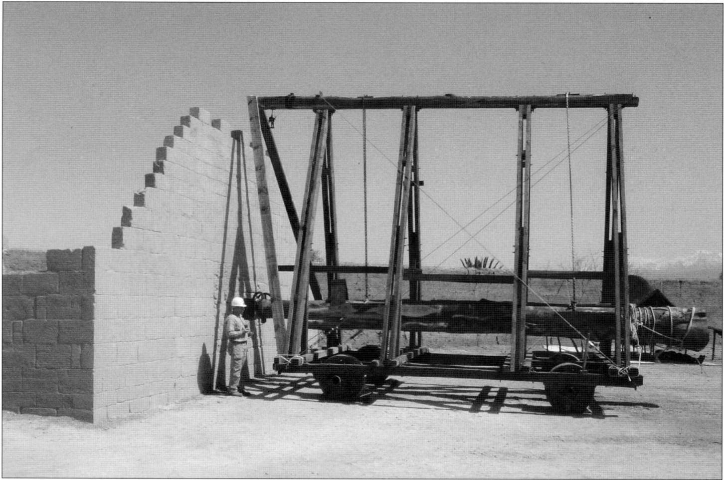
A reconstruction of the ram tortoise described by Apollodorus of Damascus. The outer cladding of timber and wickerwork, covered with a fireproof layer of clay, has been omitted, so that the frame and undercarriage can be seen. (© P. Slisz)
