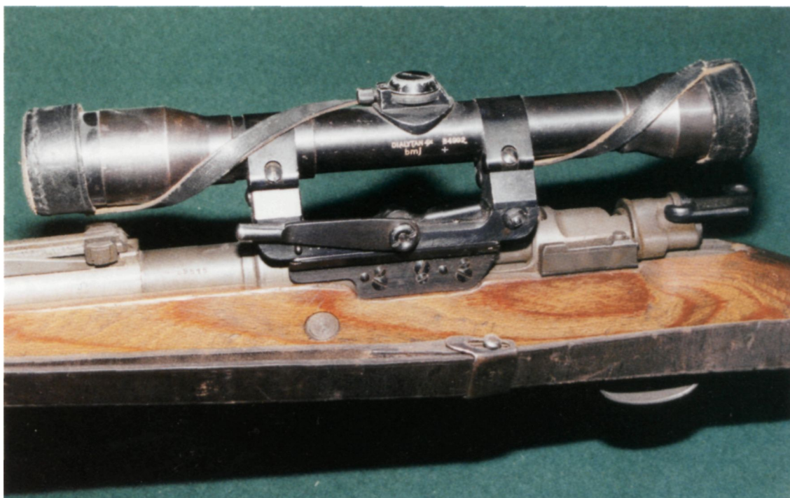
A post-1943 short side-rail Mauser with 4x Dialytan telescopic sight and leather lens cover (G. Sturgess collection)
