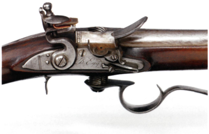
The breech of a Ferguson Rifle, in the open position. Hand cutting the threads on the breech plug was an exacting and time-consuming task, but the benefits were certainly worthwhile. This rifle was Ferguson's personal weapon. (The Board of Trustees, Royal Armouries D12003-339)
