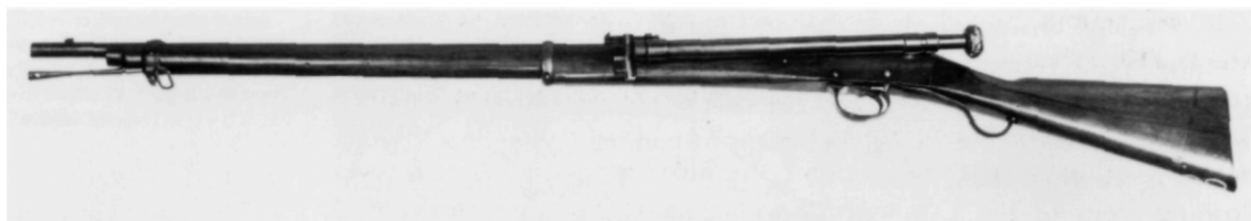
An experimental Martini-Henry rifle with Davidson pattern telescopic sight. It was the first purpose-designed centrefire rifle adopted by the British Army. (MoD Pattern Room Collection)
