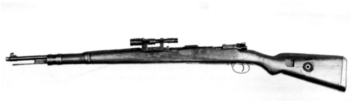
A Mauser K98k with Zf41 scope. The extreme eye relief is very clear in this picture. The best one could say of this scope was that it was marginally better than nothing. (MoD Pattern Room Collection)
