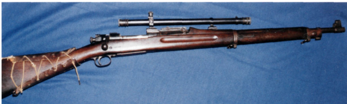
A well-used USMC Springfield Model 1903 with Winchester A5 scope and a home-made leather cheek-rest. (Springfield Armory Museum and Historical Site)
