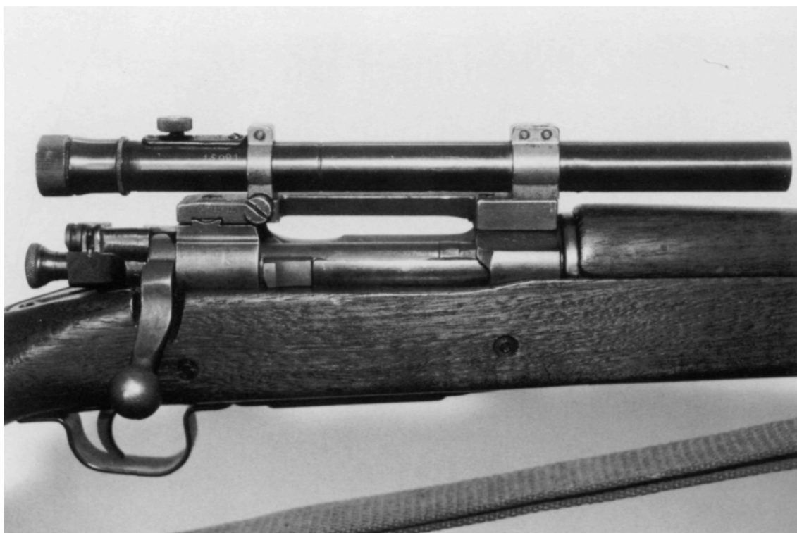
A, Springfield 1903-A4 with the M73 Weaver scope. It was an adequate, but not great combination, let down by the poor performance of the scope. (Jon Moore collection)
