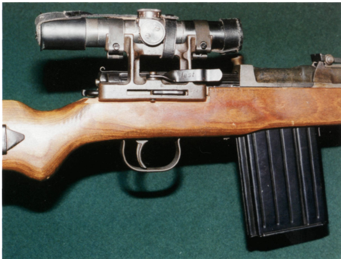
A close-up of the very compact and effective ZF4 scope and its quick-release mount. Unusually, the range drum on these scopes is placed on the right side. (G. Sturgess collection)
