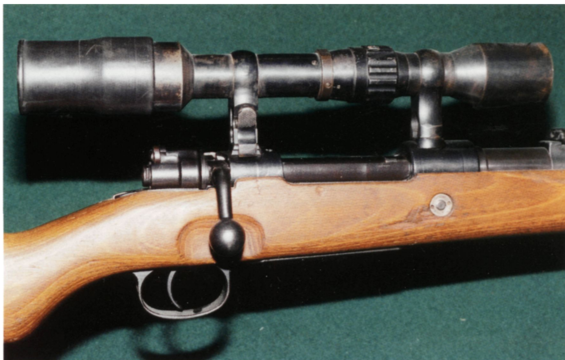
An SS issue double claw-mount K98k, showing the circular range drum on its Opticotechna scope body. (G. Sturgess collection)
