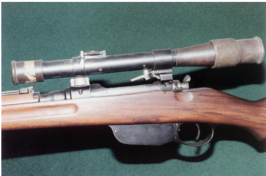
A Mannlicher with its distinctive scope mounting. The spring catch forward of the rear mount enables the scope to be unlocked and lifted clear. The leather eyepiece was a standard accessory. (G. Sturgess collection)
