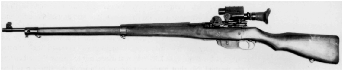
Ross Mk. III. with Warner and Swasey M. 1913 prismatic scope and its distinctive rubber-cup eye protector (MoD Pattern Room Collection)
