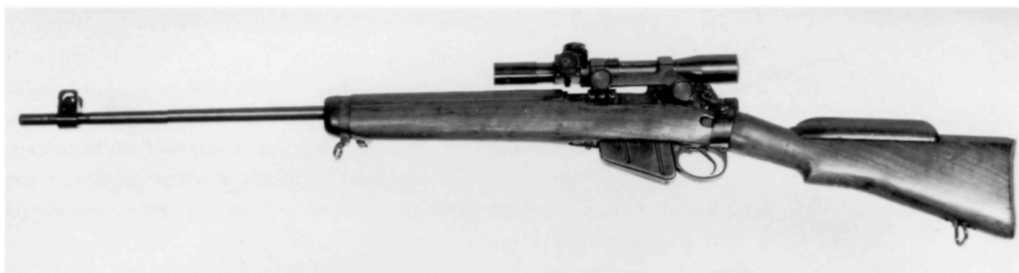
An early variant of the 7.62 mm Enfield L42 rifle. Basically a pared-down No. 4 (T) with heavier barrel, it still used the No. 32 scope. (MoD Pattern Room Collection.)
