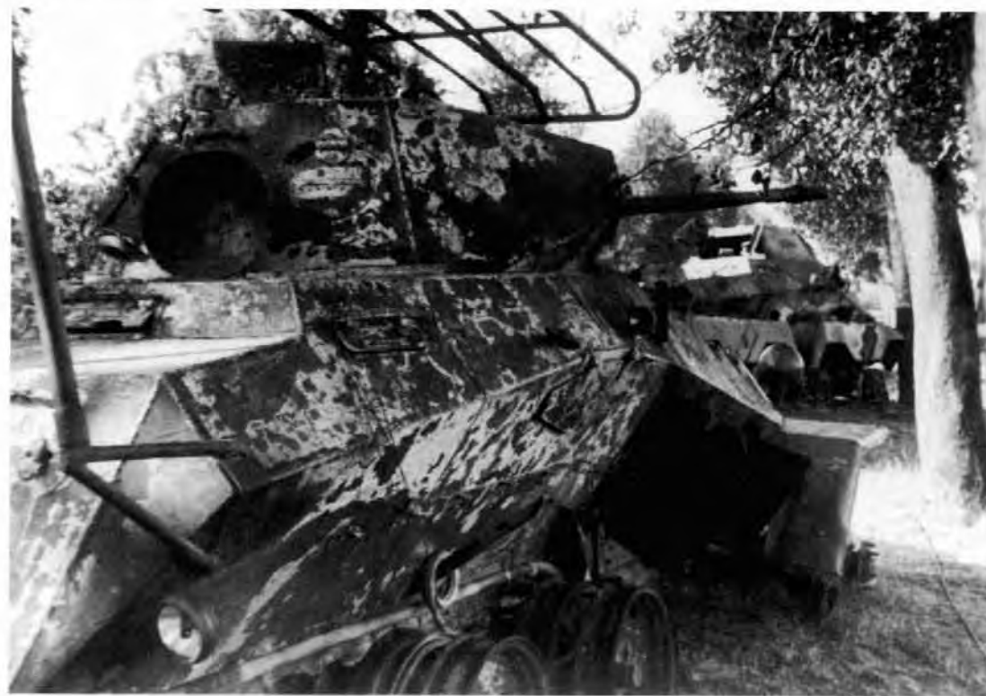
LEFT German losses at Arras. In the foreground a burnt out SdKfz 263 six-wheeled radio armoured car and, beyond, an SdKfz 231 eight-wheeled armoured car. (IWM RML 125)
