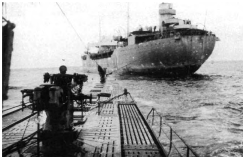
U-183, a Type IXD, is about to refuel at sea from a German tanker. The ability to refuel either from a tanker or from one of the Milchkuh submarines greatly extended the length of time a U-boat could remain on patrol. U-183 carried out 13 war cruises before herself being sunk by the US submarine Besugo on 23 April 1945.
