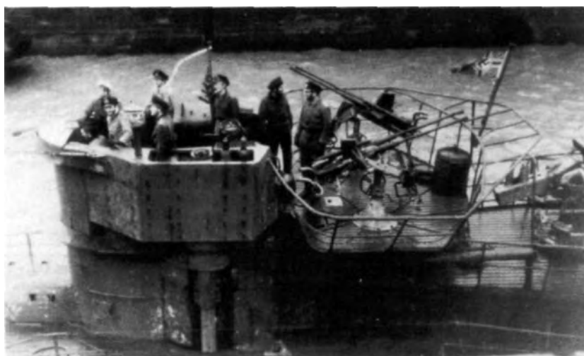
This shot taken from a dockside vantage point gives a good view down onto the extended flak platforms of a heavily armed Type VIIC with two 2cm flak Zwillinge and a 3.7cm flak
