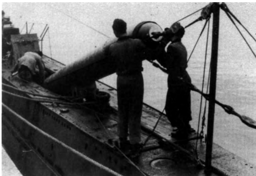
Loading torpedoes into the cramped interior of a Type II was an awkward and laborious business, requiring the use of special winches and pulleys, and much sweat and effort
