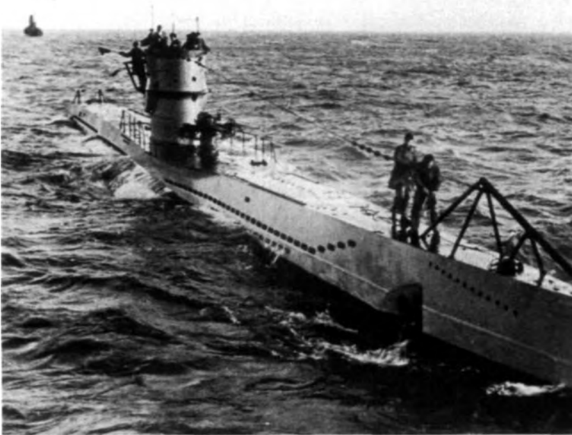
A typical Type VIIC running on the surface, again with net cutter still fitted. Note the narrowness of the foredeck compared with the roomier Type IX. Sailors needed to be sure-footed to keep their balance on such a narrow space in anything much more than a moderate swell.
