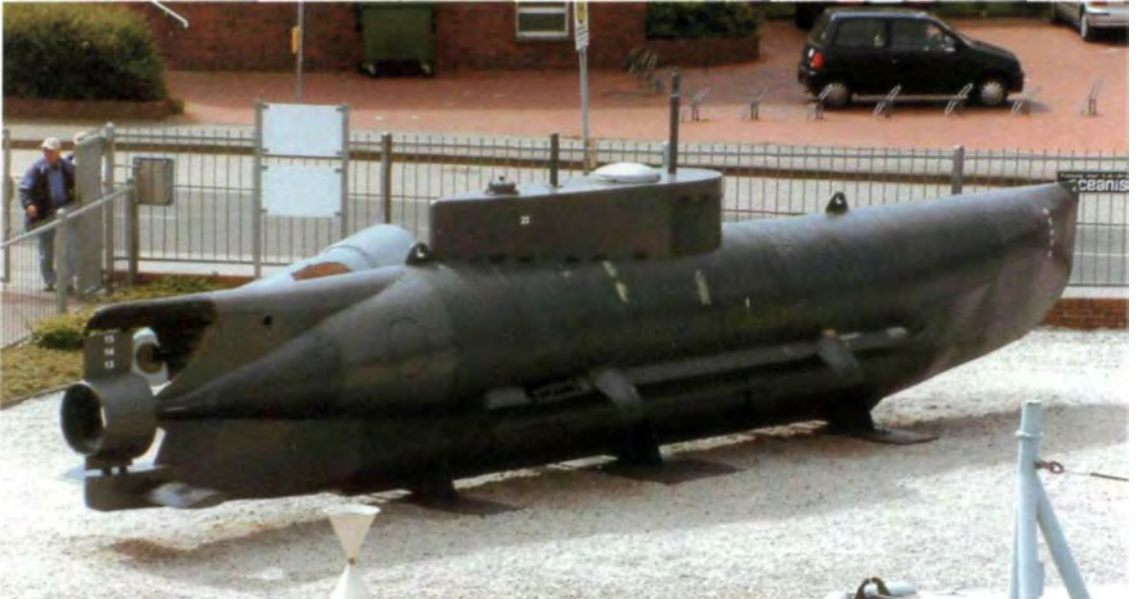
A surviving, partially restored example of the Seehund on display at the Maritime Museum at Wilhelmshaven. A further surviving example is on display at the naval dockyard in Wilhelmshaven. (Author's collection)
