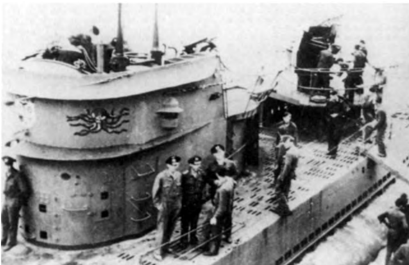
This interesting shot of a Type XIV tanker shows a special flak pedestal constructed on the after deck to carry a 2cm Flakvierling giving her enhanced anti-aircraft capability. A small walkway between the U-boat's Wintergarten platform and the additional pedestal can just be seen.
