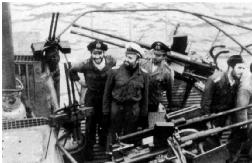
Some boats carried an extremely heavy flak armament in an attempt to give adequate defence against Allied aircraft. As well as the two 2cm flak Zwillinge on the upper platform, this boat has had two twin machine gun mounts fitted.
