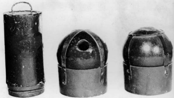
Canister, common shell (with fuze removed) and roundshot, illustrating wooden 'sabots' or shoes and methods of fixing projectile to sabot. Notice groove on canister sabot, to enable charge bag to be lashed on. (Kungl. Armémuseum, Stockholm)
