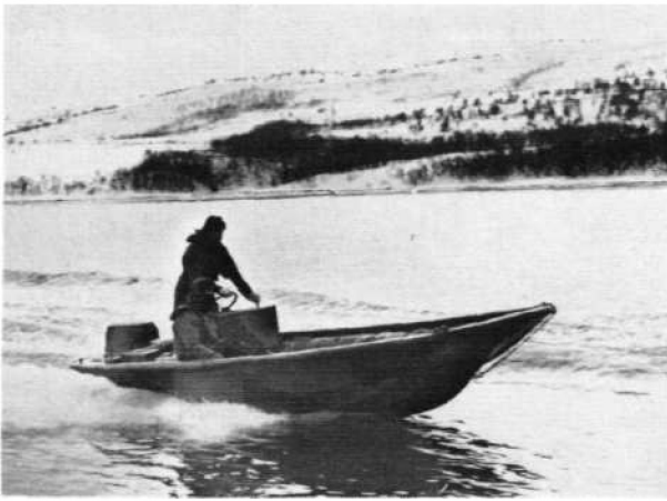
A Rigid Raider at speed in a Norwegian fjord. These small but powerful boats allow men and stores to be landed on small beaches, and can be driven up the beach beyond high-water mark by their own velocity. (Martin May, 45 Cdo.)
