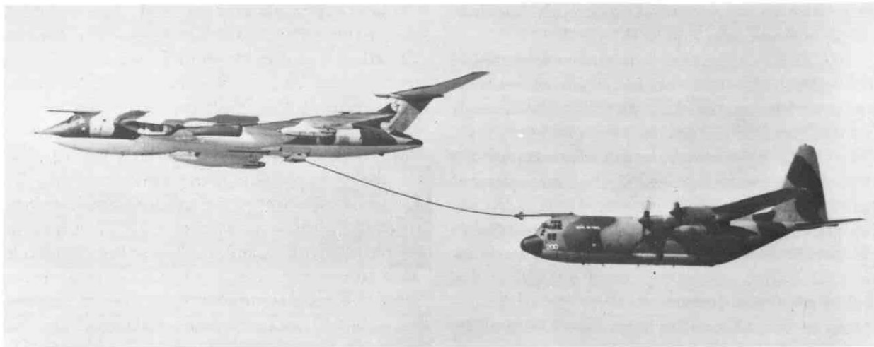
A Victor K.2 of No.57 Sqn. refuels a specially modified Hercules C.1 transport—a process repeated many times during the Falklands campaign. In-flight refuelling allowed the Hercules to become airborne with a heavier payload, without the usual trade-off in range. Special long-range missions were also flown by the Hercules to insert teams of SAS/SBS off South Georgia, and the mainland of South America. (MoD)
