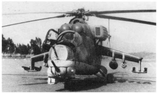
This DRA AF Hind-D was flown to Pakistan by its crew in 1985. The box-like structure above the stub wings is an infra-red suppressor for the engine exhausts, to confuse heat-seeking SAMs. This aircraft carries UV-32 rocket pods and 250kg bombs underwing.
