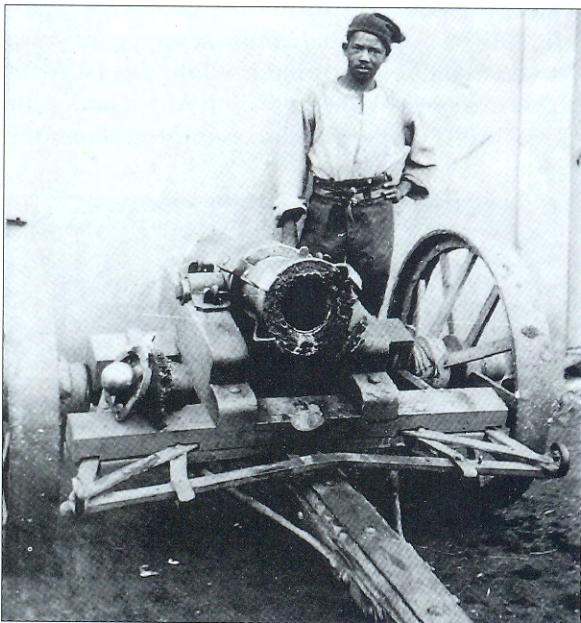
The Wolf – the most famous of the guns improvised by the British garrison during the siege of Mafikeng. This shows the damage after The Wolf burst in action. (Bryan Maggs Collection)
