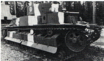
A T-28M which was captured early during the Continuation War and used by the Finns. The extra turret and sub-turret armour which distinguished this version from earlier T-28 variants is also evident on this photo (J. Cochran). Plans and modelling details for this vehicle appeared in Airfix Magazine Annual 5 .
