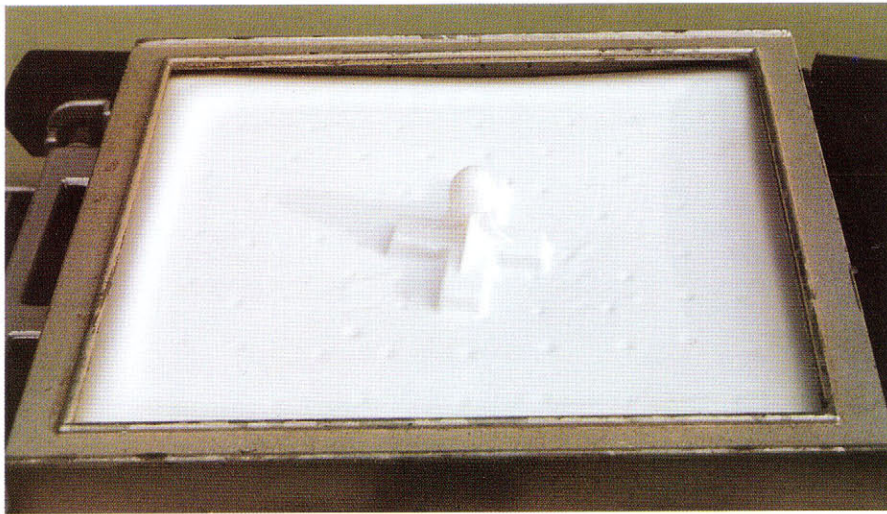
Left The plastic sheet after the vacuum pump has pulled it snugly down over the male mould.
