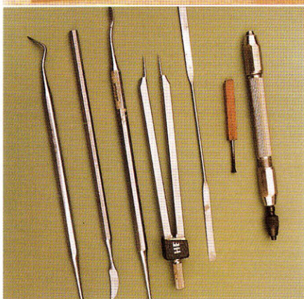
Above A selection of useful tools: from right, a pin vice with up to four different collets; a nail fixed into a wooden handle, for heat-sealing vinyl tracks; various metal carvers and spatulas, ideal for working with Milliput, etc., and a pair of dividers, useful for transferring measurements.
