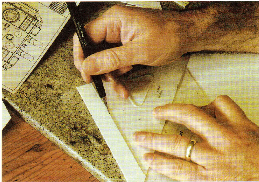
Above Two set squares, running along each other, enable perfect parallel lines to be drawn, in this case on plastic sheet.
