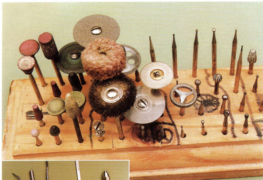
Left A selection of motor tool accessories. In this photograph the two accessories I use most often are the silicon rubber disc and the slitting disc (top row, third and fourth from left).
