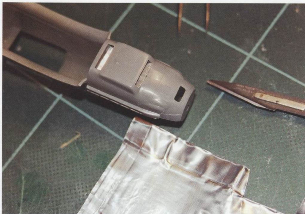
RIGHT A useful application for metal foil is as a lining for areas of a model that are difficult to reach for sanding.
