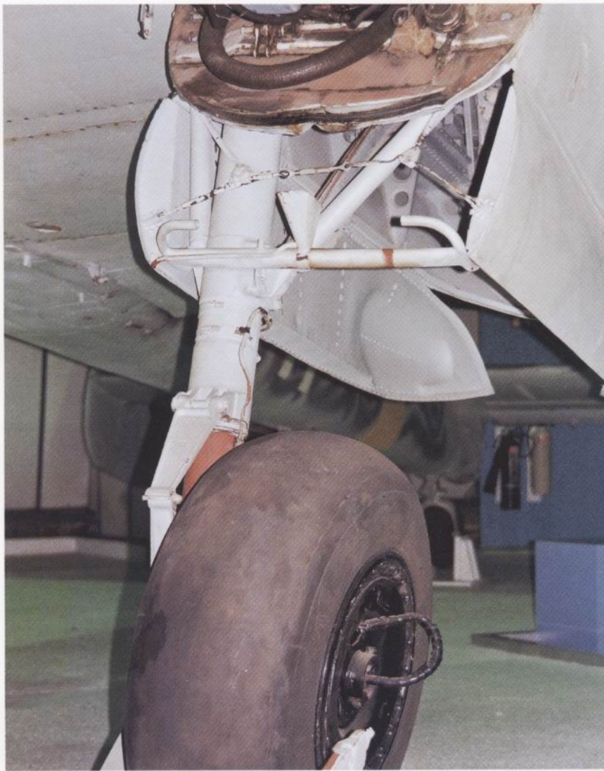
ABOVE The main landing gear of the Bf 110G-4 – notice the loop protruding from the main wheel hub.
