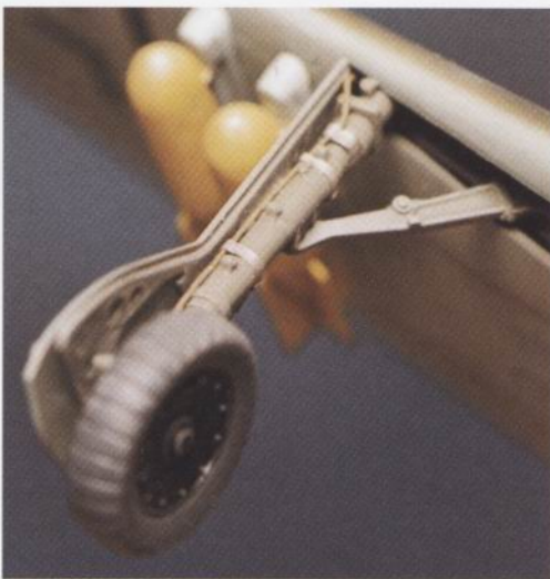
LEFT The leg of one of the author's Fw 190F-8s. Note the different arrangement for the hydraulic pipe.
