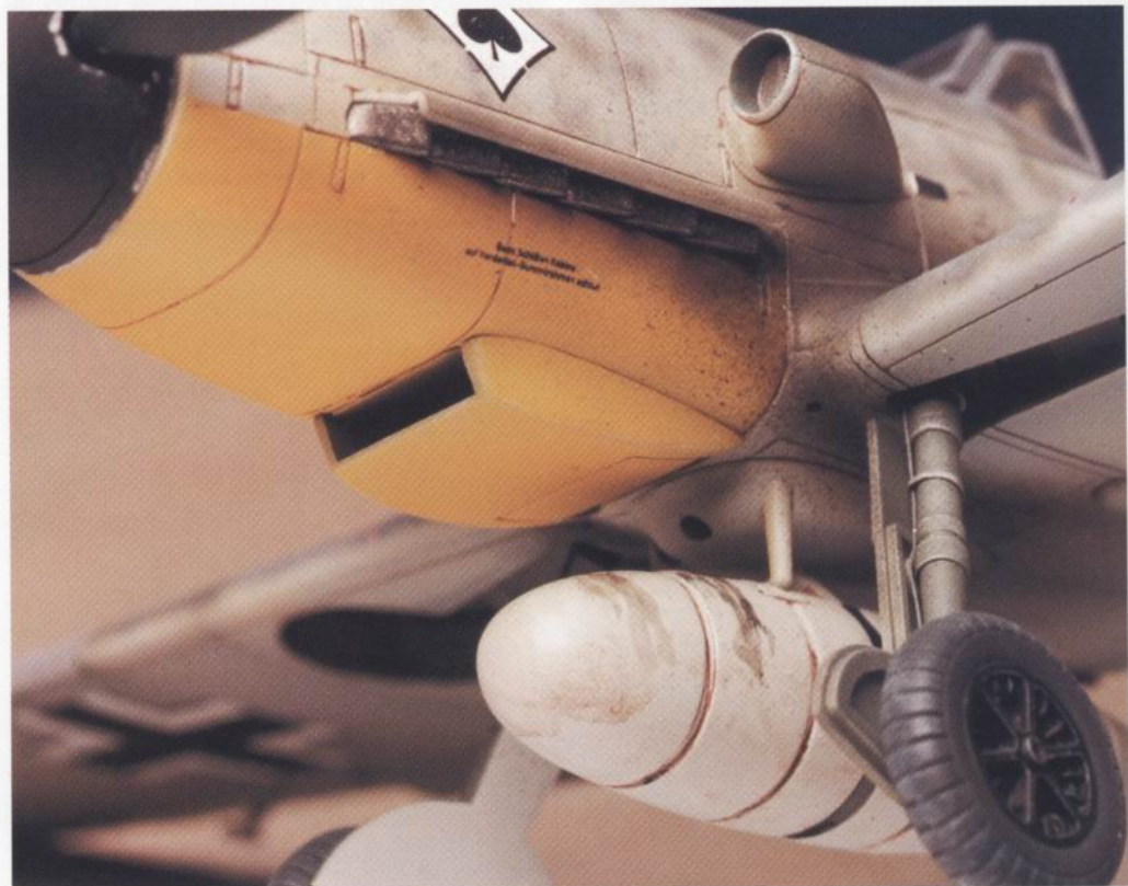
RIGHT The oil drips look effective on the centre-line tank of this Bf 109F-4. Note, too, the replacement wire-mesh grille in the air intake.
