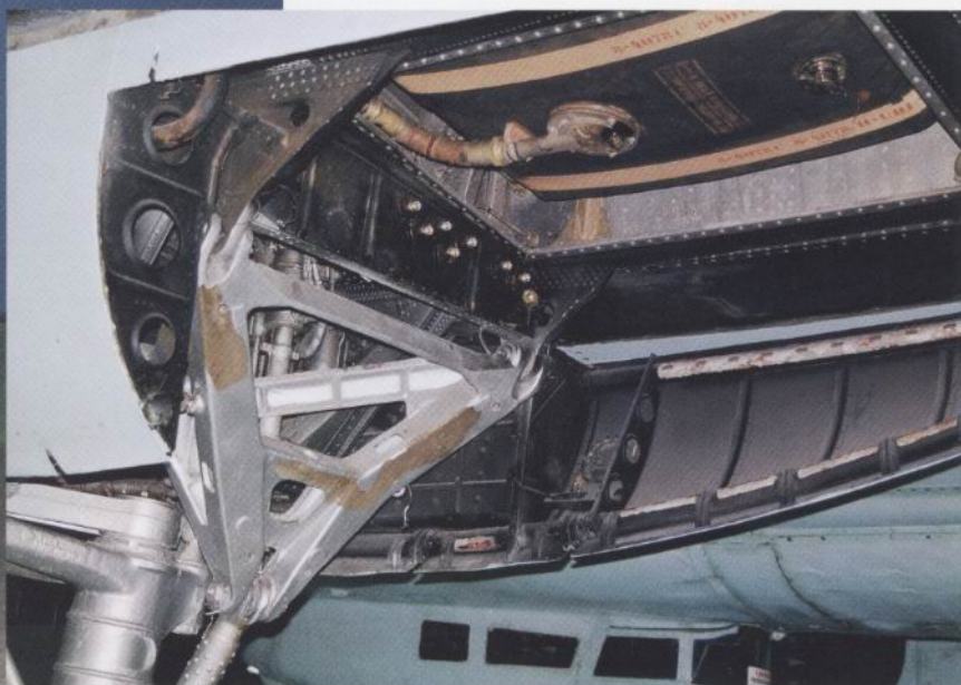
ABOVE The forward end of the Ju 88R-1's left wheel well.
