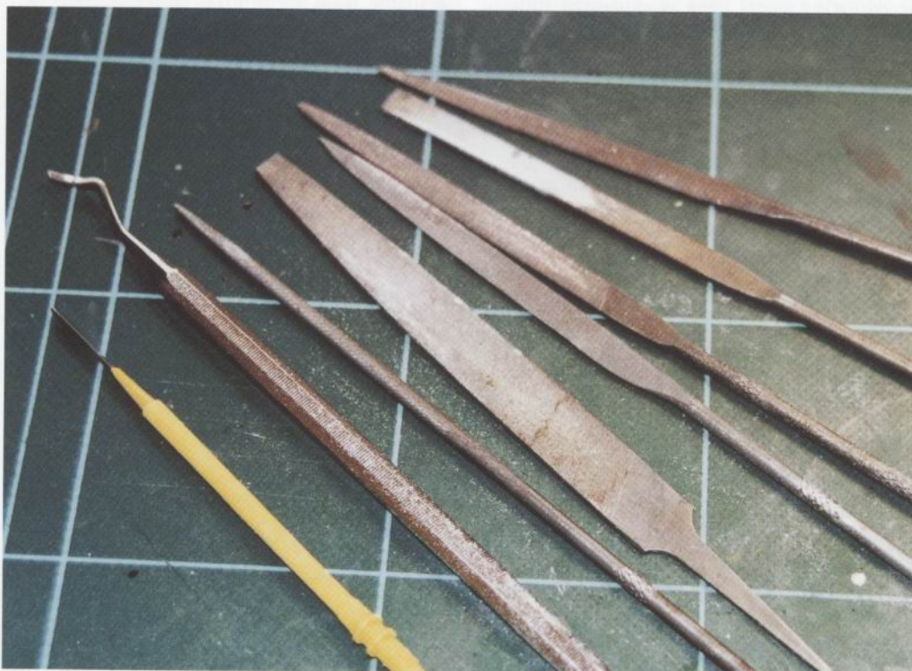
LEFT A selection of thin files, or rat-tail files as they are popularly called.
