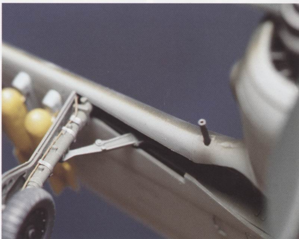
RIGHT The replacement gun barrel of this Fw 190 was made from fine brass tubing.
