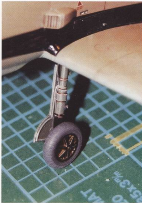
FAR LEFT The undercarriage leg of a Bf 109E-4 – note the hydraulic line that runs down the inside of the leg.
