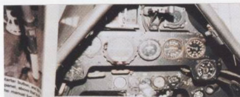
(Above) The upper and lower instrument panels are surrounded by a leather cushioned combing. On the upper left, just under the combing, are the ammunition counters (which are missing) and to the right of the counters is the Revolver 19 gun sight (not installed) mount. To the right of the mount is the AFN 2 housing indicator used for instrument approaches. (Author: Ryle)
