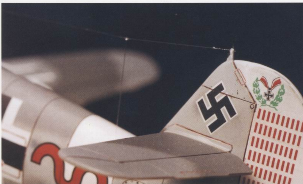
LEFT The aerial wire attached to the Bf 109G-6 fin-top mast.
