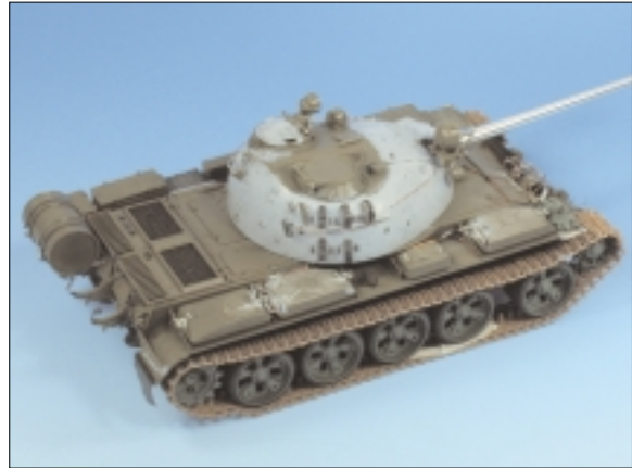
Overall rear RHS view of the built model. Note the gray surface of the turret; Gunze Sangyo Mr. Surfacer has been used to create a subtle cast effect.
