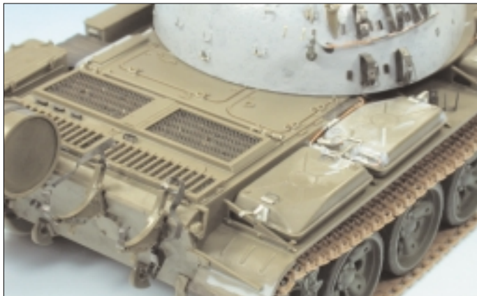
This image shows the rear plate in detail. Note the heavily damaged fuel cell straps, below which are the mounts for the unditching beam.
