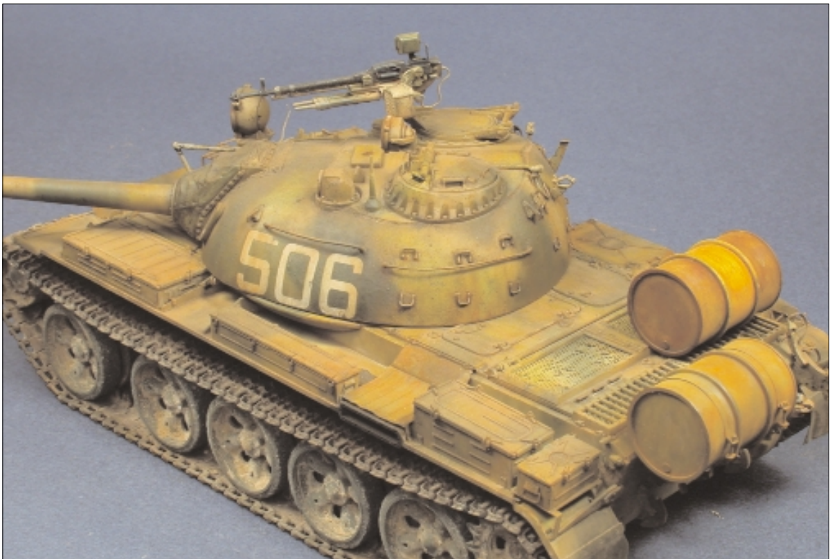
ABOVE Rear RHS view from a lower angle. The rear mudflaps were damaged using pliers, painted black and then dusted up with pastels.
