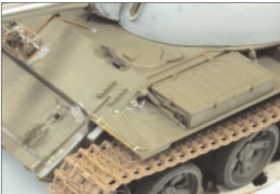
The front LHS area. Note the weld seam going across the nose of the T-55. This was made using Tamiya putty and masking tape. Note the photo etched driver's periscope guards from the Eduard photo etch set.
