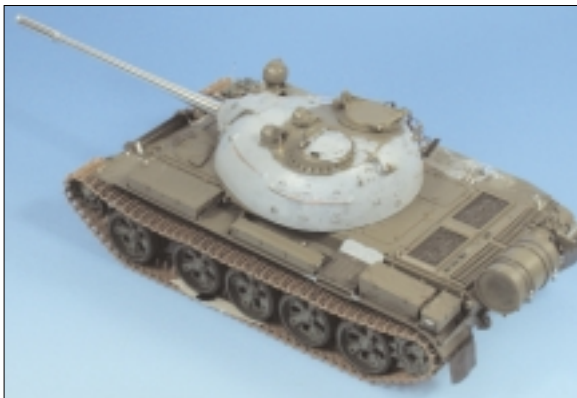
Overall rear LHS view. Mr. Surfacer has also been used to create a cast texture on the exhaust shield mount area.
