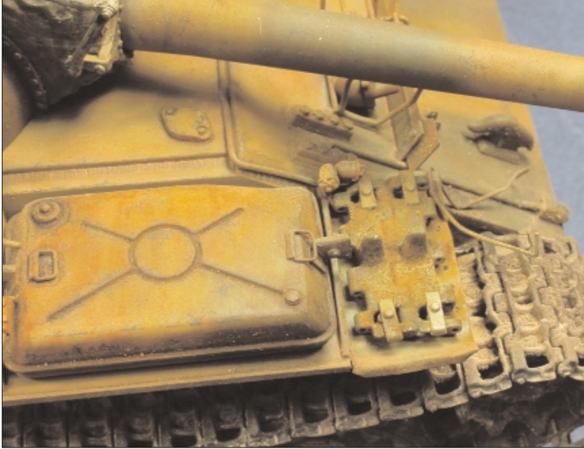
A detailed view of the front fuel cell and spare track area.
