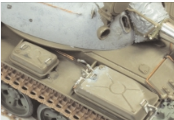
More details of the front fuel cells. Note that the fuel cells are all interconnected via a network of tubing. The tubing runs under the turret race extension. The smaller auxiliary cell features scratchbuilt handles and photo etch mounts from the Eduard set.
