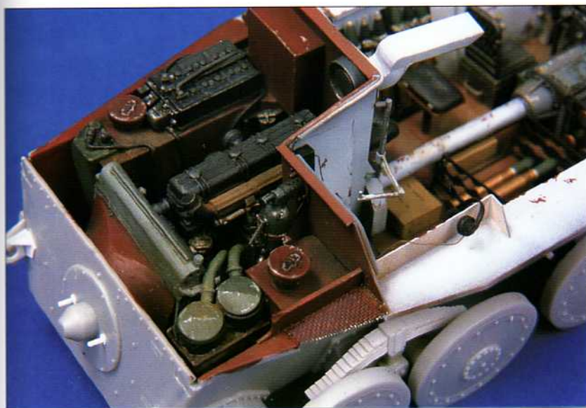
The metallic wear and tear to the engine compartment was added with a silver pencil. To the right of the starboard fuel tank is the mesh screen for one of the air intakes. The other would have been on the left side, hidden by the battery on the port fuel tank.
