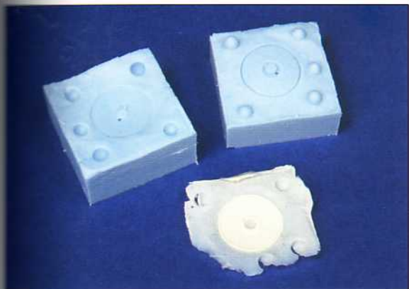
The kit's idler wheel had the holes filled with styrene, and castings were made from RTV rubber moulds and resin.
