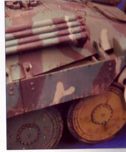
The individual ribs were first positioned using contact cement, then fixed permanently with cyanoacrylate.
