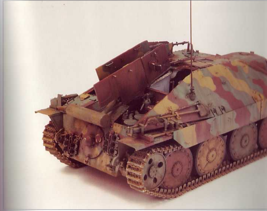
ABOVE The engine hatch on the right side was enlarged to gain access to the air filters. The small coolant hatch was welded closed, and the rear panel cut and welded to the engine hatch itself.
