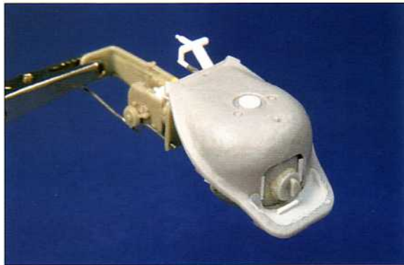
Putty was added to the sunken chin of the Kugellafette , and the stops for the gun cemented into place.
