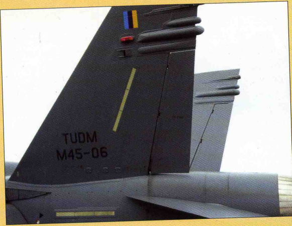
Nice picture of the left fin, slime lights and smart three-colour national insignia. (Jason Cheah)
