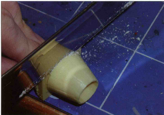
A decent modeller's razor saw is vital for accurate cutting, especially when trying to remove the resin block from finely detailed accessories (as shown here).
