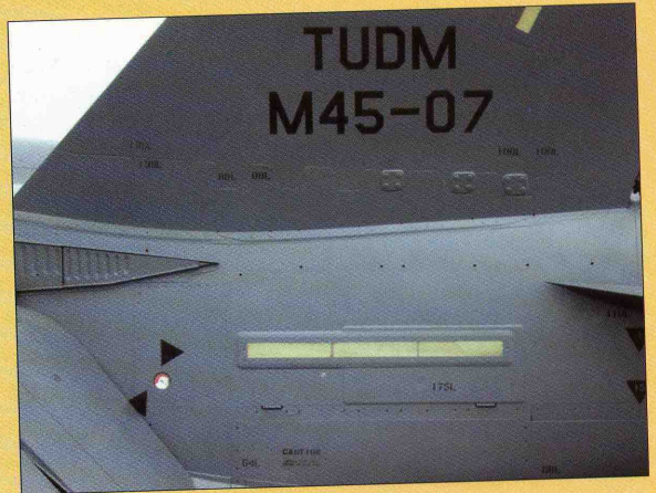
Close up of 07 – note the stencil data and colour of the slime lights. (Jason Cheah)
