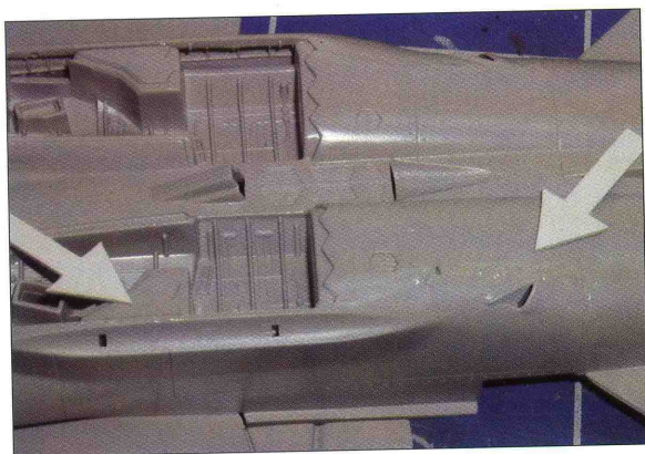
The main assemblies are a poor fit and gaps need to be filled – again superglue works well. Try using an activator or glue accelerator to set the glue immediately.
