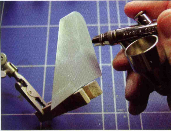
ABOVE AND RIGHT By using your airbrush at a very low setting (c. 6psi) great control is gained when trying to add the touch-up
