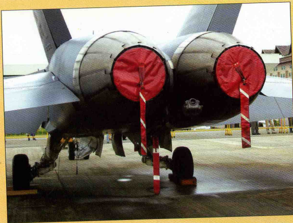
Excellent! I just love the twin FOD cushions that sit inside the jet pipes. Note too the trailing RBF tags – which will be added to the forthcoming F/A-18F build. (Jason Cheah)
