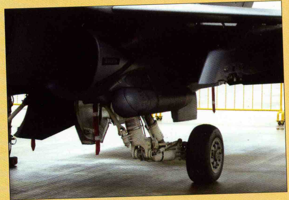
You can just make out the bulges on the leading edges of the main gear doors – aft fairings for the twin chaff-flare dispensers. (Jason Cheah)
