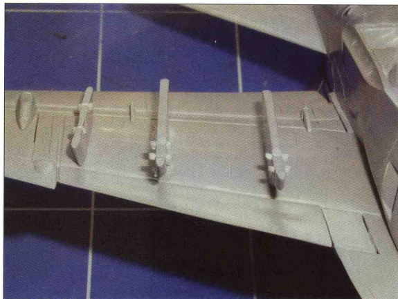
The under-wing pylons on the F/A-18E/F actually deflect outwards from the centreline by 4 degrees. The outer pylon under each wing also tilts away from the centreline by 3.5 degrees – all just visible in this shot.
