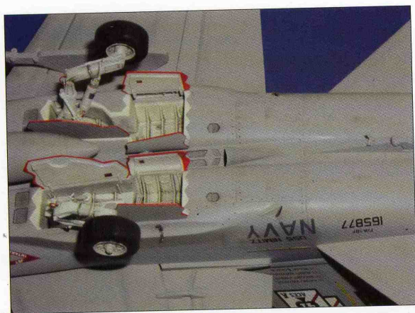
The completed main gear units with additional retraction arms just visible at the front of each leg.
