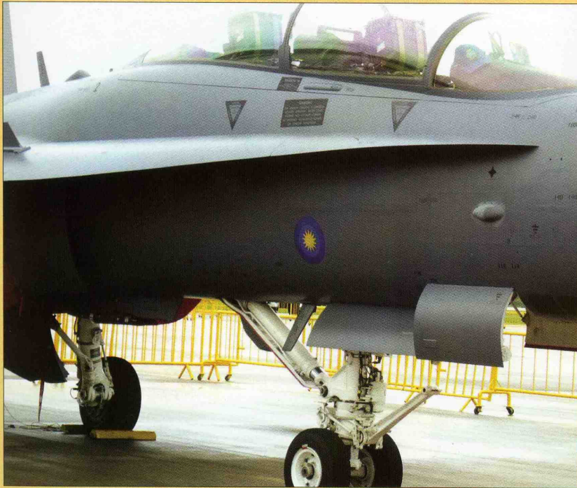
BELOW Left side of the nose. You can just see the RBF tags and engine intake covers. (Jason Cheah)
