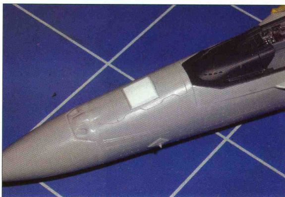
The new 'pizza-box' fairing stuck down with superglue and shaped to fit – made from a thick piece of plastic card.
