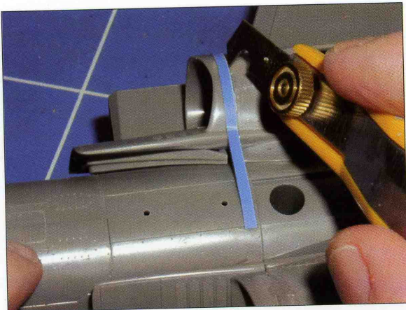
The fit of the intakes left a little to be desired. The gaps were filled with superglue and sanded; then re-scribed, as you can see.
