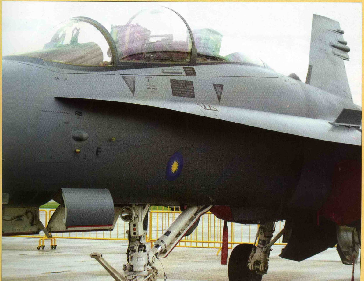
BELOW Left side of the nose. You can just see the RBF tags and engine intake covers. (Jason Cheah)
