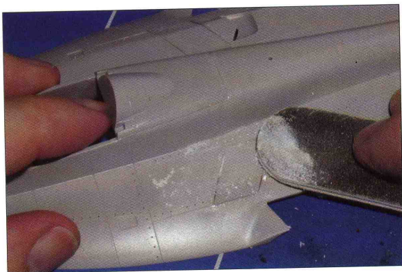
The LEX vents are a very poor fit and are best glued in place, filled and re-scribed. In fact the vents and leading-edge slat spoilers that fit into the wing roots are invariably closed when Super Hornets are parked. The LEX vents are totally flush when closed and so lend themselves to re-scribing.
