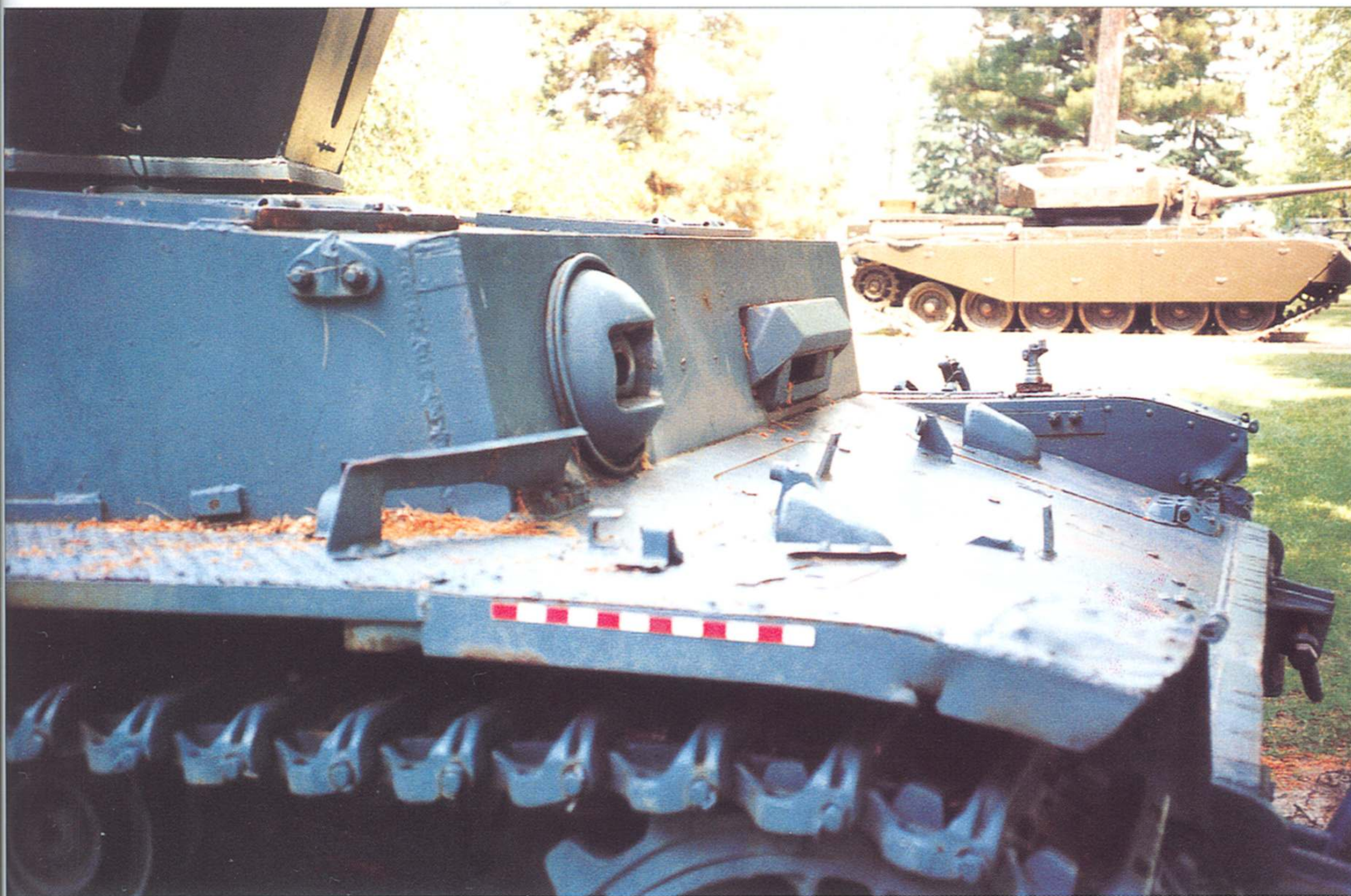
ABOVE The Kugelblende (armoured ball mount for a machine gun) can be seen in the centre of the picture. To the right of this is the driver's vision slot. (Bob Grimster)
