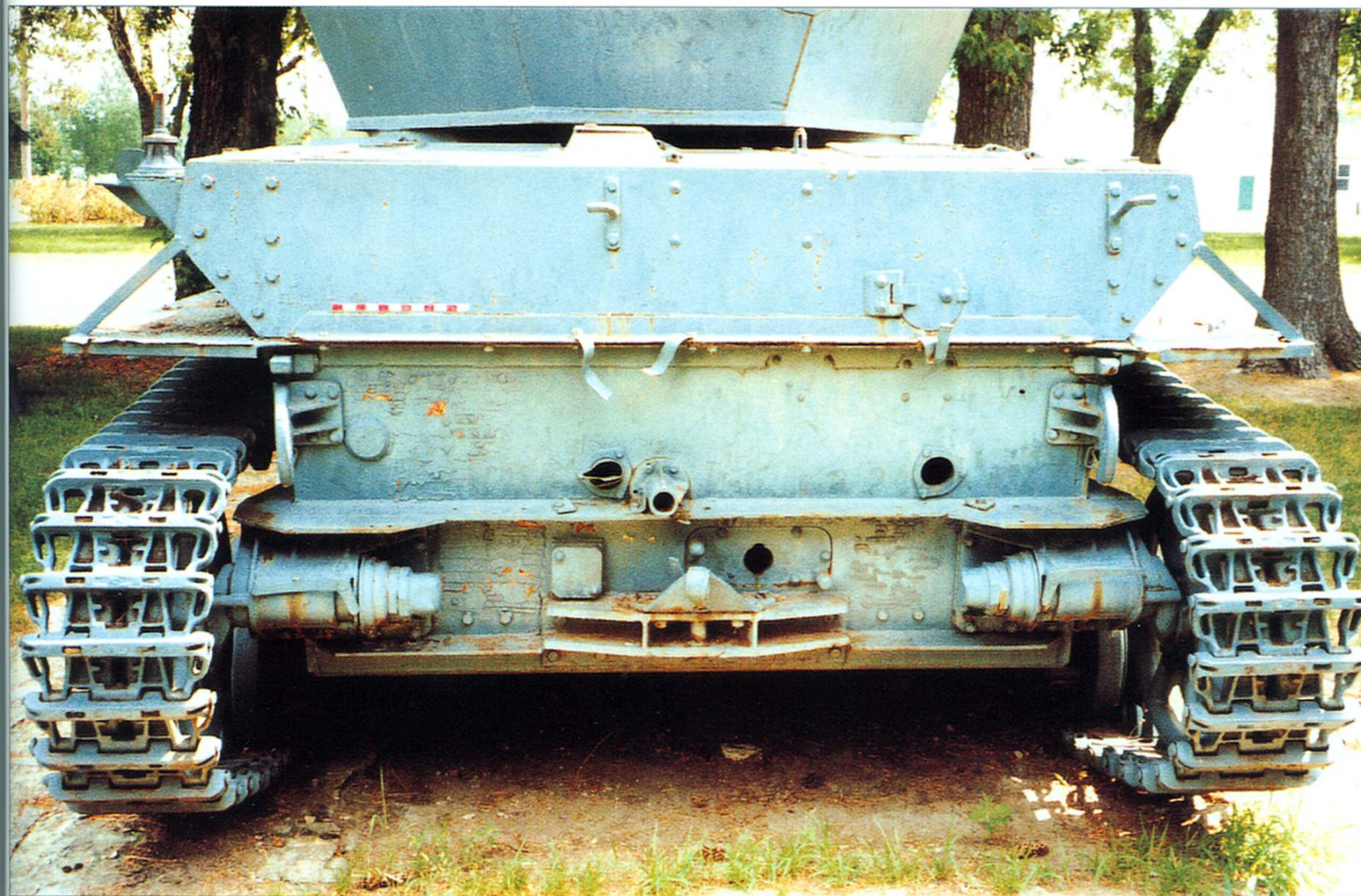
BELOW An overall view of the hull rear showing that the exhaust muffler and mounts are missing. Note the fender supports either side of the hull. It's not clear whether these were wartime modifications or were fitted after the war. (Bob Grimster)
