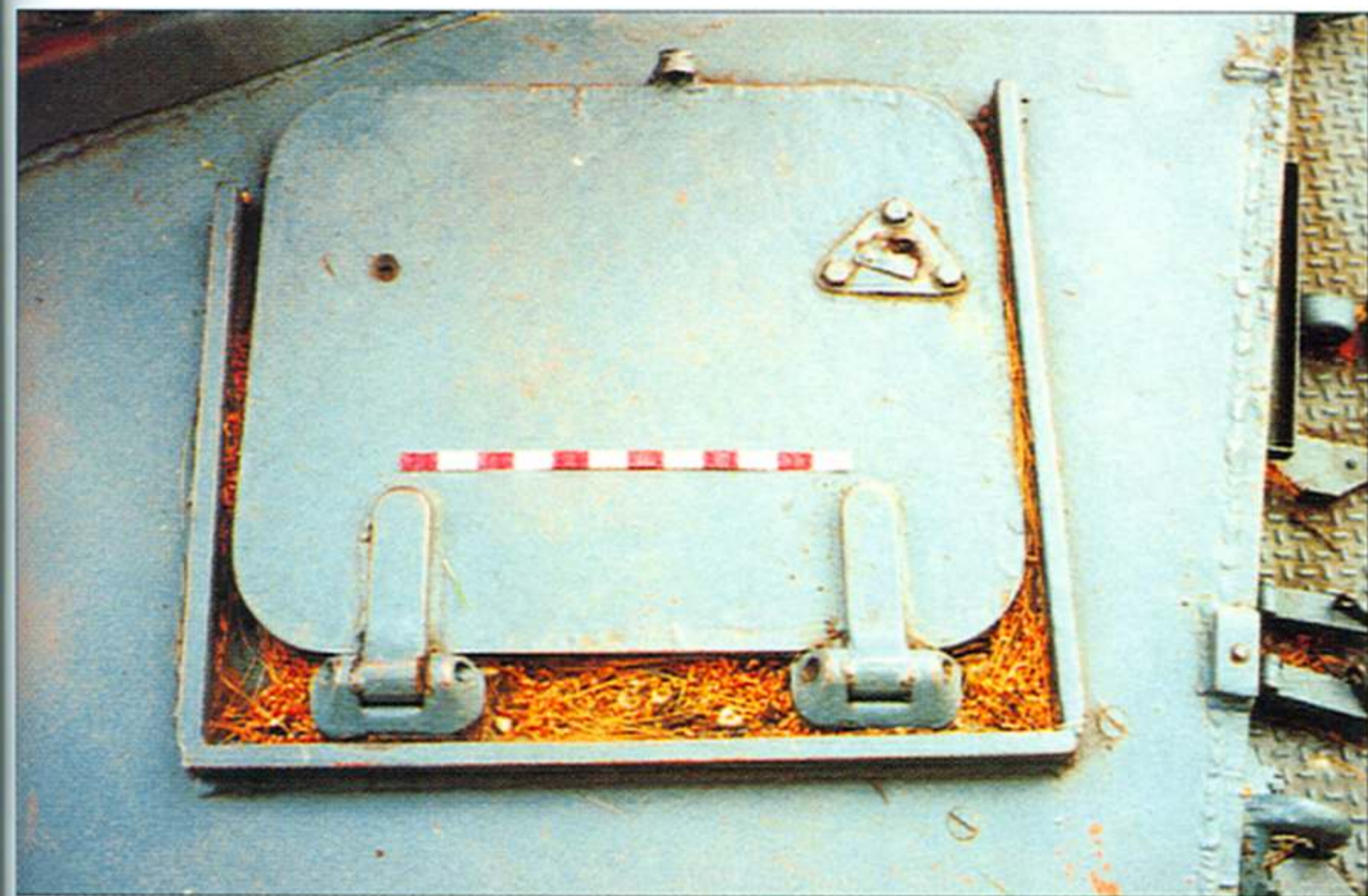
ABOVE The driver's hatch. The shape of the strip guard around the edge is characteristic of later versions of the Panzer IV. (Bob Grimster)
