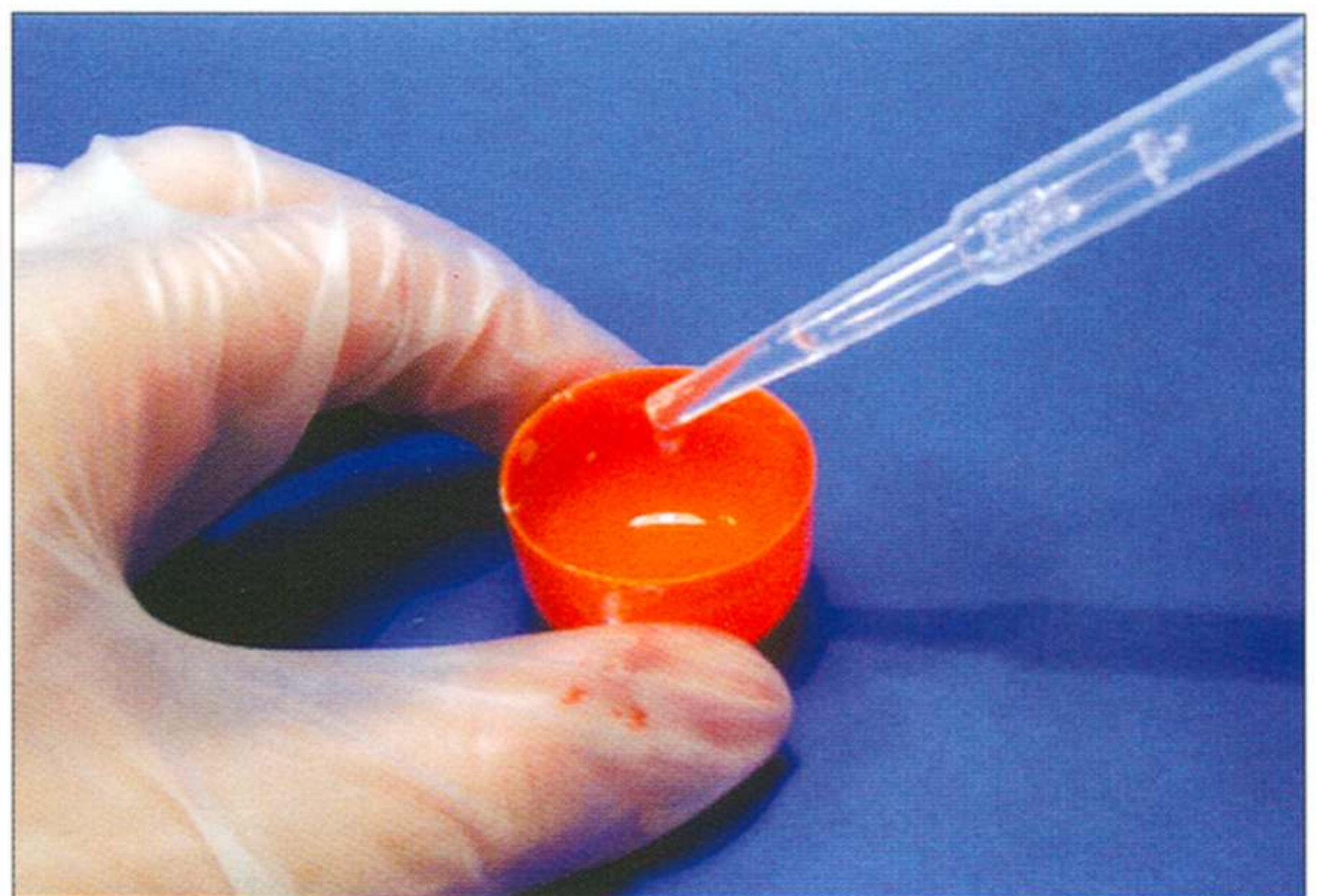
I use Quickcast two-part liquid resin and measure the quantities with small pipettes.
