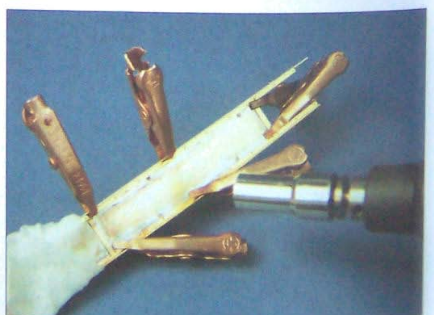
With the tinned sections clamped together, heat was applied with the blowtorch attachment on the soldering tool. To protect previously soldered sections from the heat, wet tissue was wrapped around as a heat sink.
