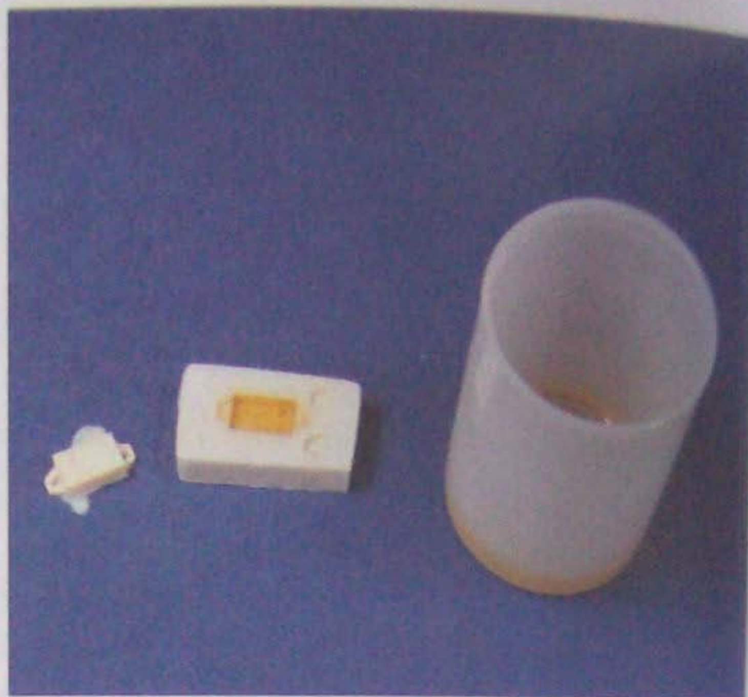
Two-part resin was poured into a mould to make a radio. The amber liquid hardens into the final part seen to the left.
