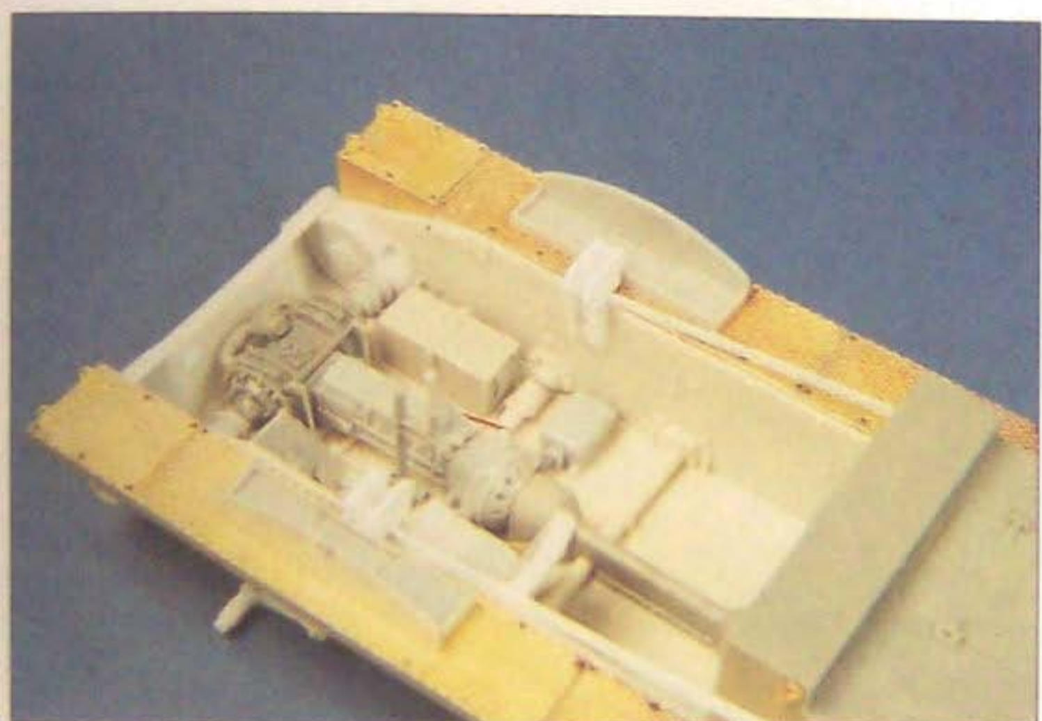
Bracing for the gun sloped downwards from the rear gun support and ran forward to the sIG33 wheel mounts. The brace attachment to the mounts was speculative.
