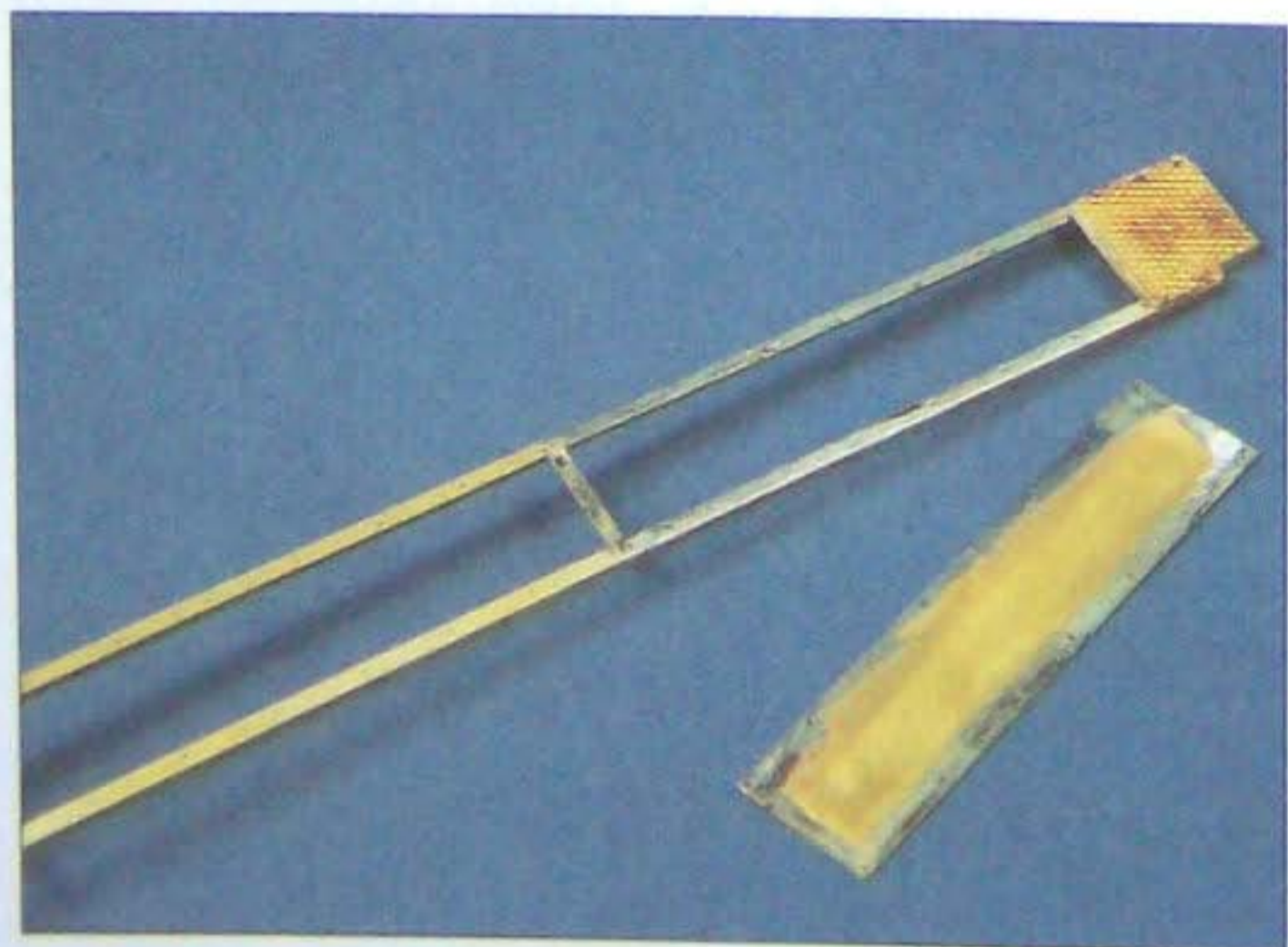
Aber's PzKpfw I fenders were 'tinned' to add the sections of tread plate to the frames.
