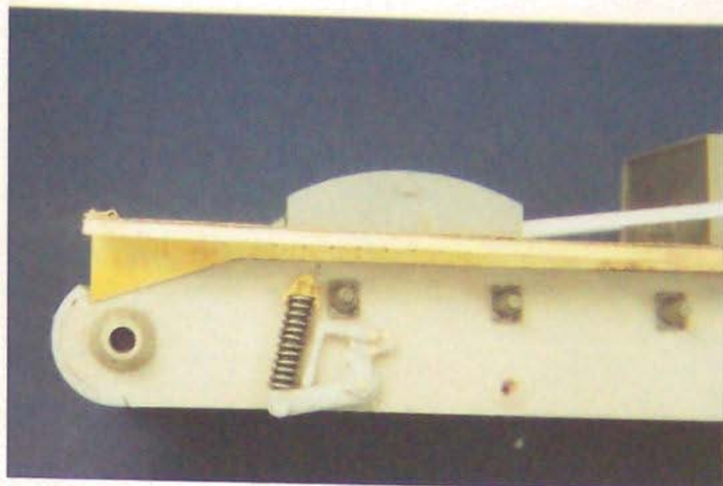
A spring was constructed from solder wire, and the axle for the roadwheel was positioned to align with the base of the hull.
