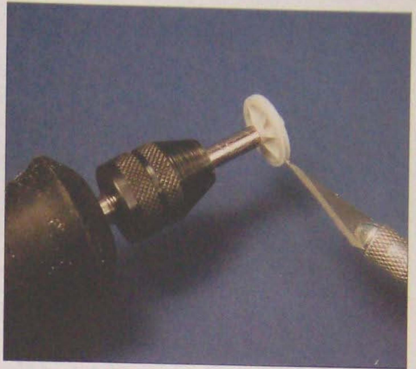
A Dremel motor tool is a versatile aid in forming parts. Care must be exercised when using this tool, and safety glasses are a must.
