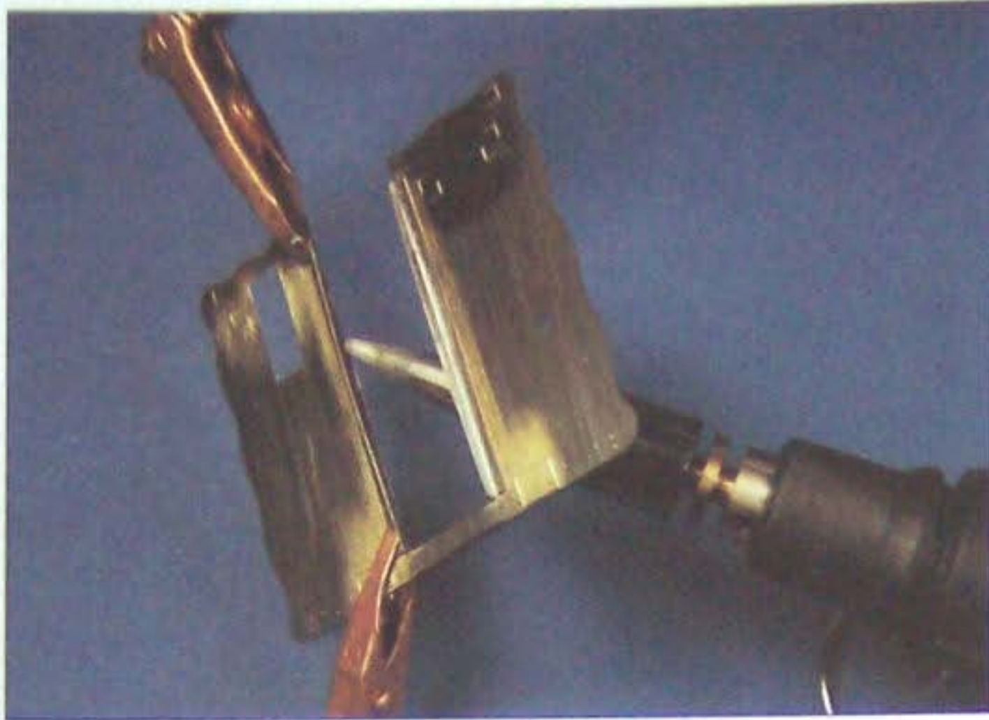
After clamping the parts together, heat was applied to the joint with the soldering tool to make a bond.
