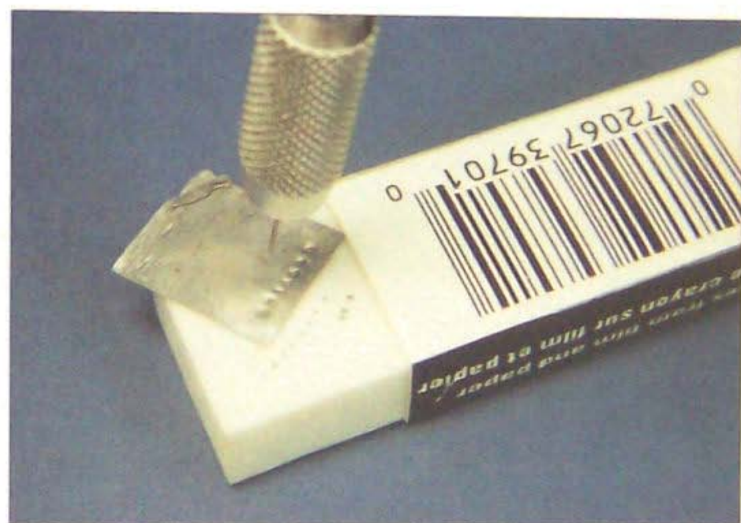
A drill bit was placed backward into a pin vice and pushed into lead sheet supported on a pencil eraser, producing small rivets.
