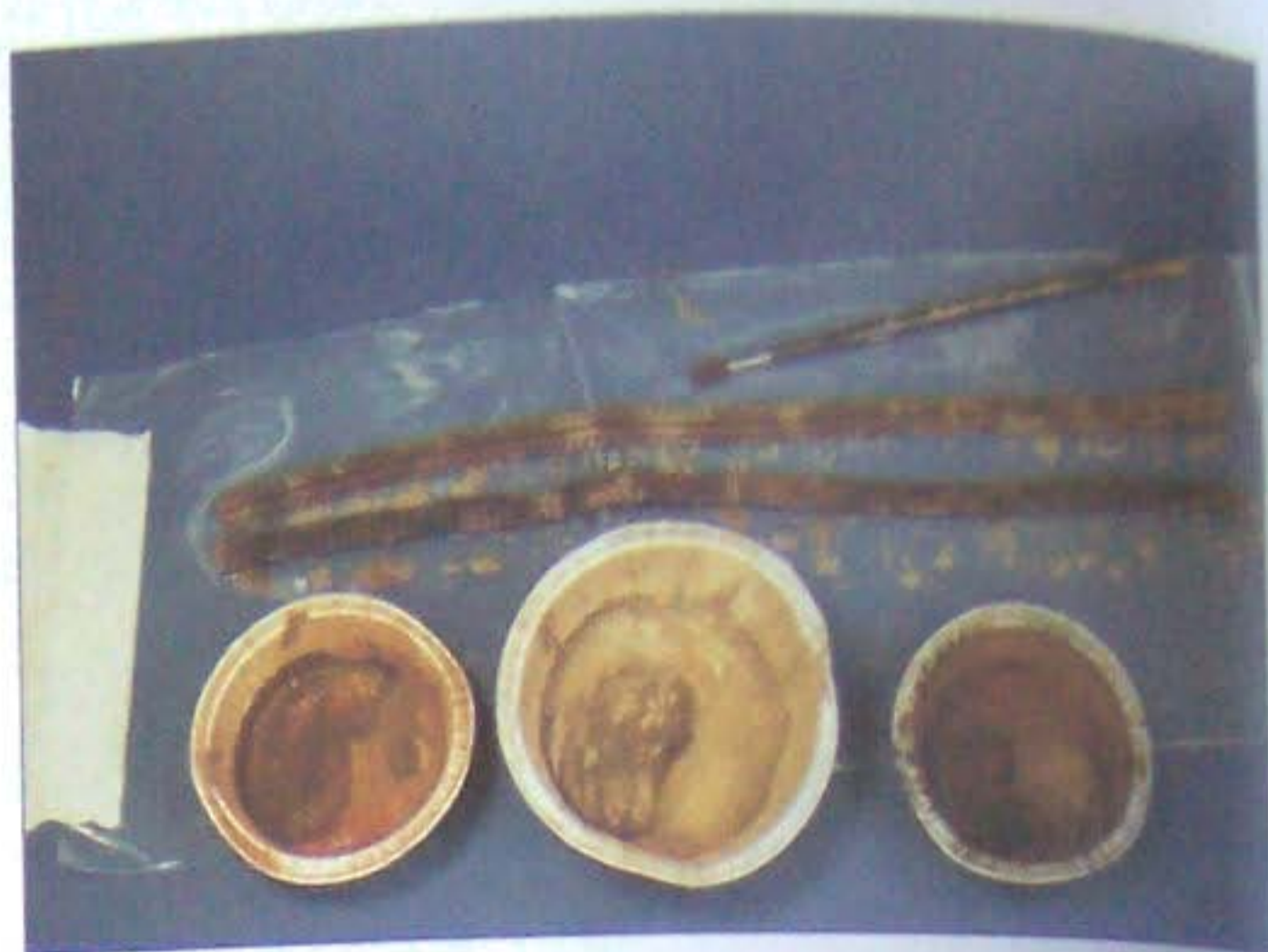
Pastel chalk powders of various colours were thinned with Tamiya's acrylic thinner and randomly daubed onto the track runs. Since this process can be messy, a section of polyethylene served as a base.
