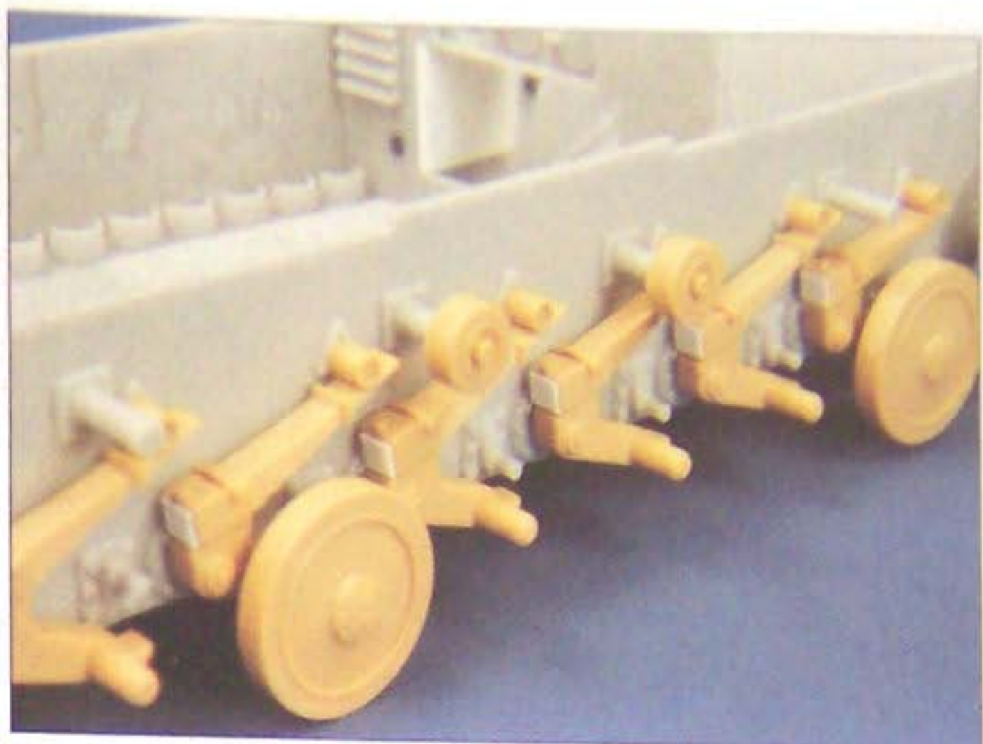
The suspension arms were detailed with squares of scribed styrene to represent the ends of the leaf-spring elements.
