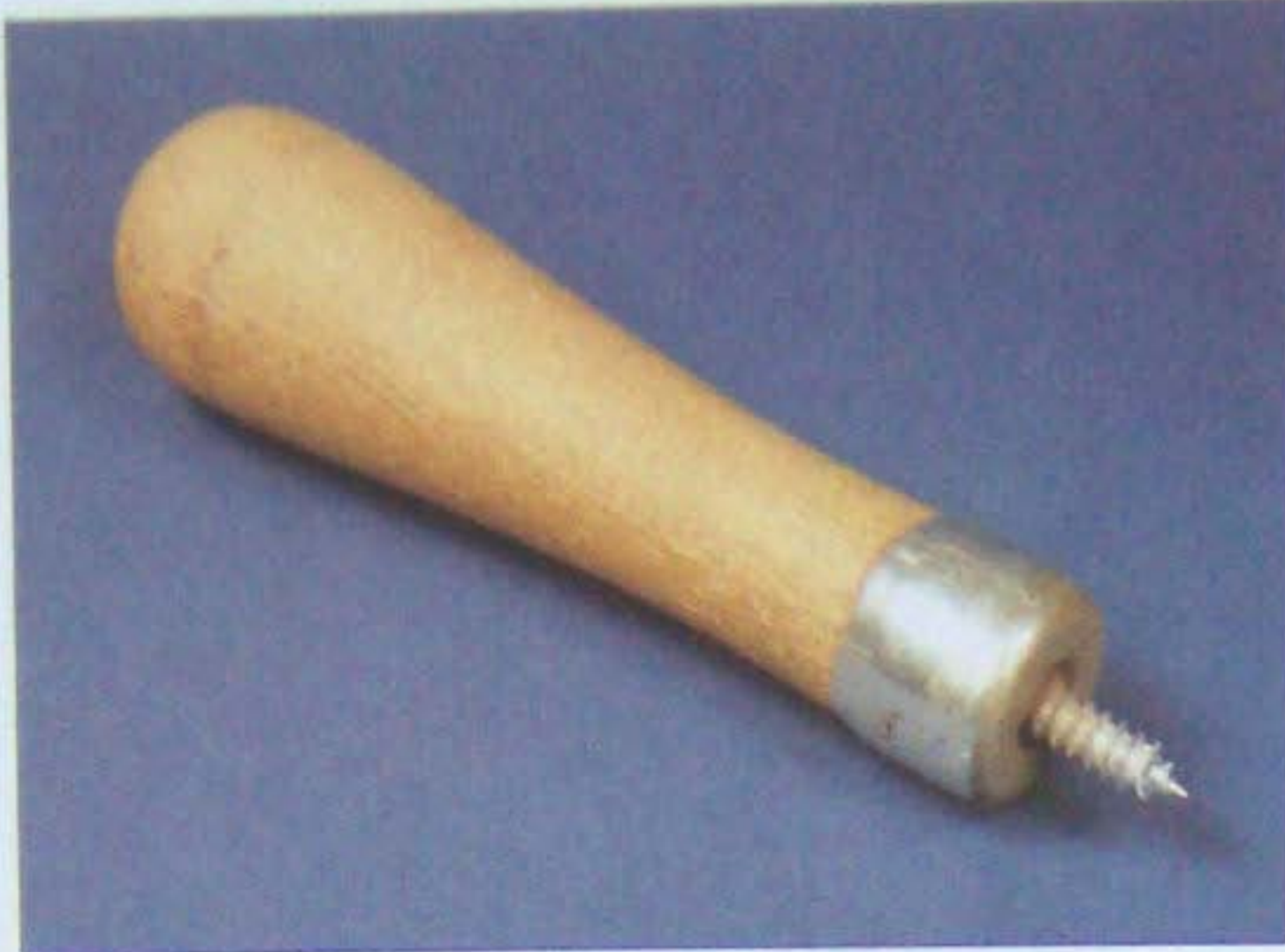
To hold the model while painting, a homemade tool was fashioned by gluing a wood screw into a file handle. The tool was then screwed into a pre-drilled hole in the bottom of the model.
