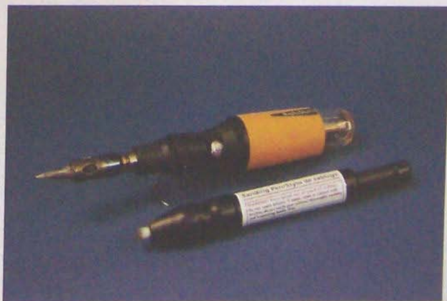
A butane soldering tool was purchased from a local electronics supply shop. The glass filament brush is for cleaning etched-brass details before soldering.
