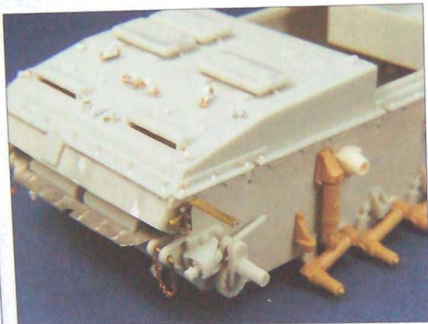
The rear fender supports were bent from 1/16 in. brass channel. The tow cable mounting hardware was scratch-built from soft metal, styrene and ModelKasten wing nuts.
