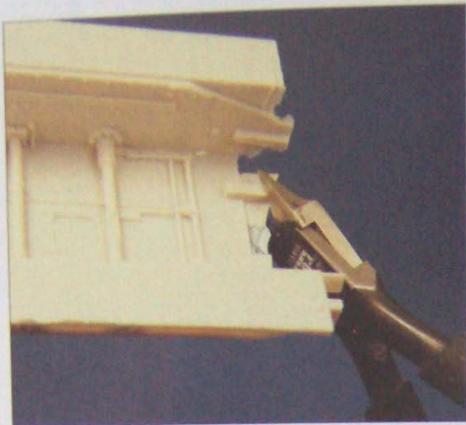
A sharp pair of side cutters is ideal for trimming the pour-plugs from resin castings, in this case the hull from the Bison I conversion kit.
