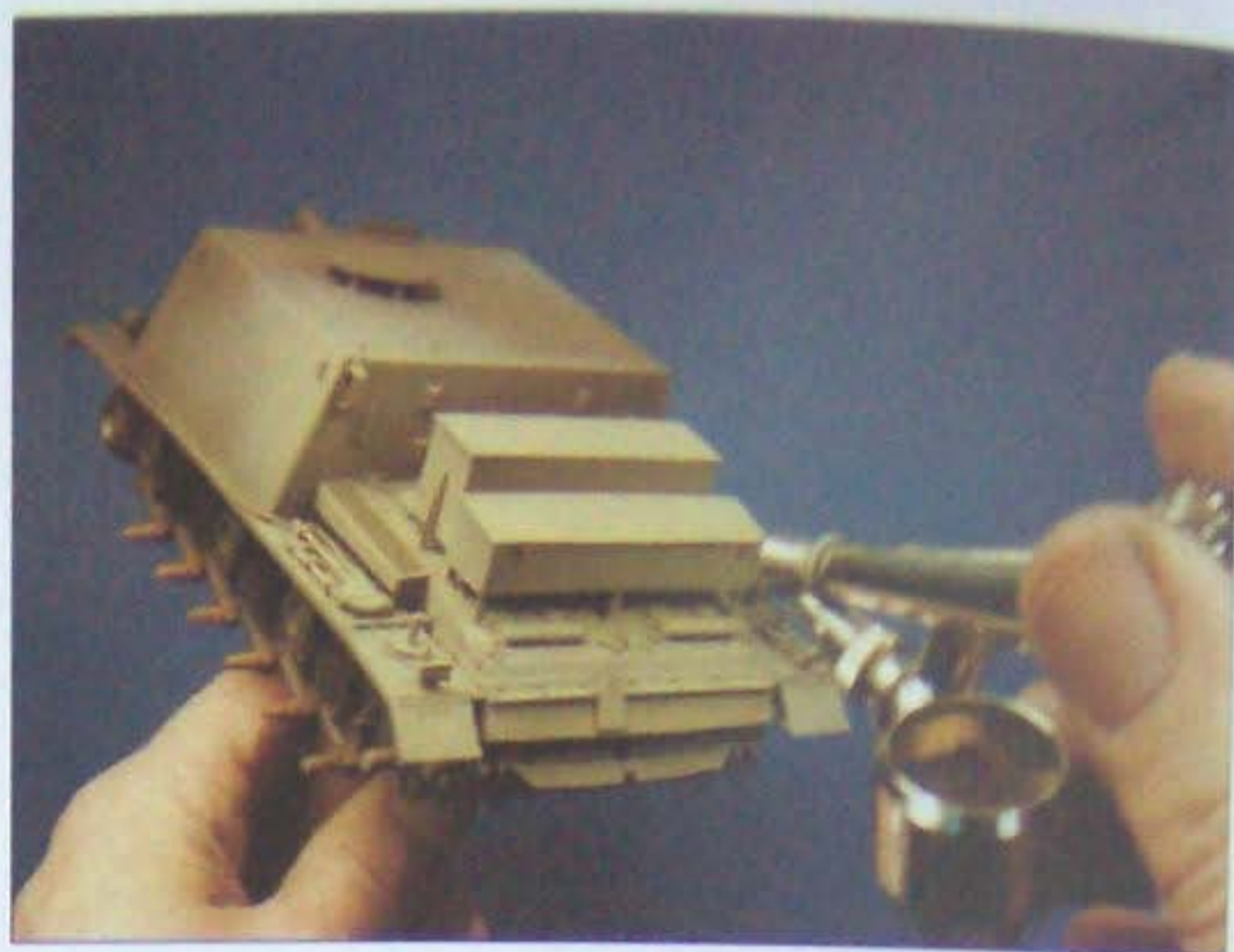
After priming with dark brown Floquil lacquer, a base coat of acrylic three-colour camouflage was airbrushed onto the model.
