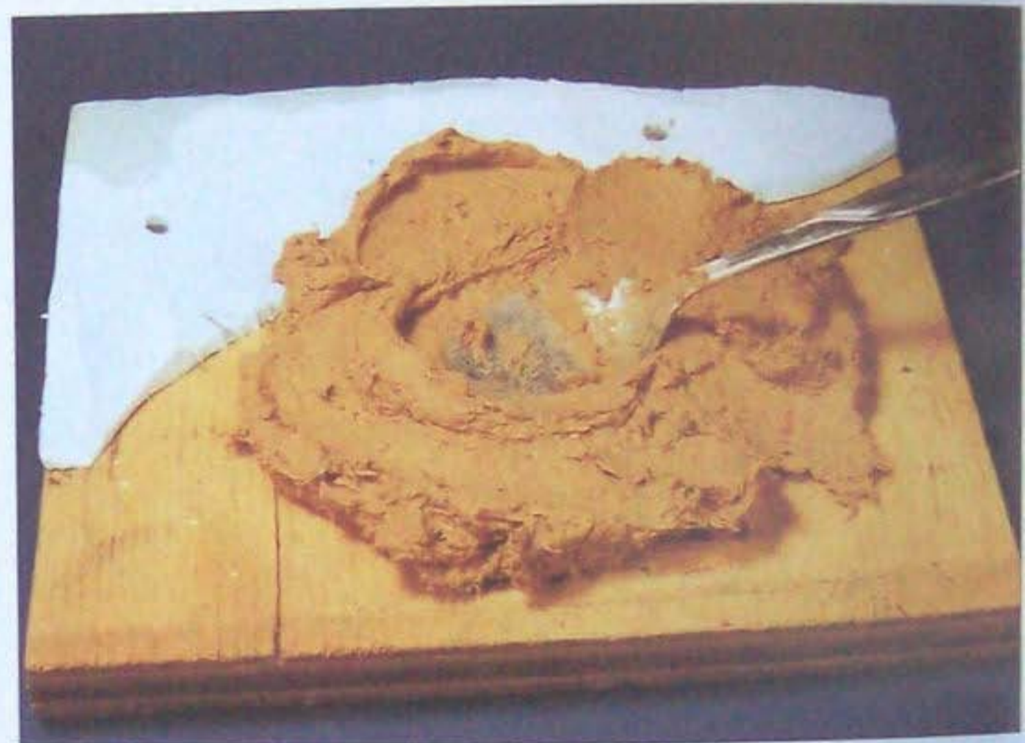
After screwing the polystyrene down, a mixture of Celluclay, Hydrostone plaster, white glue, paint pigment and water was spread onto the base.
