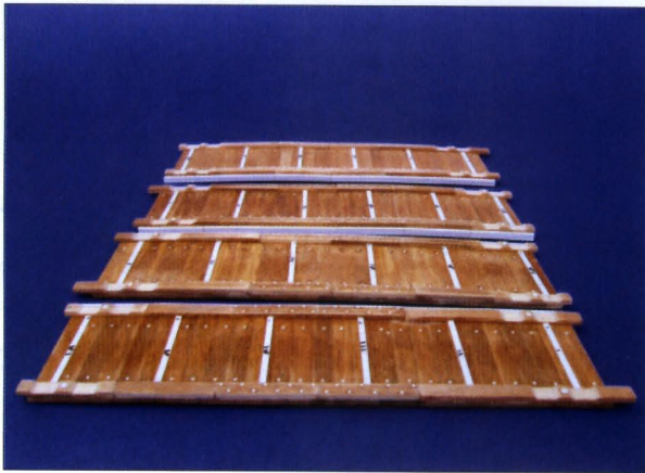
The decking was fashioned from bass wood cut to size and length, and rivets were added using a punch and die set.
