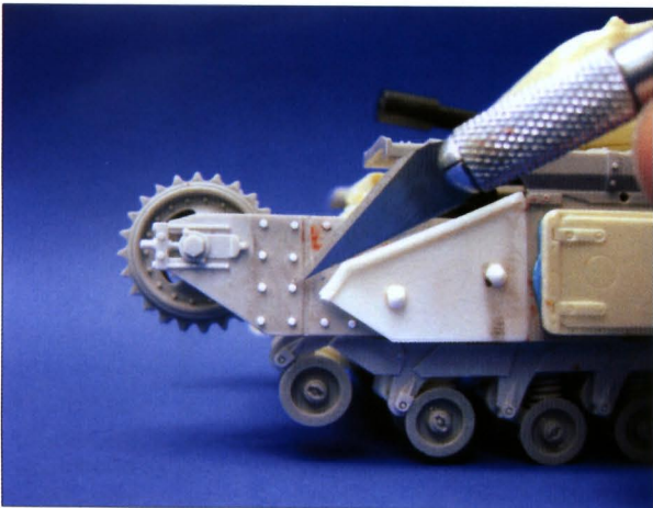
Adding rivets made using a punch and die set.
