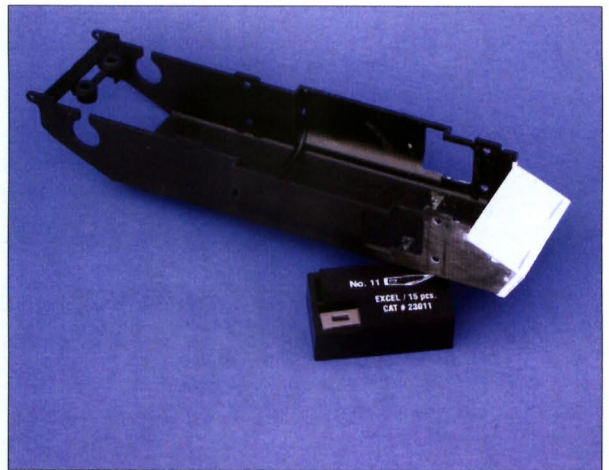
The front nose of the Tamiya kit was discarded and a new one was built using sheet styrene.
