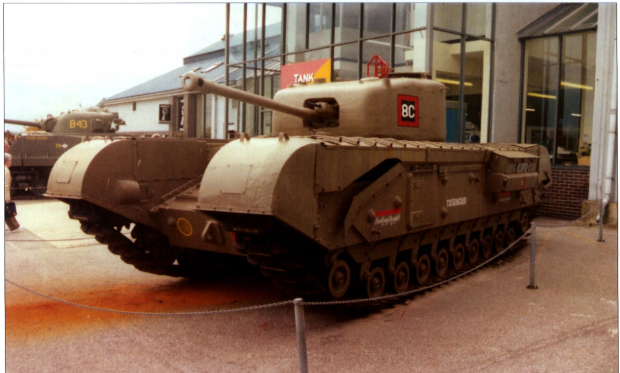
BELOW A Mk.I or II upgunned to a Mk.IV, with a mounted 75mm gun and Mk.VII suspension, located at Bovington, UK. (Chris Shillitos)
