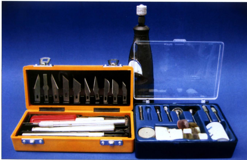
LEFT AND BELOW LEFT An assortment of blades and Dremel bits, an X-Acto knife, a compass (for measuring spaces between rivets), a metal file, and tweezers and nail clippers for snipping photo-etch.
