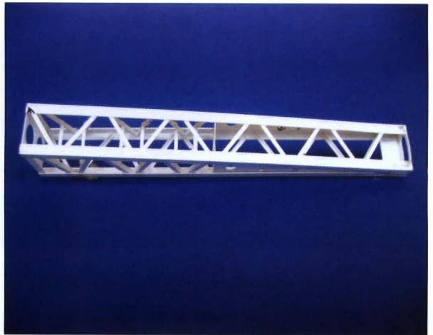
One of the support brackets constructed from Evergreen sheet styrene.
