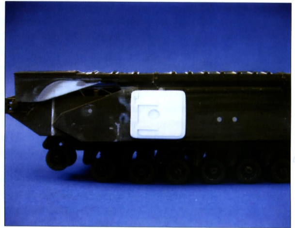
The side escape doors were scratch-built using sheet styrene.
