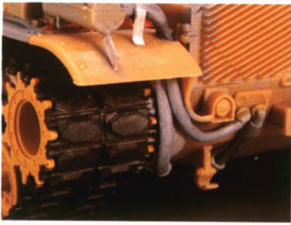
The pipes of the dozer blade's hydraulic system stand out on the rear part of the upper hull.
