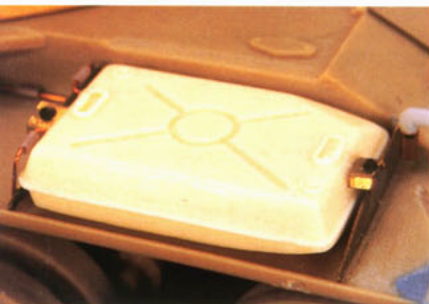
The fuel cans were based on one from the Tamiya T-62 kit. After modification, resin copies were made.
