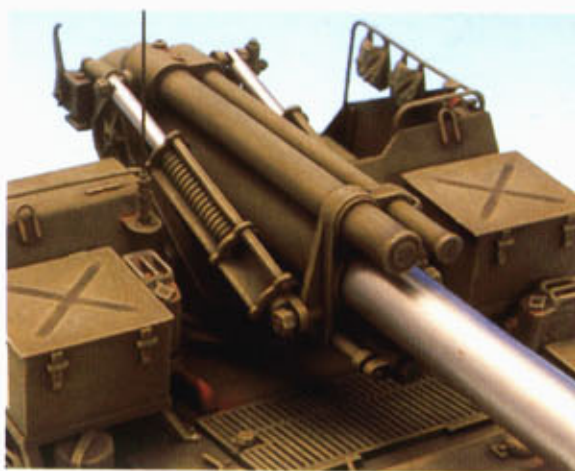
Italeri 155mm howitzer; the top carriage needs to be lowered by 3 mm.
