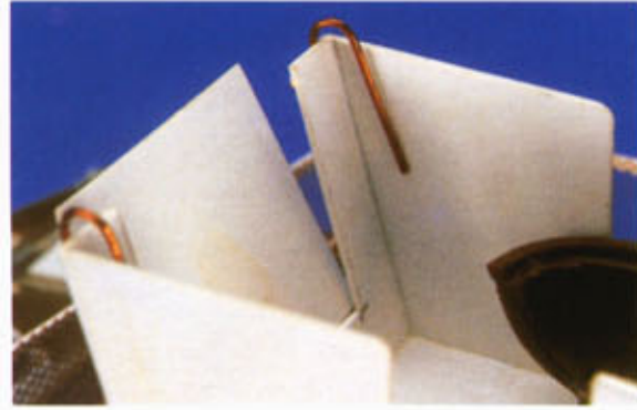
The rear door opens with a device made of copper wire.
