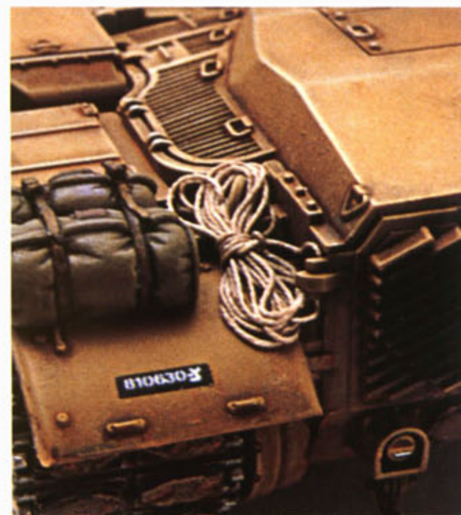
Use putty for curved shapes and resin or plastic for angles.
