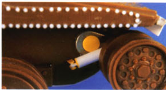
The front wheel has a shock absorber, made of plastic tubing.
