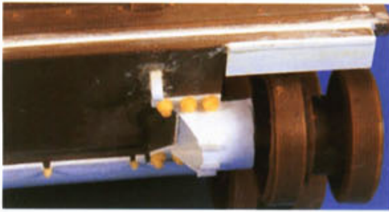
Reconstruction of the front wheel axle protector, made with plastic sheet, rivets and small rods.
