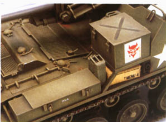
The grids are reconstructed with 0.20 x 0.40mm plastic strips.
