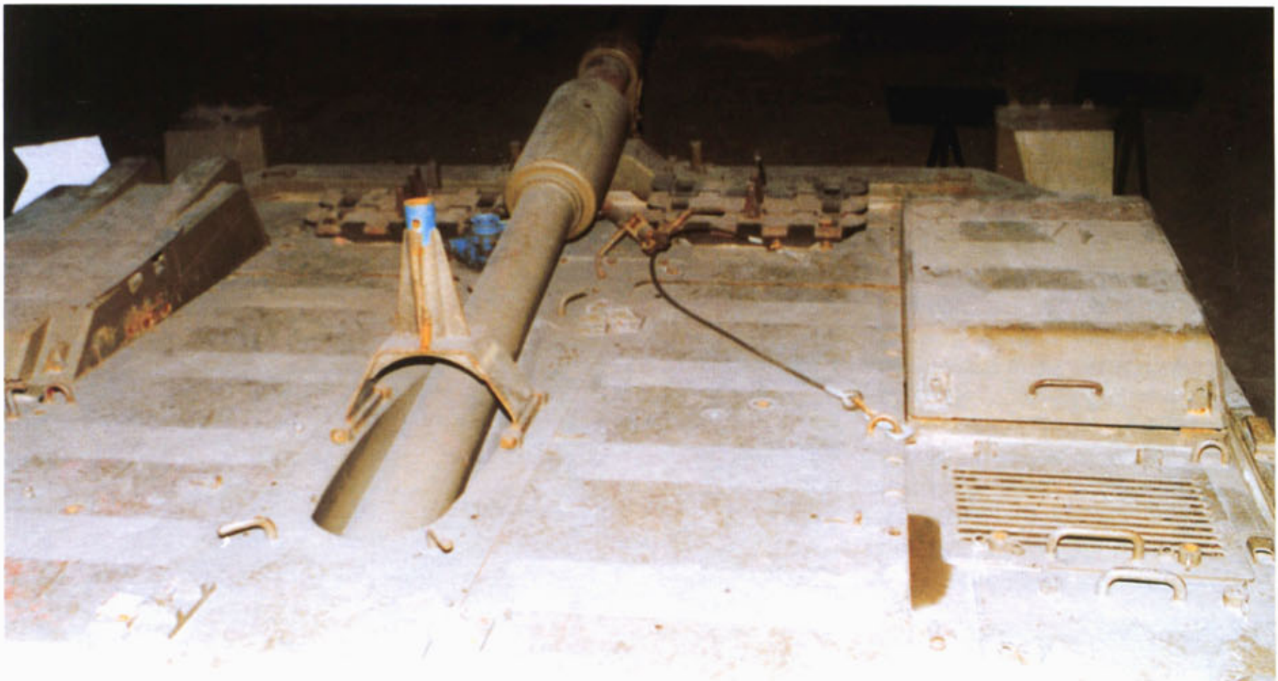
View down the barrel and of the glacis plate: note the non-slip bands.
