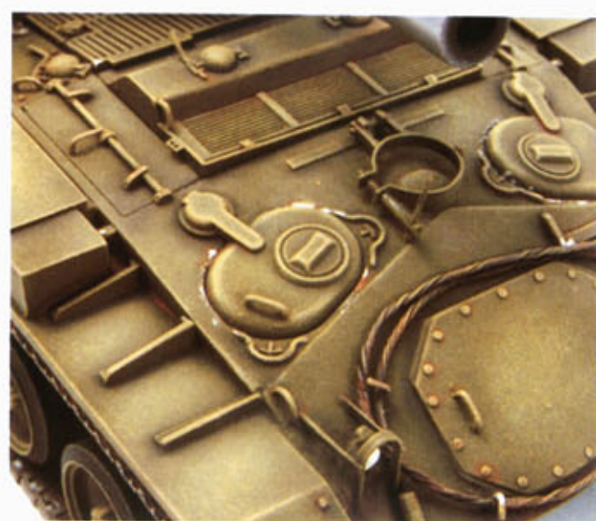
Front reconstructed with the elimination of the machine gun and the addition of a support fixture for the gun.
