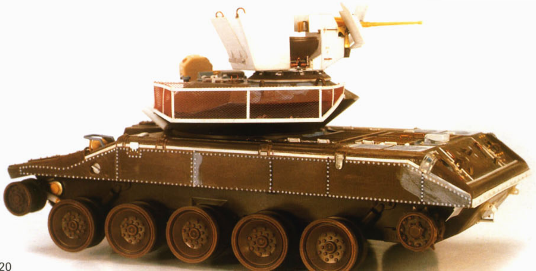
Note the rear carrying basket. The metal grid is imitated with Verlinden synthetic mesh.
