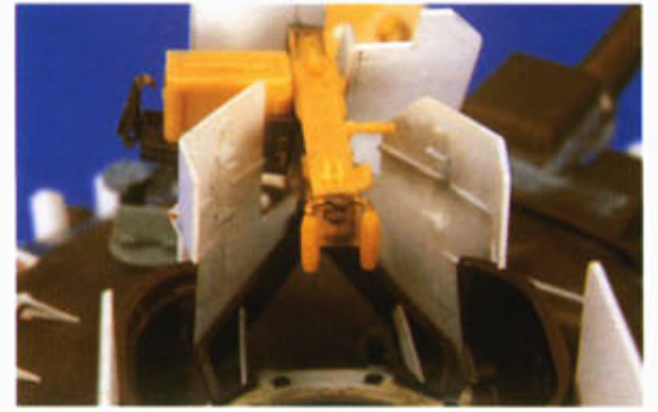
The connectors for the different armour plates were made by cutting plastic strips to length.
