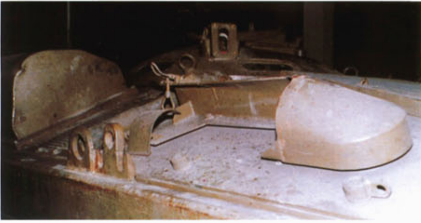
Support for the extinguisher located on the right side.
