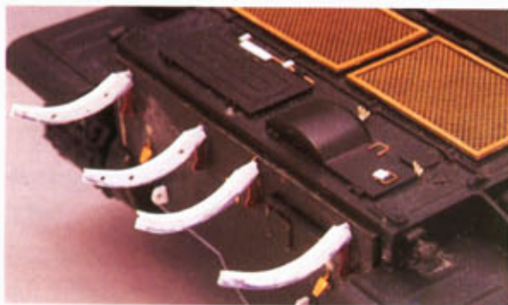
Rear view. Showing the plasticard fixings for the drums and etched-brass ventilation grids.
