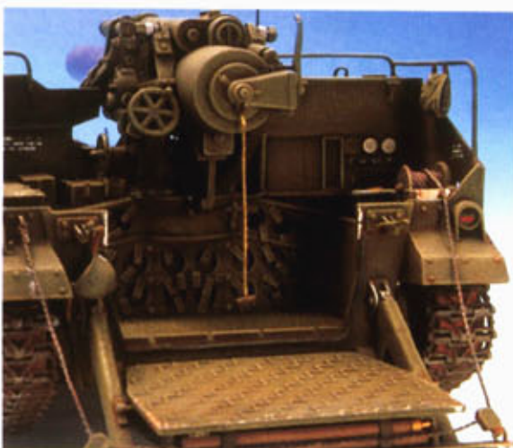
Combat chamber with the compartments for ammunition and their locks.
