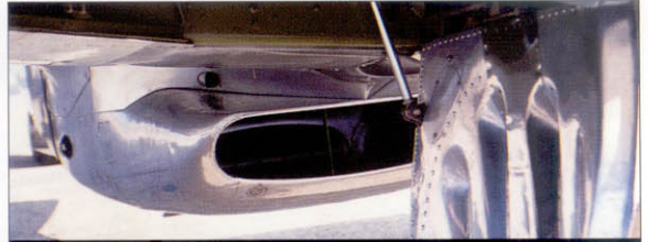
5 Detail of the air manifold and radiator.
