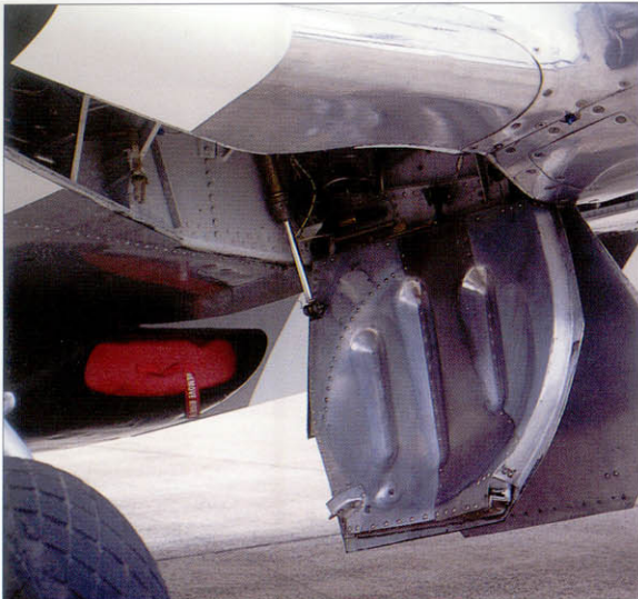
4 Interior of the wheel wells and undercarriage doors.
