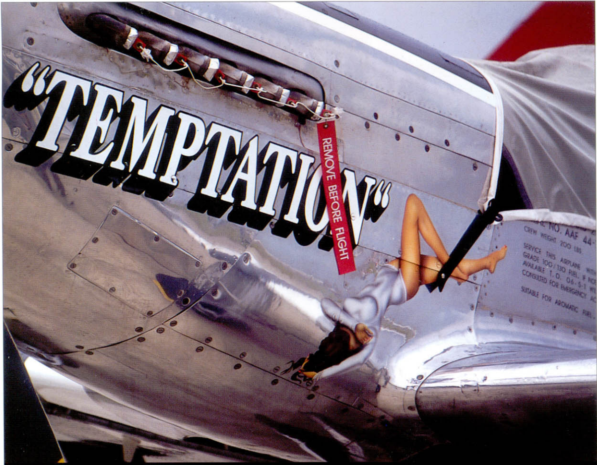
7 Note the dramatic nose art and the shading differences on the engine panels. The exhaust outlets are protected with their individual protective covers.
