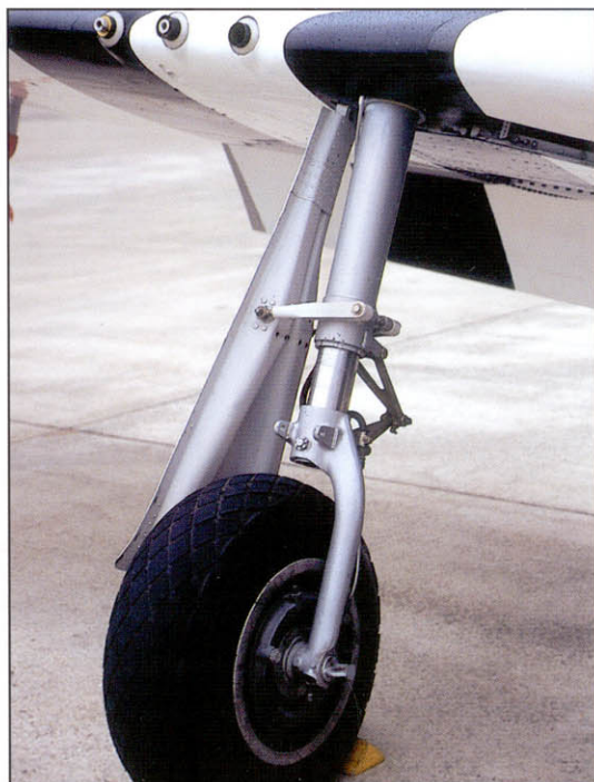
9 Right-side undercarriage. We can also see the muzzles of the three 0.5in machine-guns.
