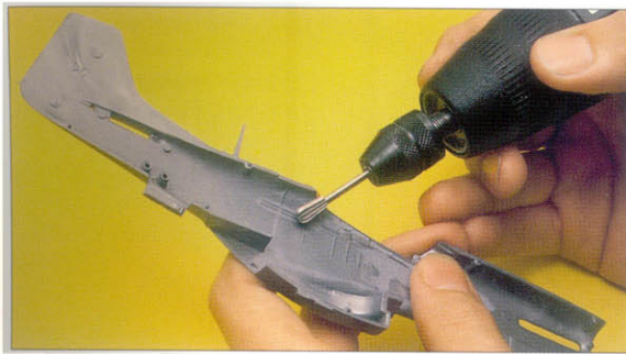
ABOVE Unwanted detail on the cockpit interior was removed with a drill bit.
