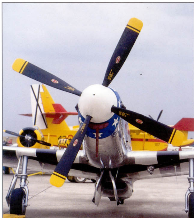
8 Detail of the 'cuffless' type Hamilton Standard propeller fitted to the final Mustangs and commonly seen post-war.
