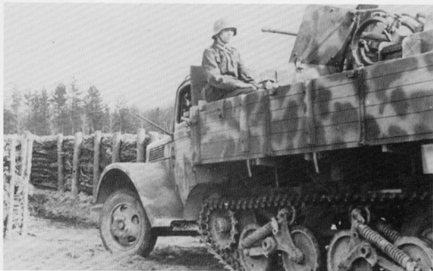
This reference photo for the Maultier conversion shows that relatively few changes to the vehicle are required. Note the extra wood blocks on the sides of the body.
