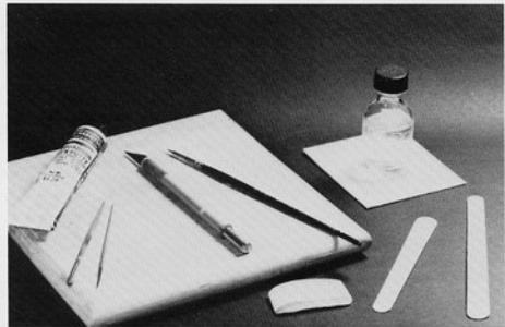
Basic tools and materials for kit assembly. From left: plastic body putty ("green stuff"), needle files, hobby knife, loop of masking tape for small parts, cement brush, liquid cement bottle epoxied to piece of card, and emery boards for sanding.
