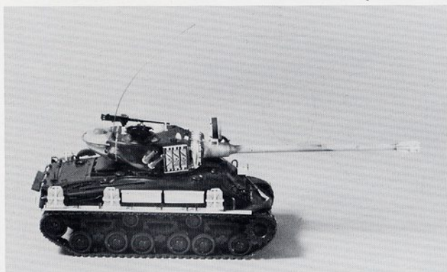
(Left) The completed model before painting and weathering. The new fenders are sheet styrene with Plastruct brackets, the mantlet cover was made from tissue, and the stowage boxes were made of thick Evergreen styrene strip. The searchlight was made by covering an extra road wheel with sheet styrene, then adding a tissue cover over the front. The smoke grenade launchers on the side of the turret are brass tubing, cut in a miter box to ensure accurate square cuts.
