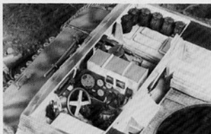
The Tiger I driver's and radio operator's compartments. Note the ammo storage.
