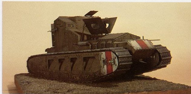
Jim Stephens' superb 1/25 scale WWI Whippet is one of the finest scratchbuilt armor models I've ever seen. The hull is sheet styrene, detailed with hundreds of Sig copper rivets, and the engine louvers are vacuum-formed. The tracks were cast from a sheet styrene pattern. The roof of the crew compartment is removable to show off the interior.
