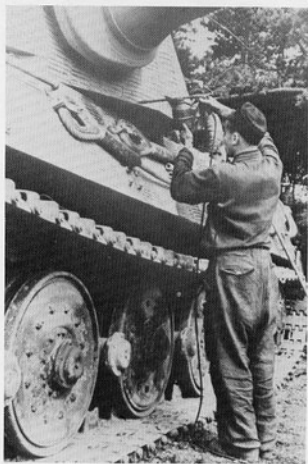
Some WWII German armor crews could paint their tanks by hooking up a spray gun to the vehicle's air compressor.
