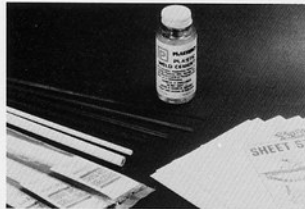
Materials for conversions and scratch-building: Evergreen plastic strips, Plastruct tubing (white), Plastruct structural shapes (dark gray), Plastic Weld (to bond ABS to styrene), and sheet styrene.
