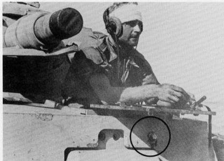
Even shots that do penetrate are not always fatal. This German tank driver seems to have survived a particularly close call with no more than a slight head wound; note the small impact hole in the front armor plate (circled).
