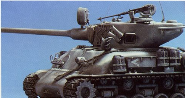
A close-up showing the side stowage, including spare tracks, smoke grenade launchers, and the distinctive Israeli single-handle, black rubber jerry cans.
