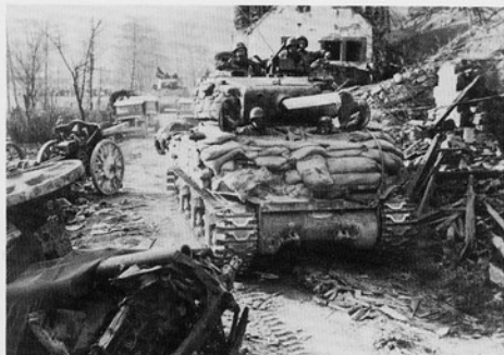
A late-WWII Sherman with heavy sandbag armor in racks on the sides and turret. Note the "grousers," extensions added to widen the tracks to spread the weight of the tank on soft ground.
