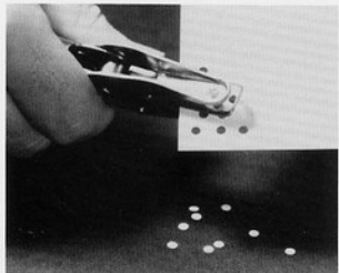
Paper punches come in a variety of sizes and work well for punching neat holes in thin styrene. Both the holes and the round punch-outs are useful.
