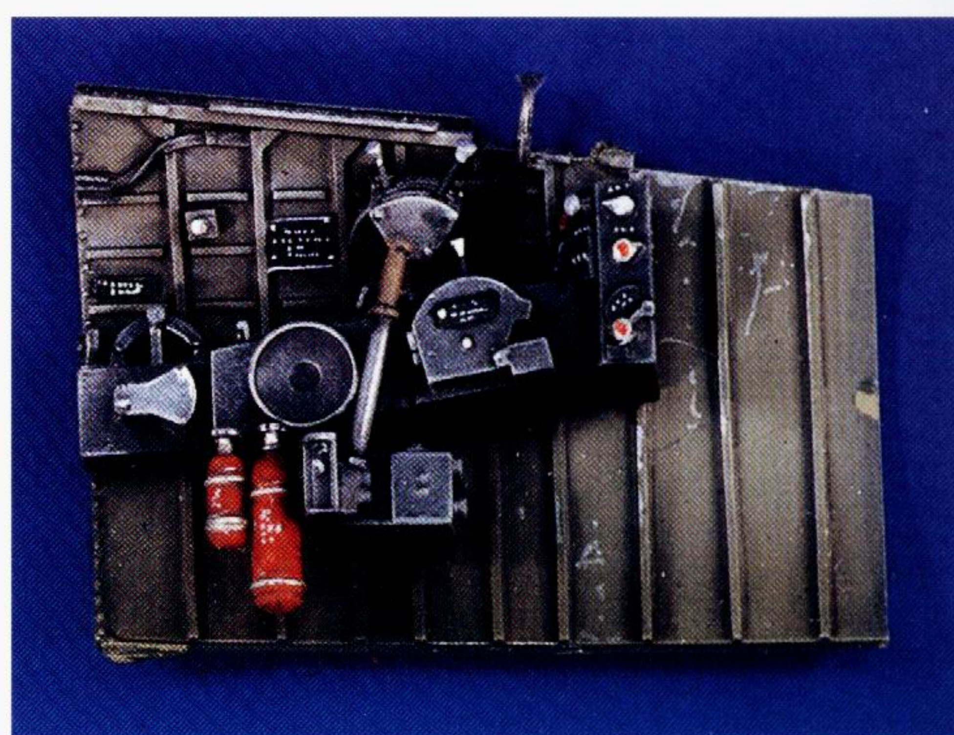
The port side-wall with associated details such as throttle, trim control, fuel tank selector, and CO2 bottles. Splashes of color, such as the Red seen here, can really enhance the appearance of the completed cockpit.
