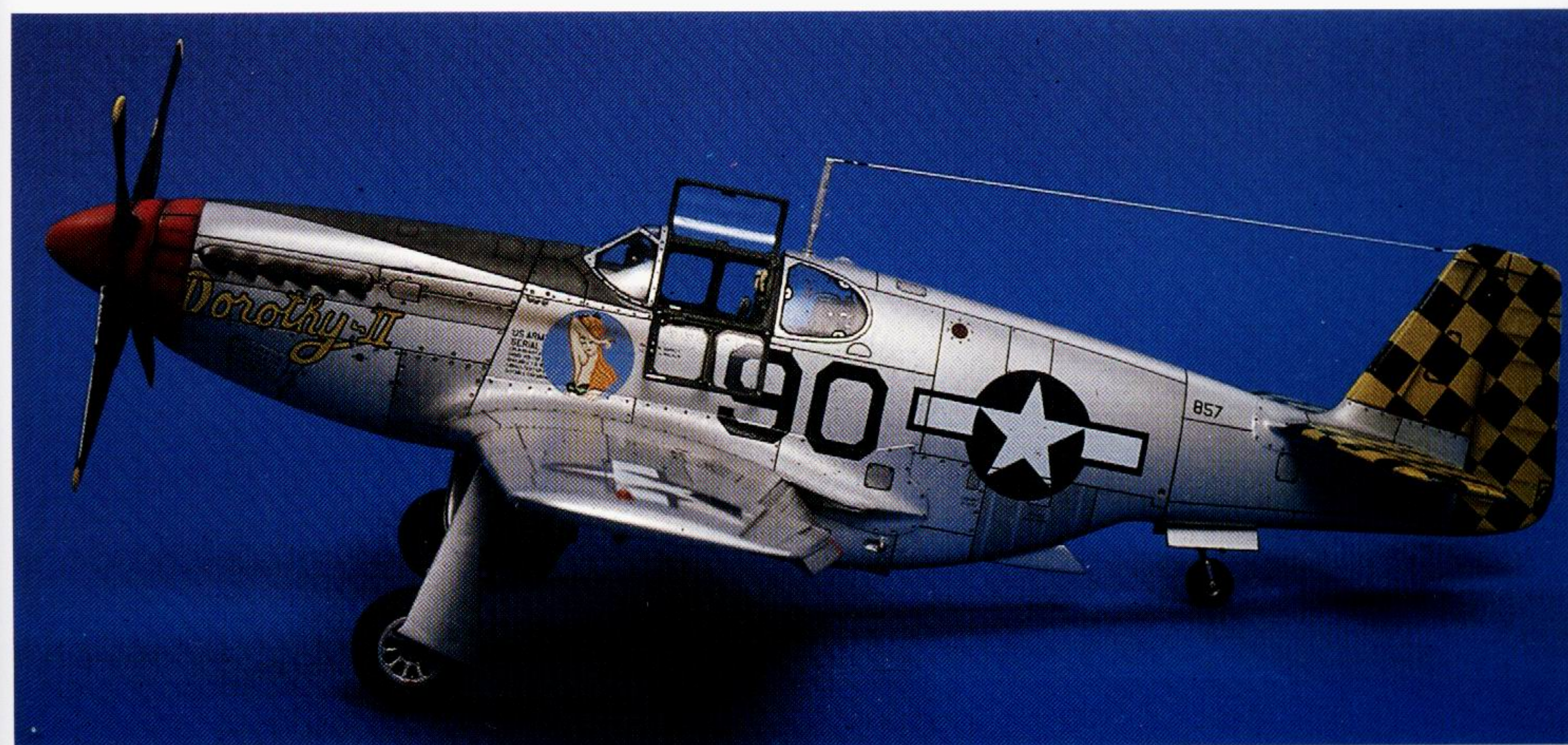
The Red nose and Olive Drab anti-glare panel were air-brushed after masking the bare metal finish with tape.
