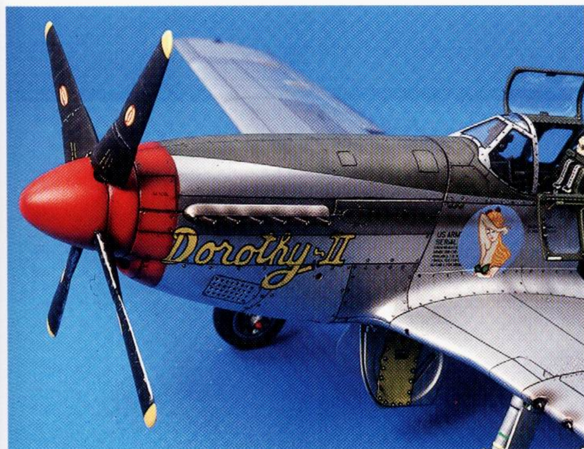
The Red nose and Olive Drab anti-glare panel were air-brushed after masking the bare metal finish with tape.
