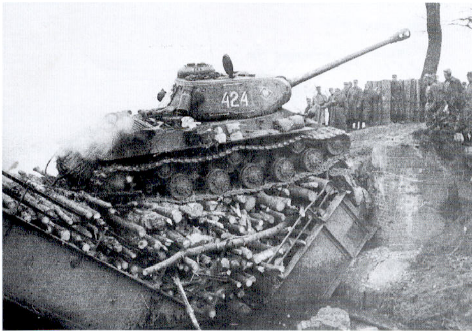
The only other army to use the IS-2 in combat in the Second World War was the Polish LWP. Here, a tank of the 4th Heavy Tank Regiment crosses a damaged bridge that has been repaired by filling it with fascines.
