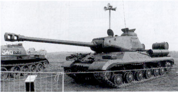
Beginning in 1954, the IS-2s were modernised as the IS-2M. This modernization included the addition of stowage boxes on the hull side, new side skirts, additional external fuel stowage and many internal improvements. This superbly restored example was handed over to the Imperial War Museum collection at Duxford Airfield in 1988, where it is currently displayed.
