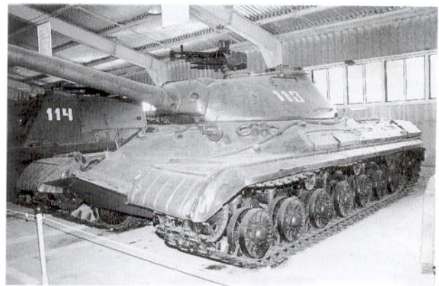
The IS-8 was basically an improved IS-3. The hull was lengthened to accommodate an improved powerplant with better cooling features. From a combat standpoint, its main
