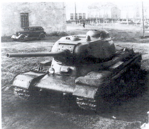
The IS-85 entered production at the end of 1943. It was a very short-lived type as it was decided to re-arm the tank with a 122mm gun. This shows the
