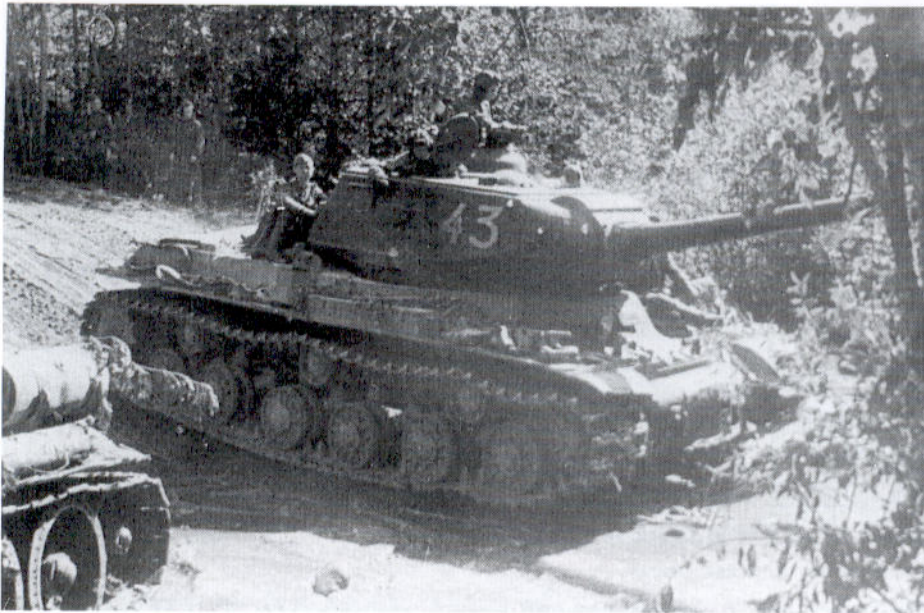
An early production IS-122 in combat in the summer of 1944. The original production batch of the IS-122 used the KV-13 hull front, the narrow gun mantlet and the early 'gum-drop' gunner's periscope on the roof.
