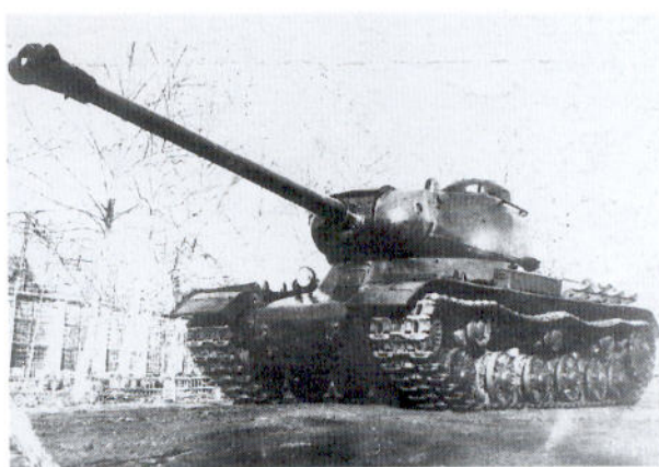
The izdeliye 240 was the prototype for the IS-2 series. It used an A-19 122mm gun with a single
