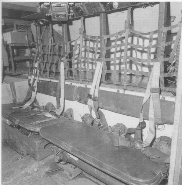
The right hand side of the troop compartment showing the harness for the troops, and the additional stowage space for personal kit behind the seats. The straps
