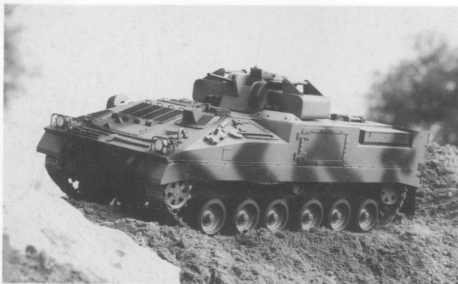
A model representation of a Warrior fitted with Trigat medium range ATGW pods. Additional missiles would be carried internally allowing the crew to reload the launchers. (GKN Defence)
