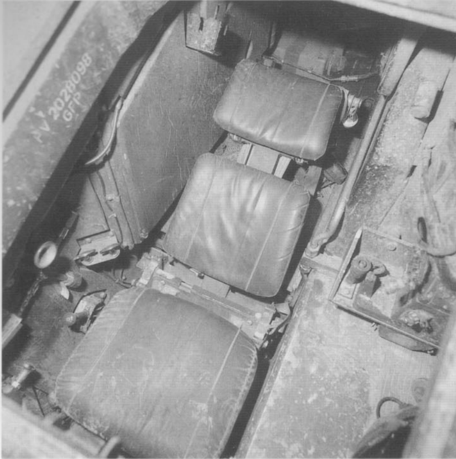
The driver's compartment looking towards the rear of the vehicle with the driver's seat reclined. This shows the cramped conditions in which the driver has to work. The two handles to the right of the driver's seat are the triggers for the Halon gas fire extinguishing system.
