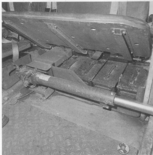
A close-up view of the storage space under the seats in the troop compartment. Here we see additional ammunition for the crews small arms (SA80 and LSW) stored under the two-
