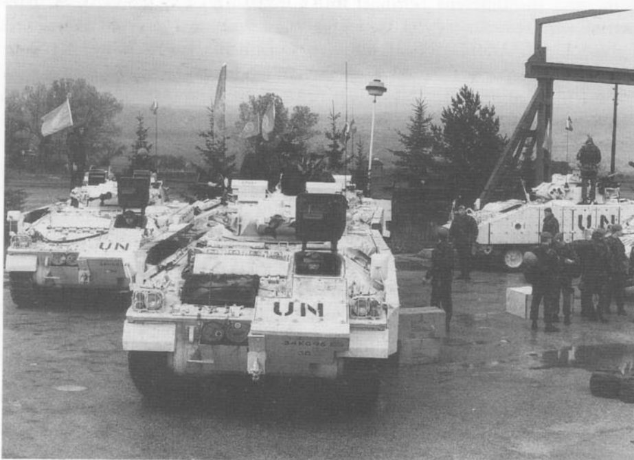
This group of Warriors from 1 Cheshire battle group are preparing to leave the unit's main base at Vitez. All the vehicles do appear to be carrying lubrication oil stowed at the front next to the additional armour plate. The vehicle in the foreground seems to have a cooker unit mounted above the oil. It appears to be the side walls of the burner for cooking in the field. This may be precaution against long delays while on escort duty. (Soldier Magazine)
