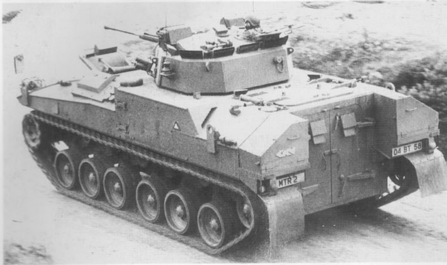
The first Warrior prototypes had twin doors in the rear of the hull as here, but these proved to be difficult to open in some tactical situations so production vehicles have a single power-operated door in the rear, although the roof hatches were retained. The turret periscopes are clearly visible, and just to the left of the commander can be seen the split mirror traversable periscope. (Terry J. Gander)
