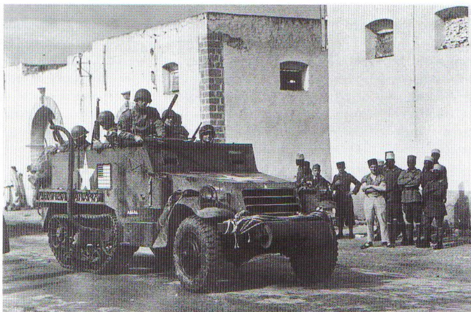
Ababa passes through Mazagan, Morocco, during the American invasion of French North Africa on 10 November 1942. This is a new production M3 with the side mine racks, a feature only authorised in August 1942. It is also fitted with the deep wading kit to allow the vehicle to be driven through the surf, evident from the exhaust extension on the hull side. (US Army Signal Corps)
