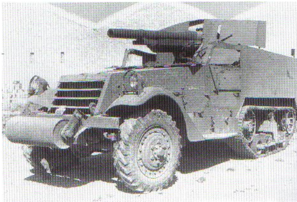
A M3 75mm Gun Motor Carriage of a tank destroyer battalion in North Africa before being issued to its crew. The production M3 75mm GMC had a more elaborate armoured shield around the gun to protect the crew from small arms fire. This is an early pro-
