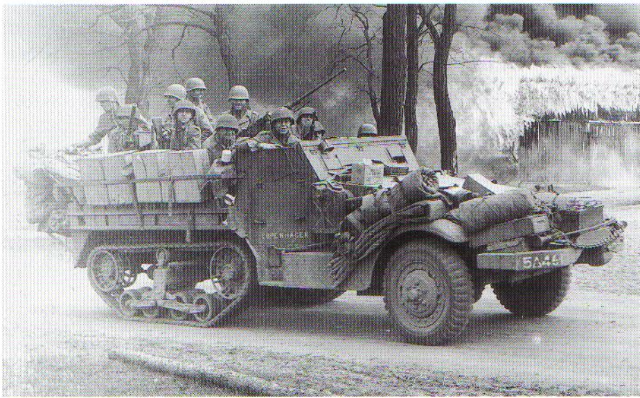
A classic view of the M3 personnel carrier in action with the 46th Armored Infantry, 5th Armored Division near Wittenmoor, Germany, on 12 April 1945. Like most half-tracks in combat for any length of time, it has become encumbered with the crew's equipment. The hull rear is fitted with a luggage rack which was first authorised in September 1943. This particular vehicle is fitted with the winch on front, and a .50cal. machine gun, usually the sign of a platoon leader's vehicle. (US Army Signal Corps)
