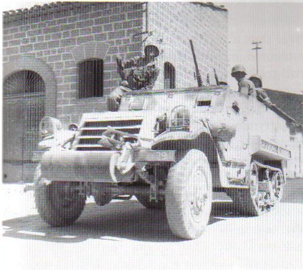
Cochran of the 82nd Reconnaissance, 2nd Armored Division moving through Rebera, Sicily, on 25 July 1943. This M3 has the side mine racks fitted; field kits for fitting them to older vehicles were autho-
