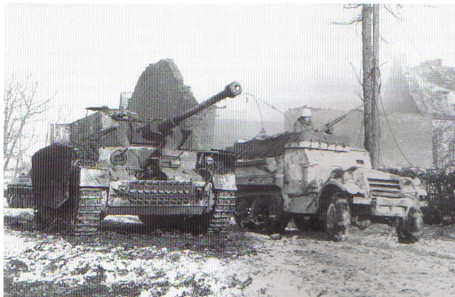
M3A1 carrier of the 6th Armored Division passes by a knocked out German PzKpfw IV in Foy, near Bastogne, in January 1945 during the Battle of the Bulge. This is another rebuilt M3, evident from the use of the old automotive-style headlights. It lacks the usual front bumper, but has been retrofitted with both the M49 ring mount characteristic of the M3A1, and the side mine racks. The front tyres and rubber tracks have been fitted with the usual winter snow chains for better traction. (US Army Signal Corps)
