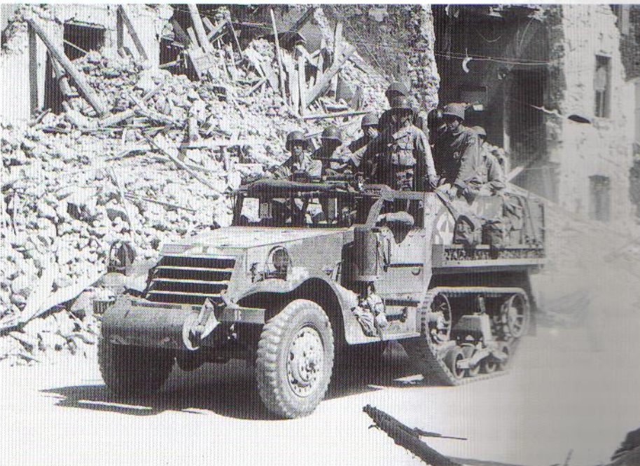
M3 personnel carrier of the 1st 'Big Red One' Infantry Division on Sicily in July 1943. This is an intermediate production type with the original style headlights, and the later external mine racks. (US Army Signal Corps)
