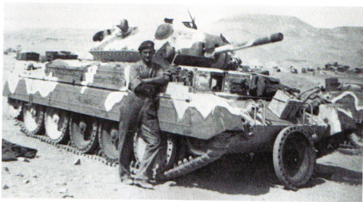
A close support Crusader, mounting the 3-in. howitzer, shown in a typical disruptive camouflage scheme. The tank alongside seems to sport another pattern altogether. These
