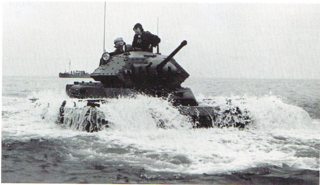
AT/1* thrashes its way through the water off Barry Island. The driver's hatch is almost obliterated by spray so he relied a lot on the turret crew for guidance.
